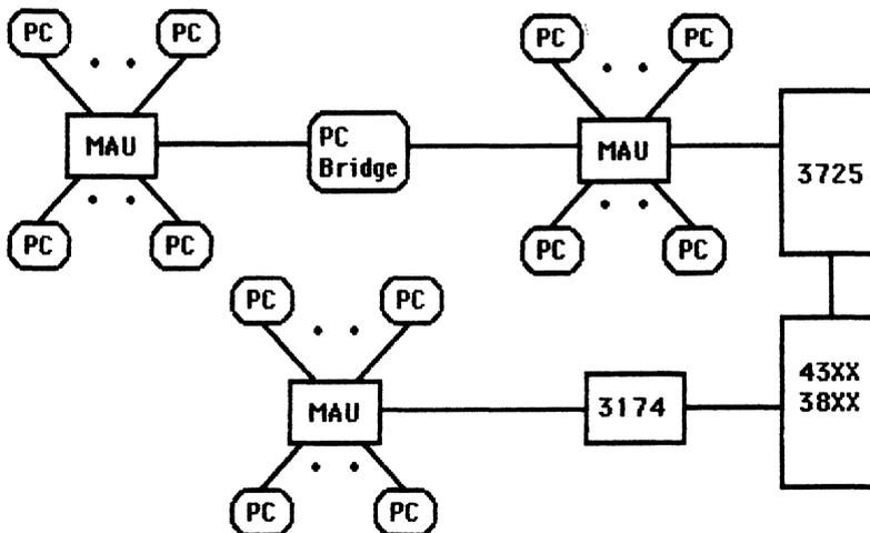
Ring support. Two of the three controllers were designed as remote devices, with an RS-232 connection to the 3725 communications controller. The third controller is designed to be channel attached to an IBM mainframe as illustrated in the lower portion of Figure 15.11 and provides a gateway to the mainframe for a "local" Token Ring local area network.
