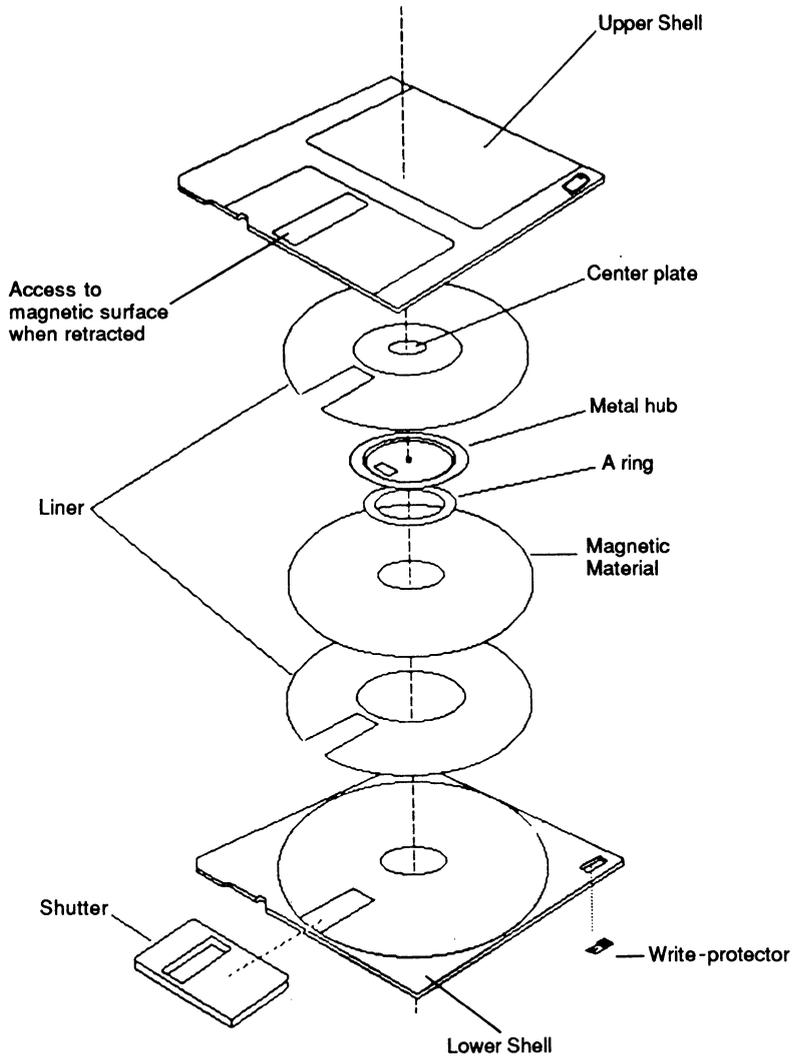
diskette to store 720K bytes of data, or you can use high-capacity diskettes to double the data-storage capacity. If you use 3½-inch high-capacity diskettes, you can format the diskette to store 18 sectors per track. The storage capacity of this diskette then becomes 2 sides times 80 tracks per side times 18 sectors per side times 512 bytes per sector, yielding 1,474,560 bytes (1.44M bytes) of information.
