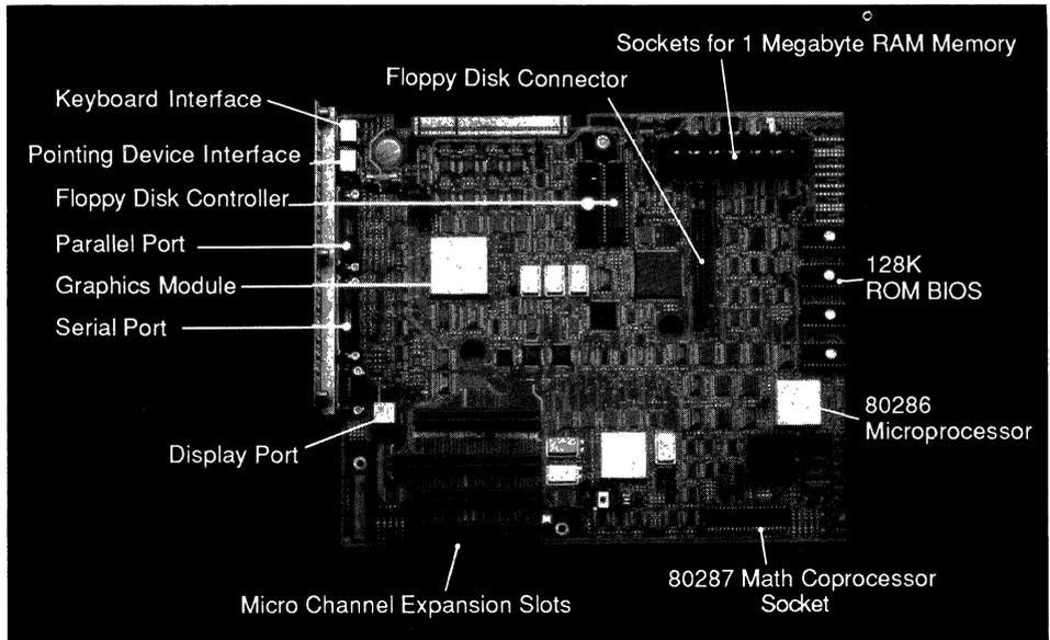
contains one of three types of microprocessors manufactured by the Intel Corporation. Models 25 and 30 use the Intel 8086; Models 30 286, 50, and 60 use the Intel 80286; and Models 55, 70, P70, and 80 use the Intel 80386 microprocessor.
