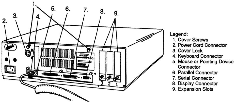
Check that the cover lock is unlocked. If it isn't, use the tubular key that came with your computer to switch the cover lock to the unlocked position, facing downward. Next, loosen the two cover screws located at the rear of the system unit using a flat blade screwdriver or coin. Then you can remove the cover to the system unit by sliding it forward approximately two inches and lifting it.
