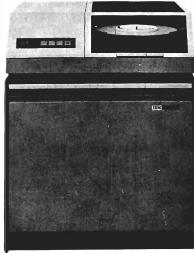
Figure 1. 2311 Disk Storage Drive
