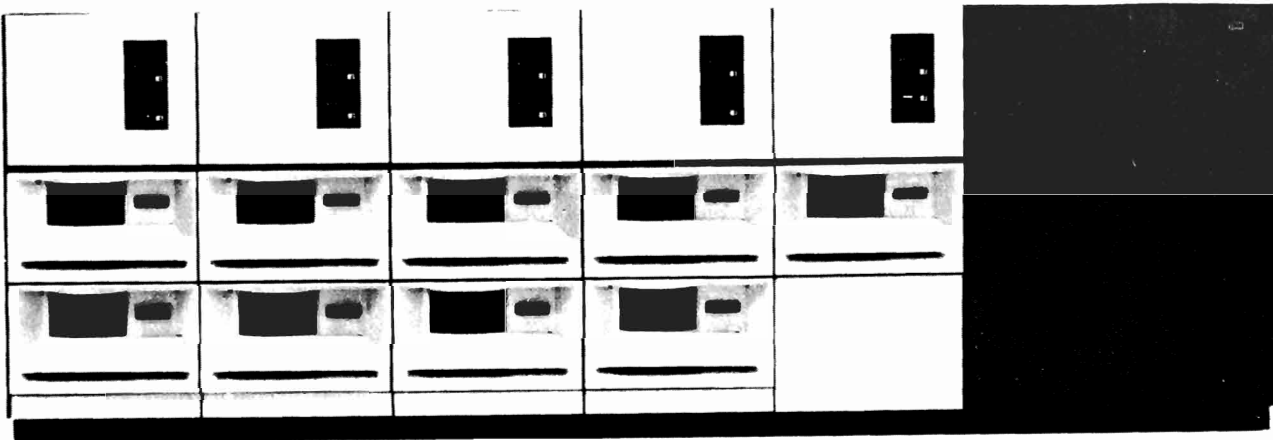
Figure 2. 2314 Direct Access Storage Facility
