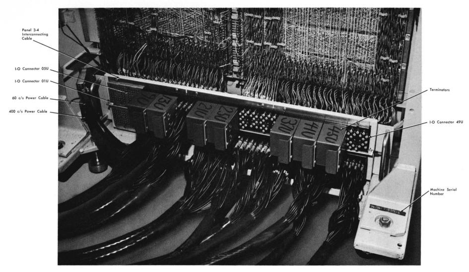
Figure 6. I-O Connectors
