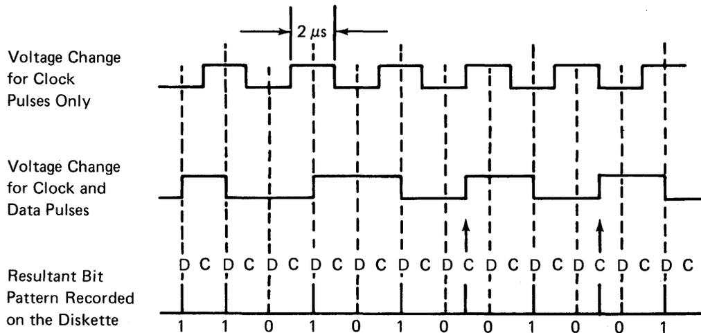
The C and D above the line show the clock and data bit times.
