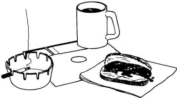
Do not place diskettes near materials that might be magnetized. Data can be lost from a diskette exposed to a magnetic field.
