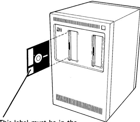
This label must be in the lower corner as the diskette is inserted in the diskette drive. The diskette drive cover must be closed and latched after the diskette is inserted.
