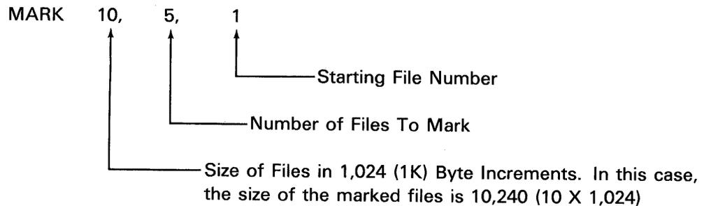
Once the MARK command is successfully completed by the 5110, the tape is formatted as follows:
