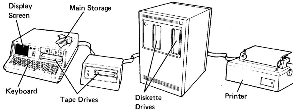
**Figure 2. 5110 Model 1 Computing System Data Processing Elements**
