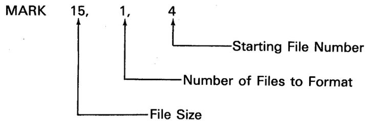
is successfully completed, the tape is formatted as follows:
