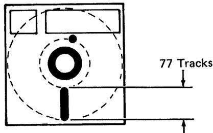
The diskette drive for two-sided diskettes has a read/write head on each side. Each track on side 0 of a two-sided diskette has an associated track on side 1.
