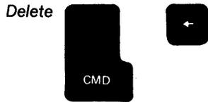
When the CMD key is held down and the backspace key is pressed once, the character at the cursor position (flashing character) is deleted and all characters to the right are moved over one position to the left to close up the space. The cursor is not moved. For example:
