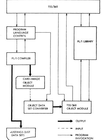
Figure 3. Relationship of a TSS/360 PL/I Object Module with the System Programs
