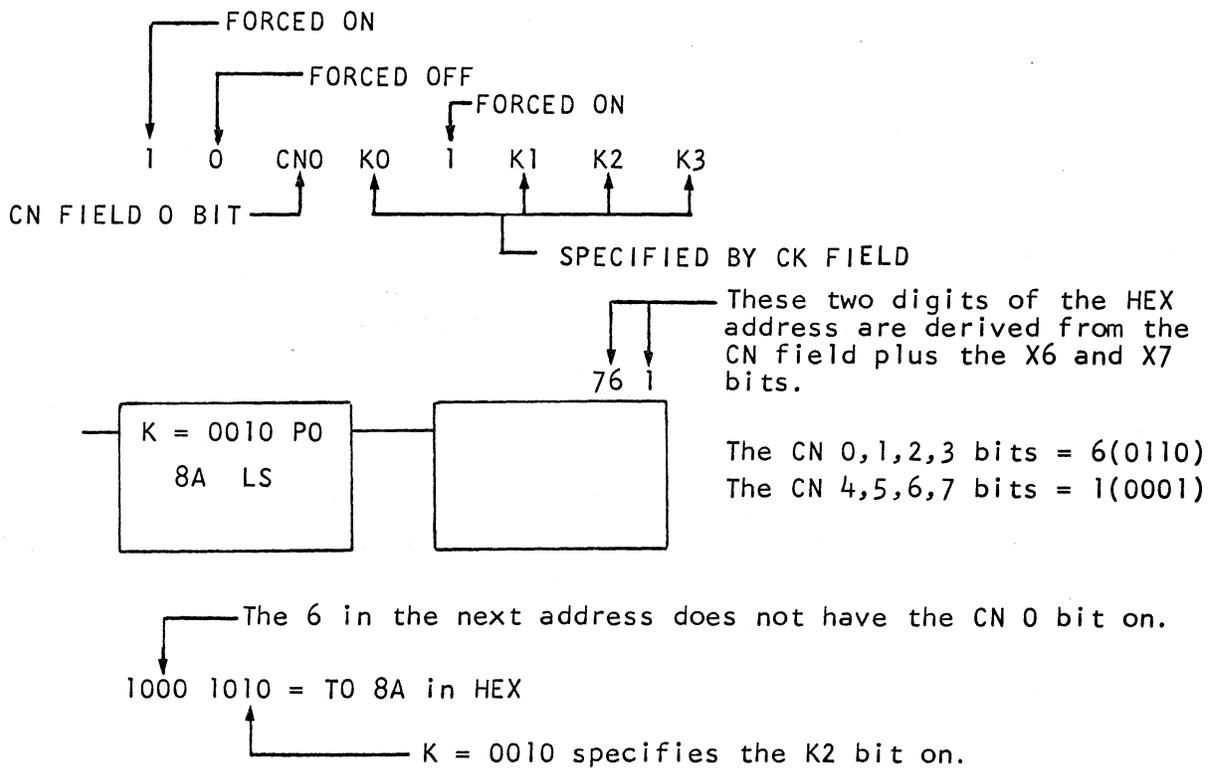
CN field 0 bit = 0 indicates the K addressable bytes 0 through 15 that will be addressed.
