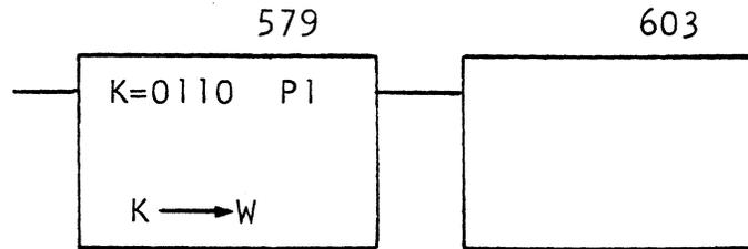
This signifies a module change (the K field value specifying that the address of the next microword is in the 600 block).
