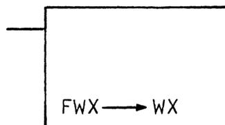
This instruction sets the FWX register (backup ROSAR) back into the WX register (100) and interrogates the X6 and X7 buffer latches to determine what the branching status was at the time of the trap, thus the instruction establishes the link address (100), which is the first word executed after the trap has been satisfied.
