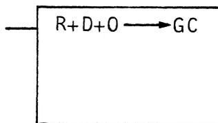
The 0 in this statement forces the carry-input line to 0, and the C indicates that if a carry out of the high-order position results, the S3 bit will be set to a 1.
