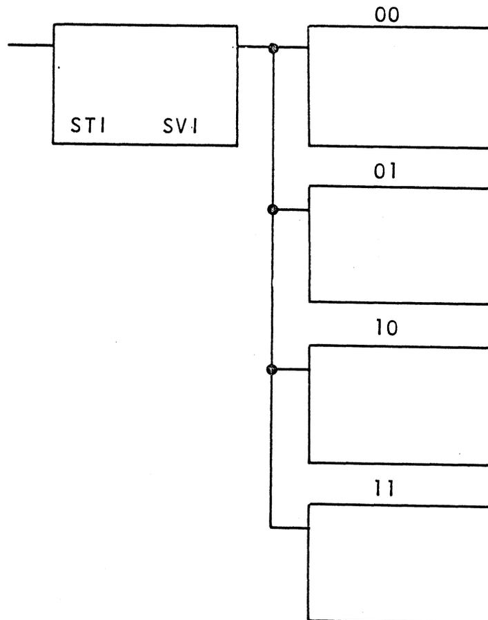
This signifies conditional branching. If the Status In Line (STI) is up and the Service In Line (SVI) is down, this condition forces a branch to the microword identified by 10.
