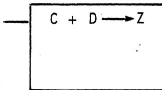
This signifies that the ALU output goes onto the Z buss but not into any register.
