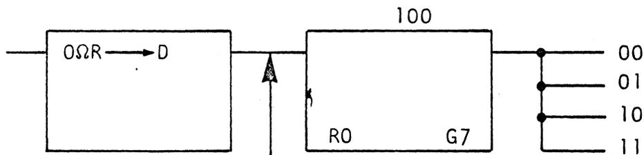
If a trap occurred at this point in a microprogram, the WX register which contains the address of the next microword (100) is set into the FWX register (backup ROSAR). The CH and CL fields are interrogated and set into the X6 and X7 buffer latches.
