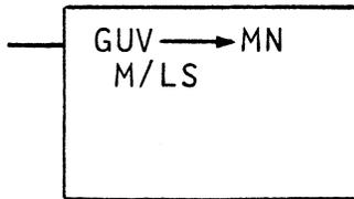
Signifies that main storage will be addressed if the G register 0 and/or 1 bits are on (1), and that local storage (CPU Bump) will be addressed if the G register 0 and 1 bits are off (0).
