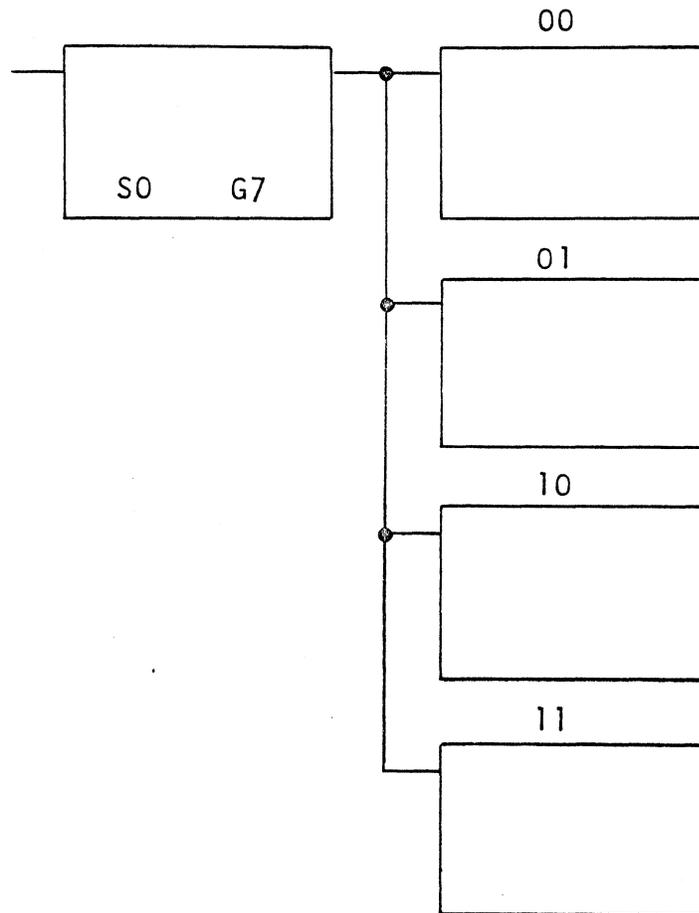
This signifies branching on latches in registers. If the S register 0 bit and the G register 7 bit are on, this condition forces a branch to the microword identified by 11.
