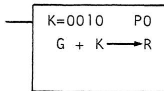
This signifies that a constant of 2 (0010) will be generated on the K buss, and is the source input data for the B register.
