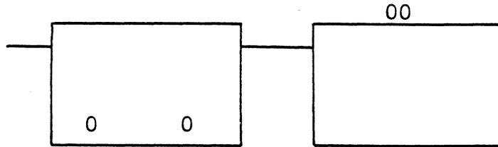
Signifies forced branching. If CH and CL are zeros, it forces a branch to the next microword identified by 00. If CH and CL are 01, it forces a branch to the next microword identified by 01.
