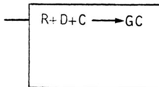
The first C in this statement forces the value of the carry latch (S3) onto the carry-input line. The second C indicates that if a carry out of the high order position results, the S3 bit will be set to a 1.
