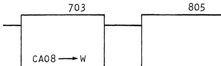
This signifies a module change. This condition indicates that the address of the next microword is in the 800 block.
