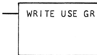
Signifies that the selector channel data register GR is the destination for data instead of the normal destination R register.
