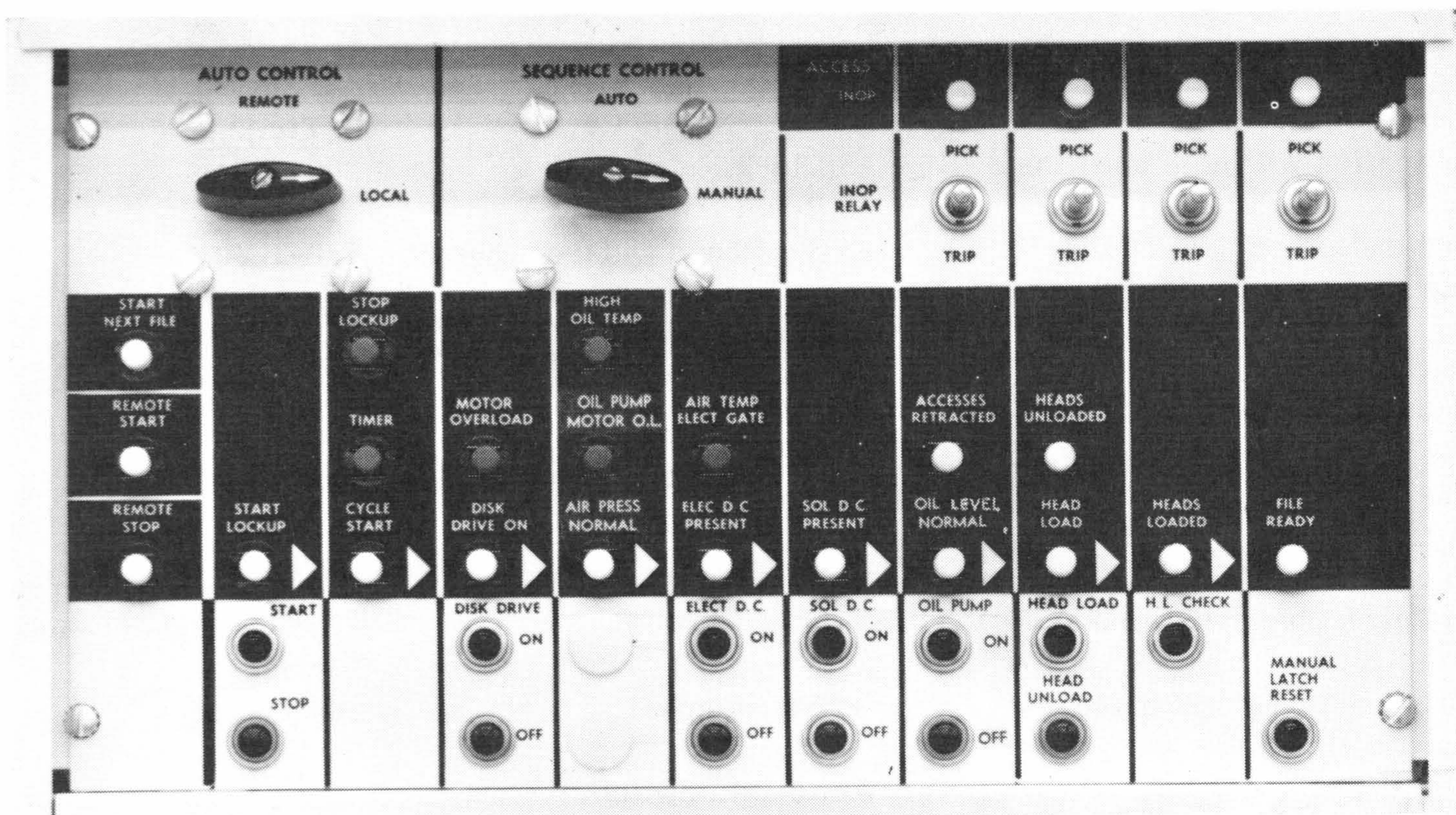
Figure 3-5. Power Sequence Control Panel
