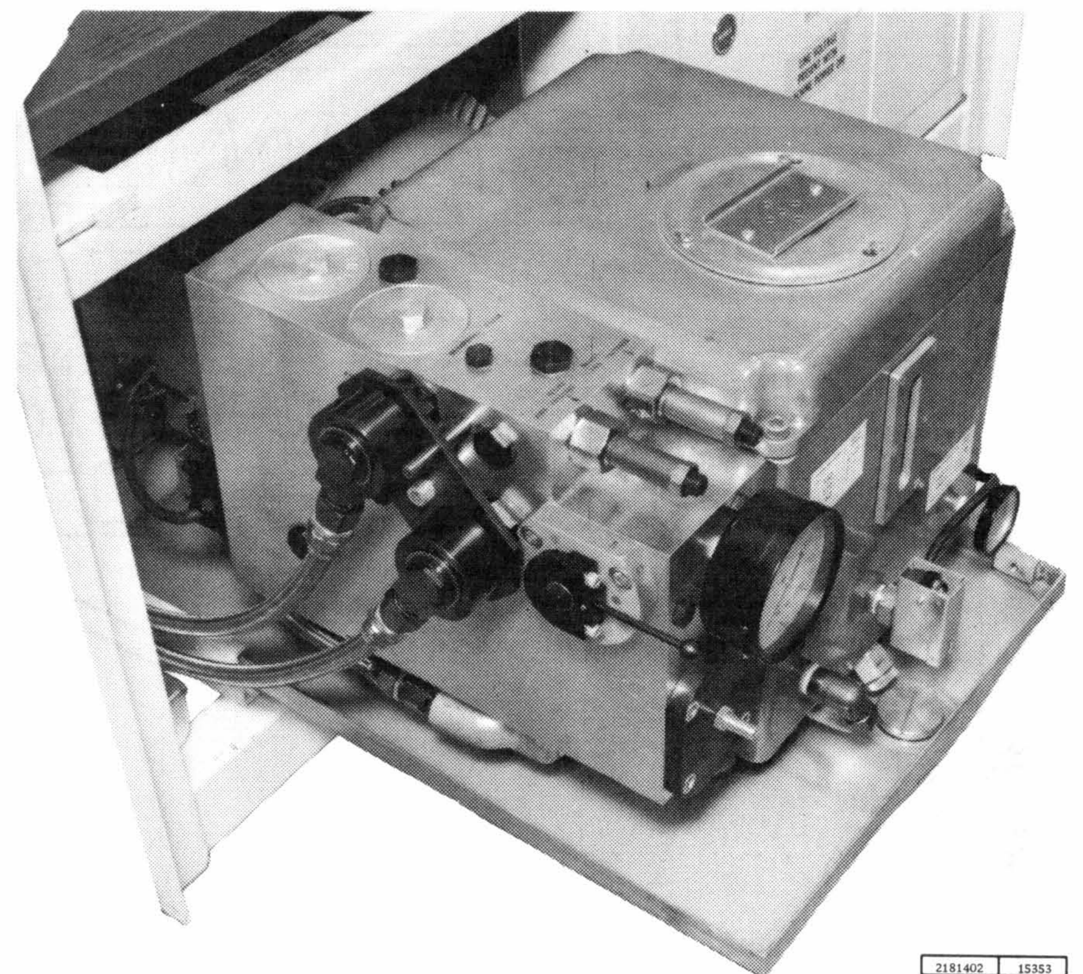
Figure 2-45. Hydraulic Power Supply in Servicing Position
