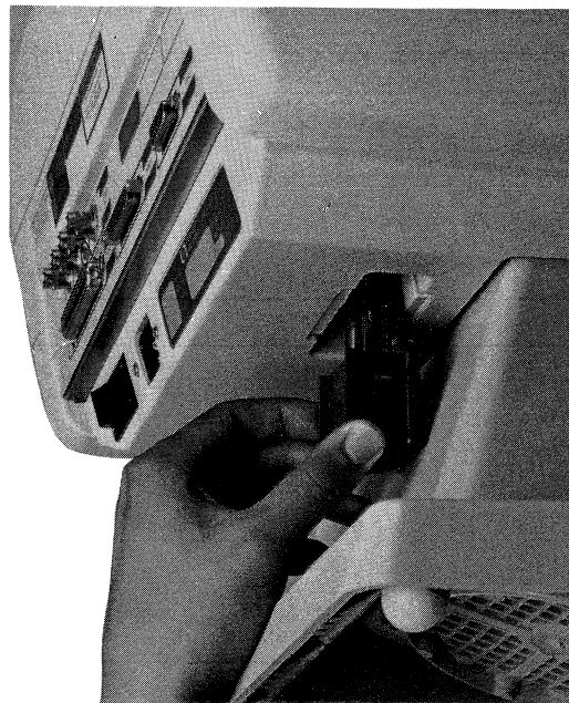
Figure 10-1. Removing the Batteries
