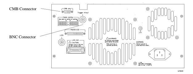
The location of the CMB and BNC connectors on the HP 64700 rear panel is shown in the following figure.
