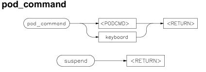
Allows you to control the emulator through the direct HP 64700 Terminal Interface.
