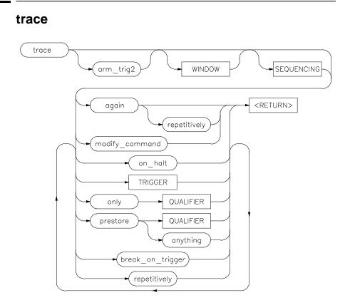
This command allows you to trace program execution using the emulation analyzer.
