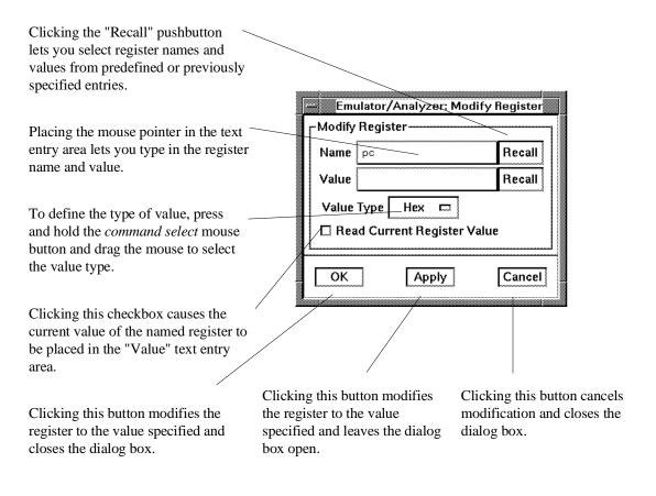
• Using the command line, enter the **modify register** <**register**> **to** <**value**> command.
