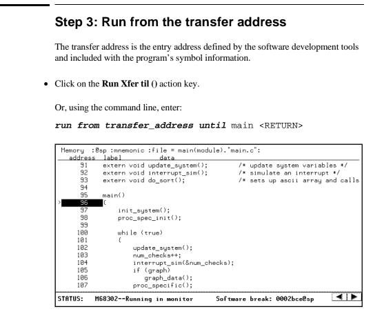
Notice the message "Software break: <address>" is displayed on the status line and that the emulator is "Running in monitor". When you run until an address, a breakpoint is set at the address before the program is run.
