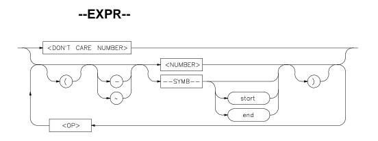
An expression is a combination of numeric values, symbols, operators, and parentheses used to specify address, data, status, executed address, or any other value used in the emulation commands.
