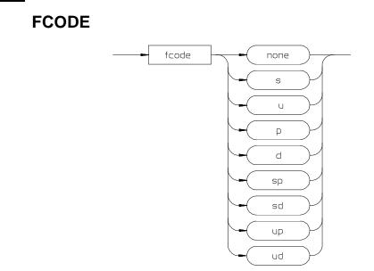
The function code is used to define the address space being referenced. Select the appropriate function code from those listed below.
