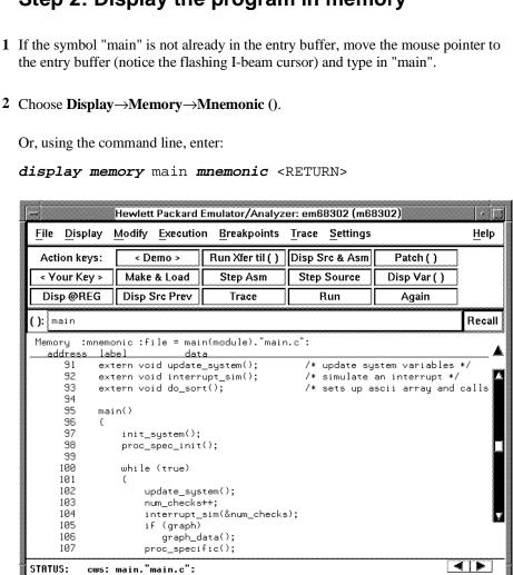
The default display mode settings cause source lines and symbols to appear in displays where appropriate. Notice you can use symbols when specifying expressions. The global symbol "main" is used in the command above to specify the starting address of the memory to be displayed.
