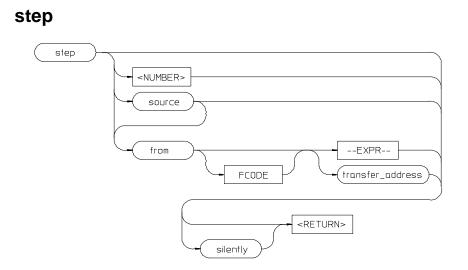
The **step** command allows sequential analysis of program instructions by causing the emulation processor to execute a specified number of assembly instructions or source lines.
