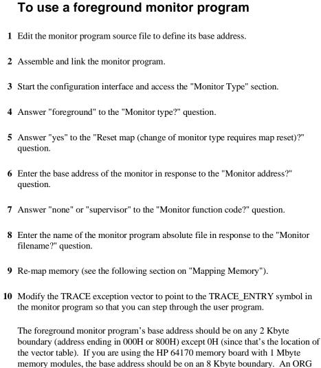
statement in the foreground monitor source file defines the base address. Also, the base address is specified when configuring the emulator to use a foreground monitor program.
