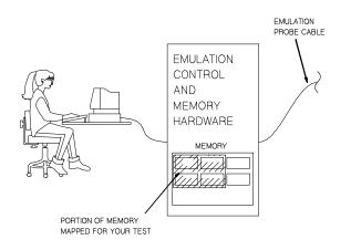
Figure 2-1. Out-Of-Circuit Emulation
