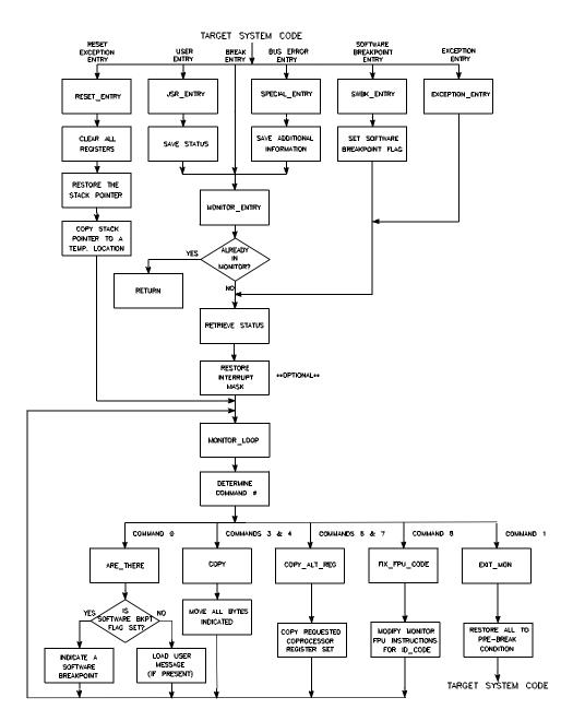
Figure 3-2. Emulation Monitor, Typical Block Diagram
