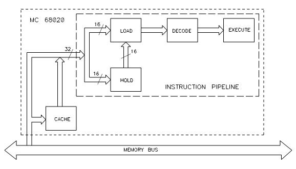
Figure 11-1. Pipeline Diagram Of The 68020
