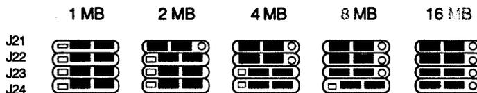
**FIGURE 7-3. Slave window size jumper settings J21–J24**
