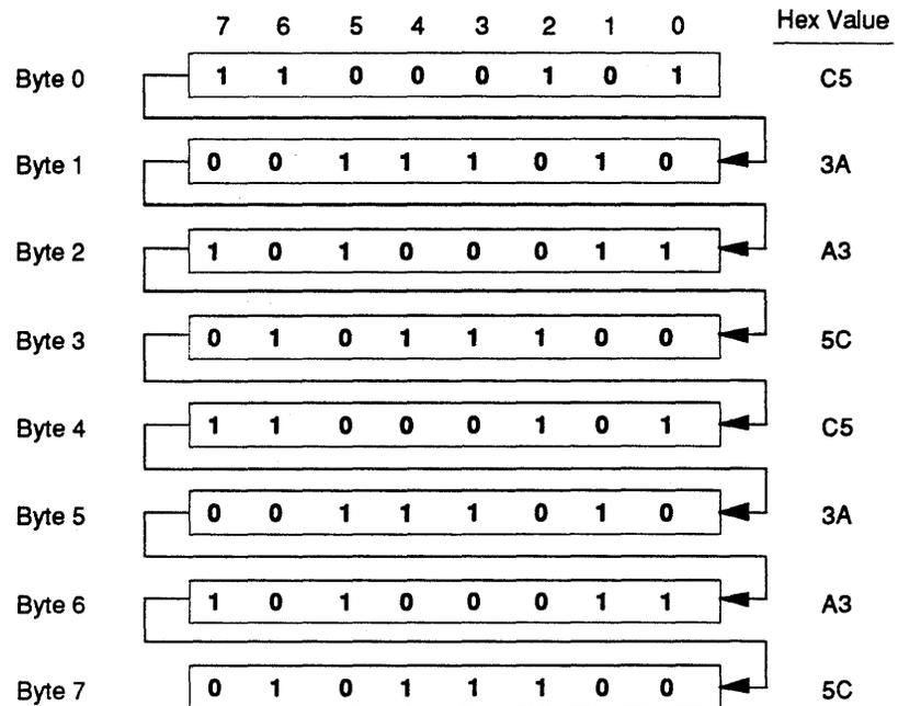
**FIGURE 13-2. RTC comparison register definition**
