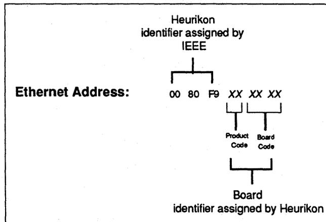
**FIGURE 12-1. Ethernet address format**
