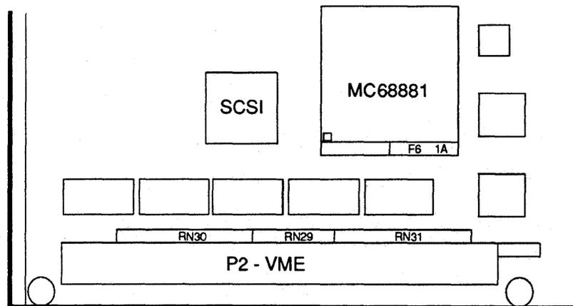
**FIGURE 11-2. Location of SCSI terminating resistor networks and fuse F6**
