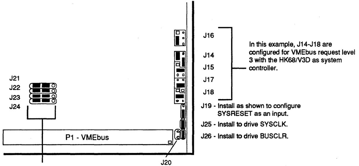
In this example, J21-J24 are configured for 16-megabyte slave window size.
