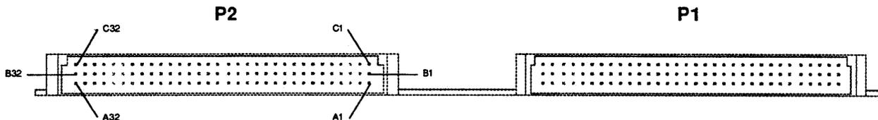
**FIGURE 7-7. VMEbus connectors, P1 and P2**
