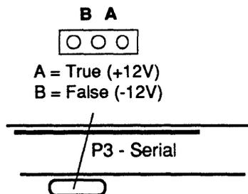
Be sure the ROM size jumpers J5–J8 are configured to match the size of ROM on the board (settings are described in the section "On-card Memory Configuration," section 5). The serial cable should connect the terminal with port B on the HK68/V3D. Terminal settings should be 9600 baud, 8 data bits, 1 stop bit, no parity.
