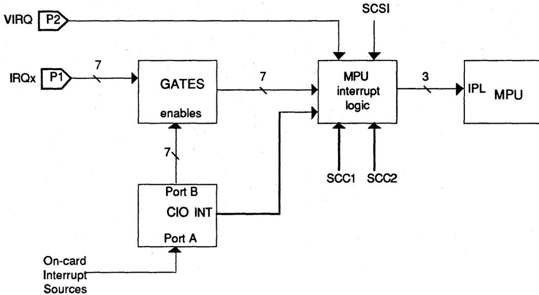
**FIGURE 7-6. Interrupt signal routing**
