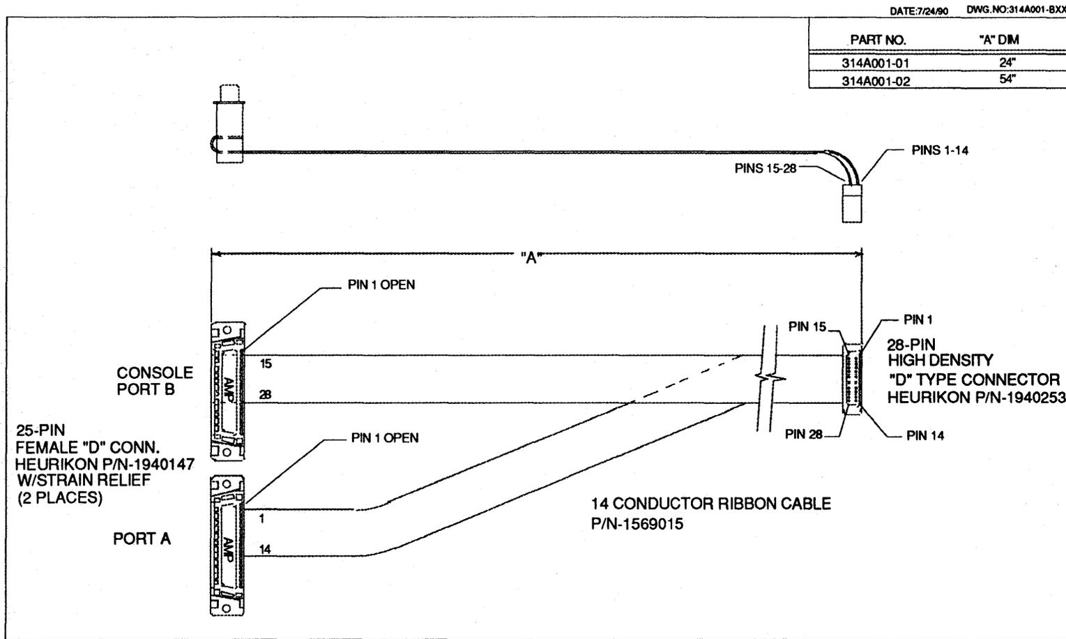
**FIGURE 10-2. Serial I/O cable**
