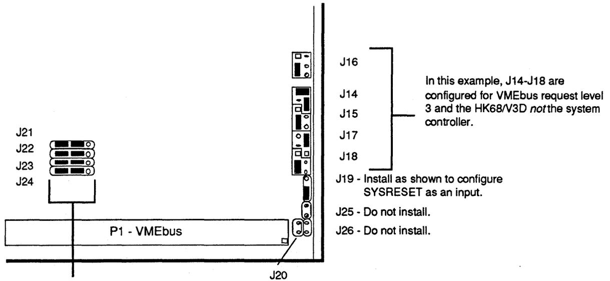
In this example, J21-J24 are configured for 16-megabyte slave window size.
