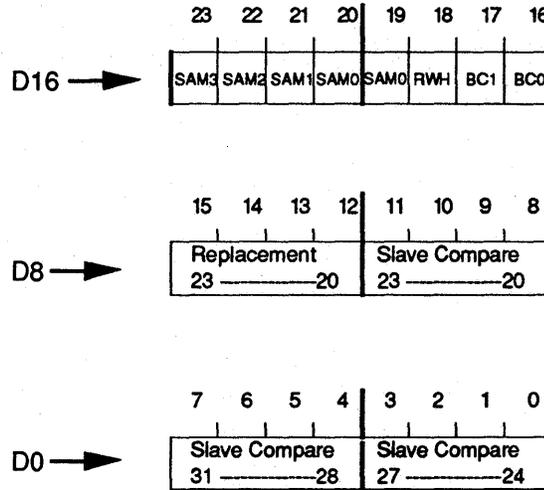
**FIGURE 7-4. Bus control latch**
