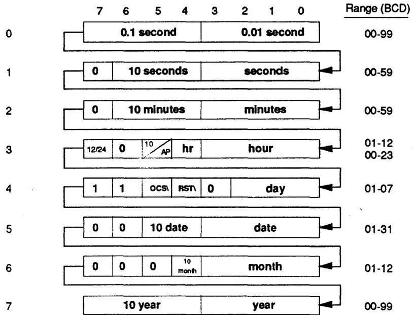
**FIGURE 13-3. RTC register definition**
