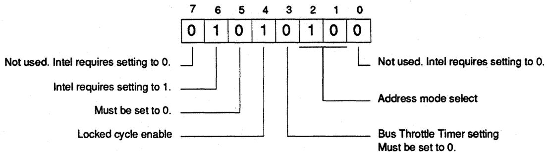
**FIGURE 12-2. Required settings of the System Configuration Pointer SYSBUS byte**
