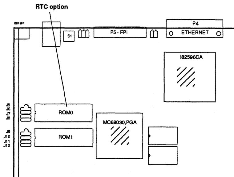
**FIGURE 13-1. Real-time clock socket**
