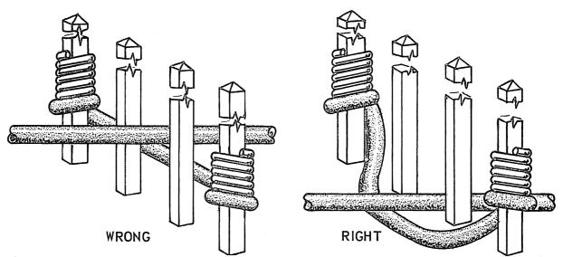
FIG. 17 - USE OF DRESSING FINGERS TO PROVIDE SLACK FOR DRESSING THE WIRE DOWN TO RELIEVE BUILD-UP
