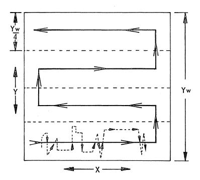
General Path of Machine Carriages Resulting from the X,Y Sequencing.
