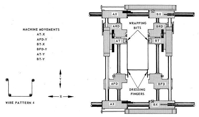
FIG. 11 - FINAL CARRIAGE POSITIONS PATTERN 4
