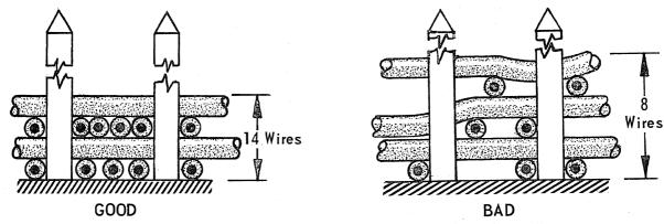
FIG. 18 - SEQUENCING TO REDUCE CHANNEL BUILD-UP
