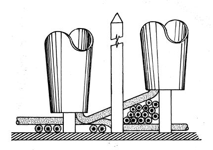
FIG. 16 - CHANNEL BUILD-UP EFFECT ON SHORT Z-1 WRAPS
