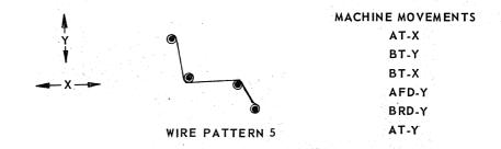
FIG. 12 - FINAL CARRIAGE POSITIONS PATTERN 5
