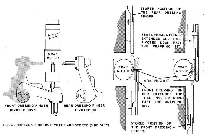
FIG. 6 - DRESSING FINGERS PIVOTED AND STORED (TOP VIEW)
