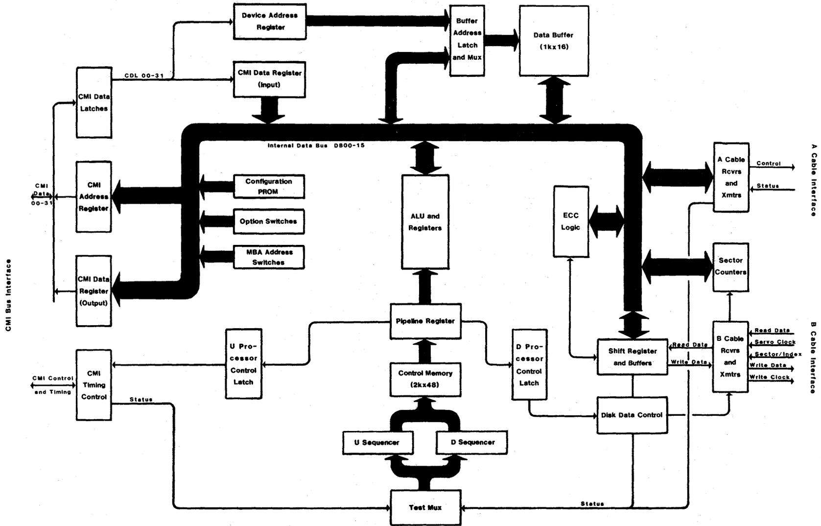
Figure 2-1 SC750 Block Diagram
