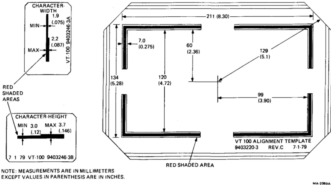
Figure 3-1 Video Alignment Template Dimensions
