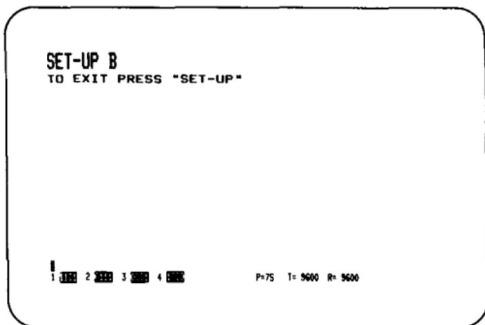
Figure 6-2 SET-UP B (VT101)
