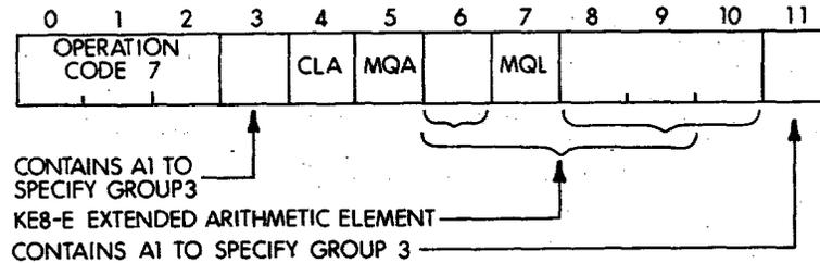
**Figure 3-4 Group 3 Operate Microinstruction Bit Assignments**
