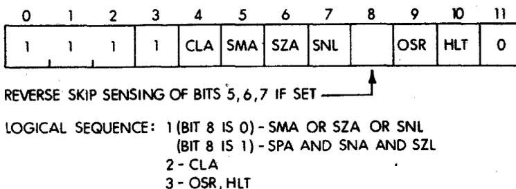
**Figure 3-3 Group 2 Operate Microinstruction Bit Assignments**
