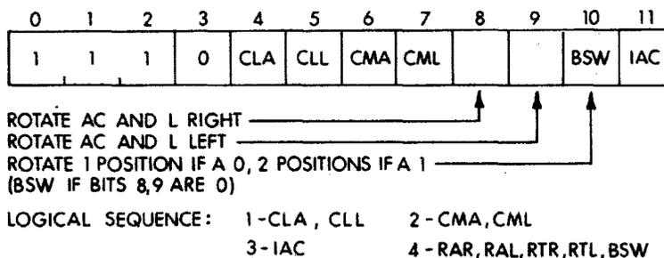
**Figure 3-2 Group 1 Operate Microinstruction Bit Assignments**
