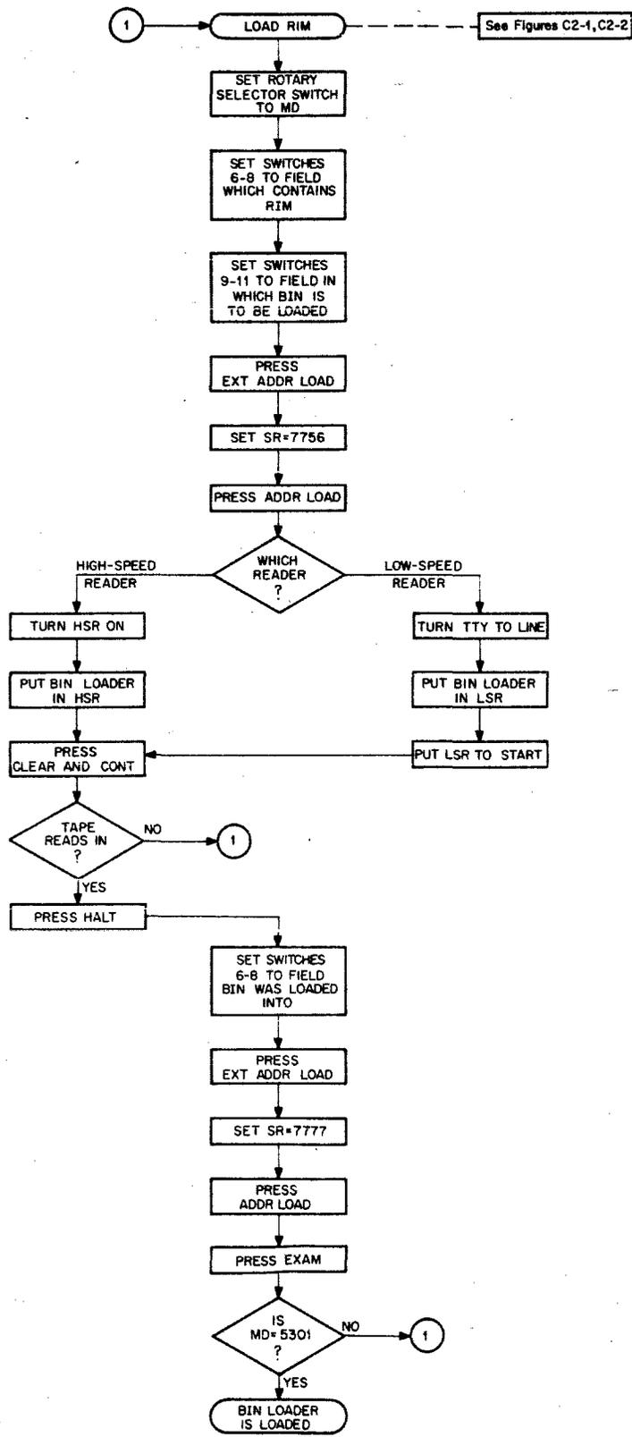
Figure B-3 Loading the BIN Loader
