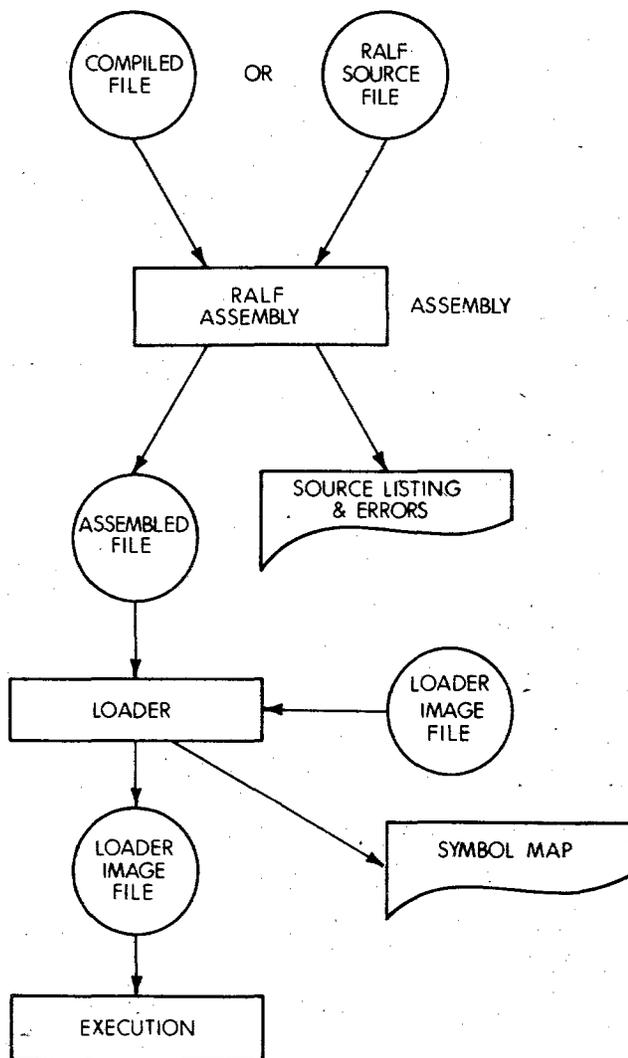
**Figure 8-3 Assembling, Loading, and Executing a RALF File**
