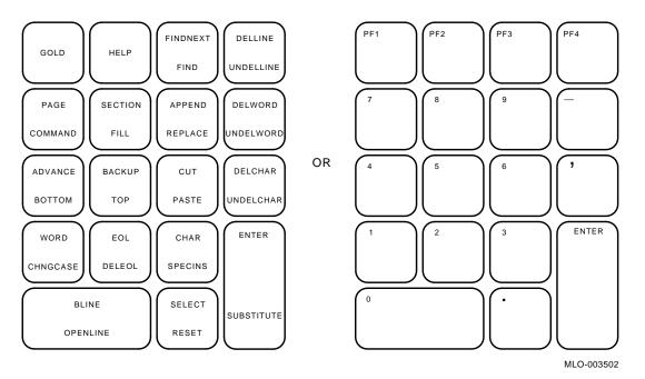
Most of the function keys specify two functions: a standard function and an alternate function.
