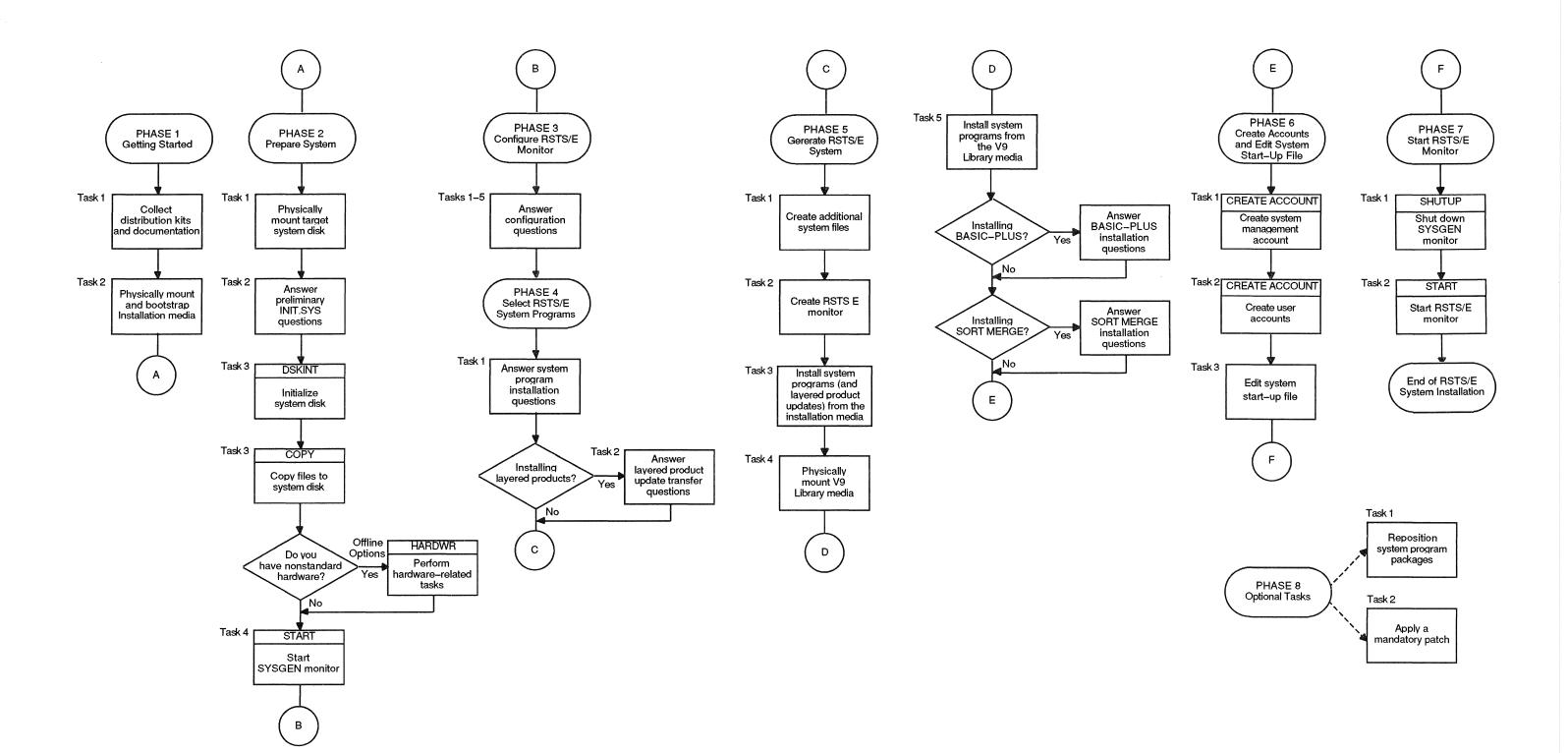
Figure 3: System Installation Flowchart
