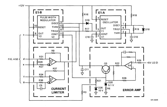
Figure 4-51 Output Control Circuit, Simplified Diagram
