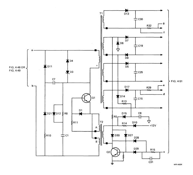
Figure 4-50 Flyback Inverter Circuit, Simplified Diagram
