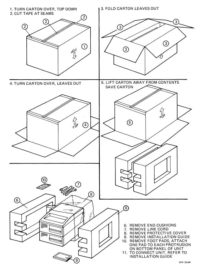
Figure 2-1 PDT-11/150 Unpacking Procedure
