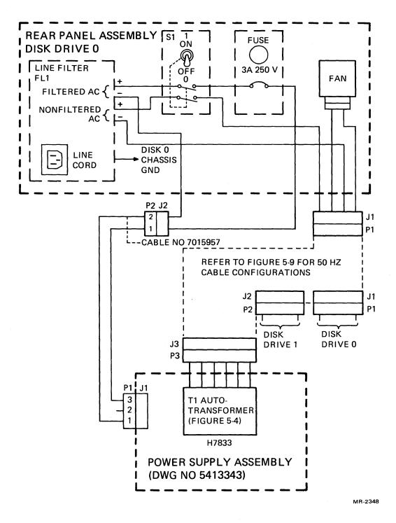
Figure 5-8 AC Power Distribution, 50 Hz Units
