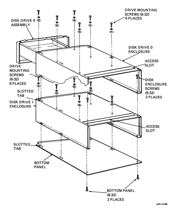
Figure 5-36 Disk Drive and Enclosure Mounting
