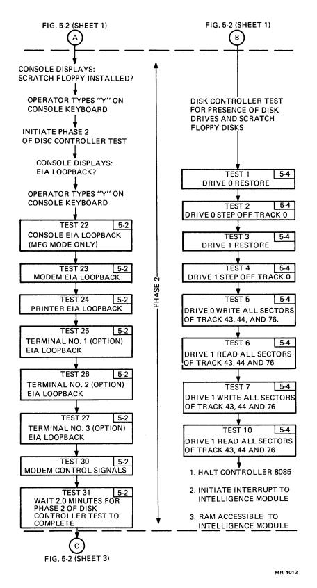
Figure 5-2 Self-Test Sequence Chart (Sheet 2 of 3)
