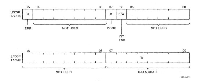
Figure 6-9 Printer Terminal Interface Register Formats
