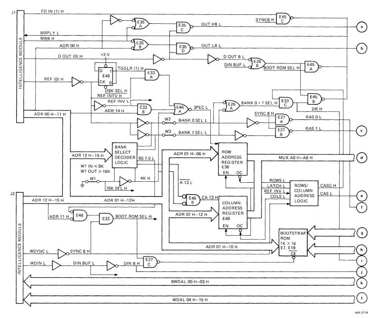
Figure 4-16 RAM Module, Simplified Function Diagram (Sheet 1 of 2)
