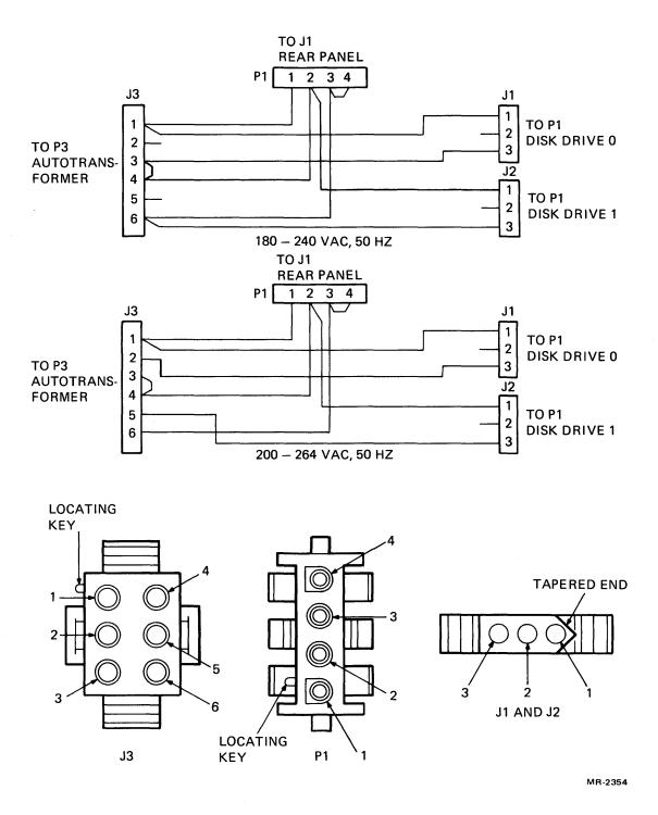
Figure 5-9 50 Hz Internal Cable Configurations (Sheet 1 of 2)
