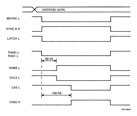
Figure 4-21 Row/Column and Address Multiplexer, Timing Diagram
