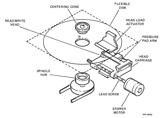
Figure 5-50 Read/Write Head Positioning Mechanism
