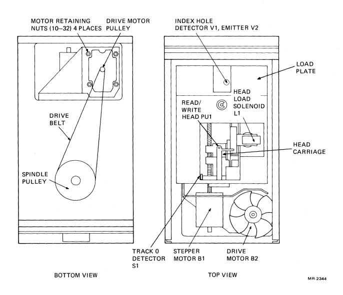
Figure 5-46 Disk Drive Assembly, Component Locations
