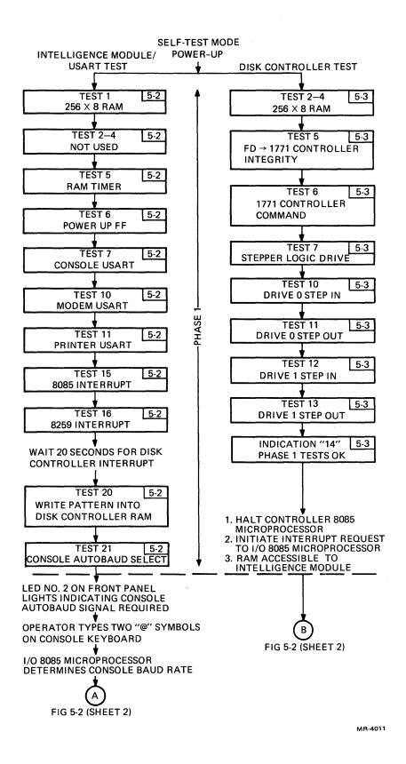
Figure 5-2 Self-Test Sequence Chart (Sheet 1 of 3)
