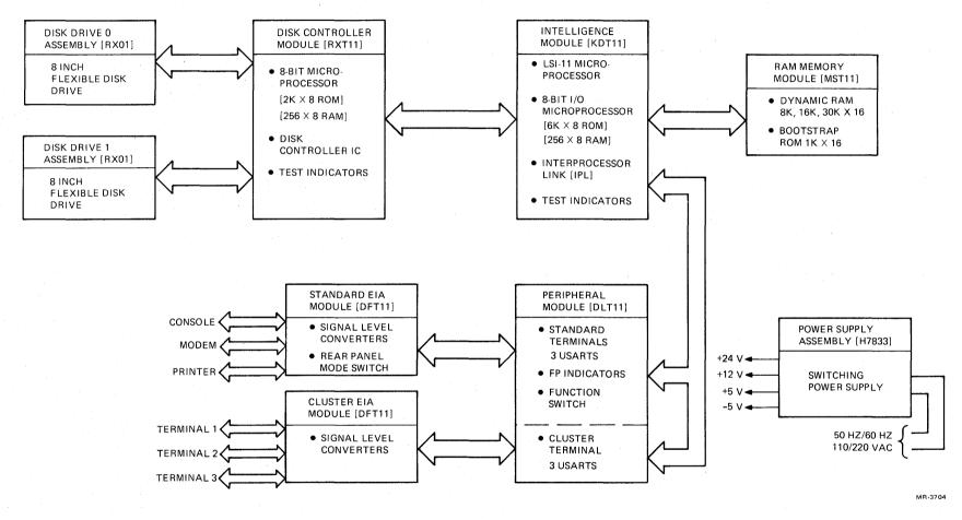
Figure 4-1 PDT-11/150, Simplified Block Diagram
