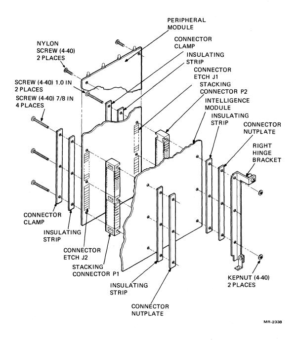
Figure 5-26 Peripheral Module, Removal and Replacement
