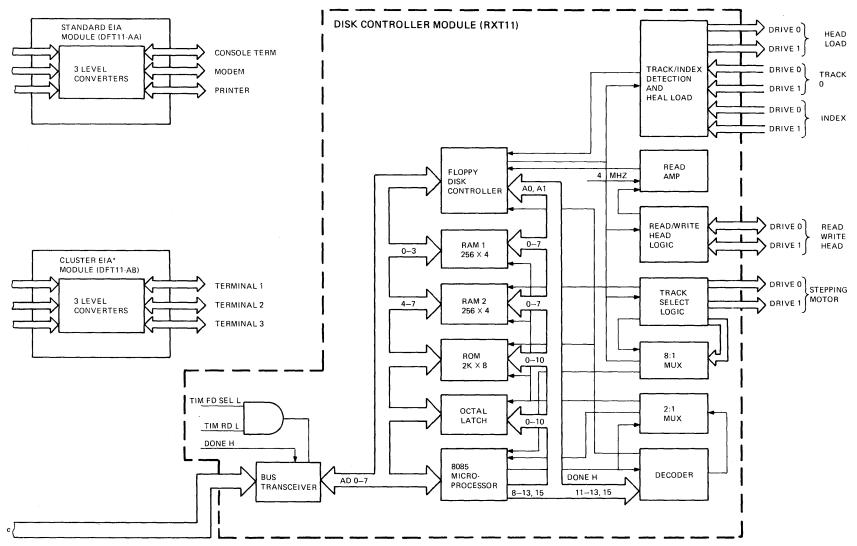
Figure 4-2 PDT-11/150 Bus Structure (Sheet 3 of 3)
