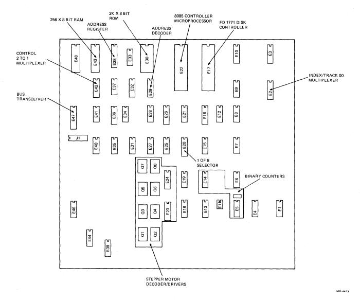
Figure 5-44 Disk Controller Module (Revision L), Functional Layout
