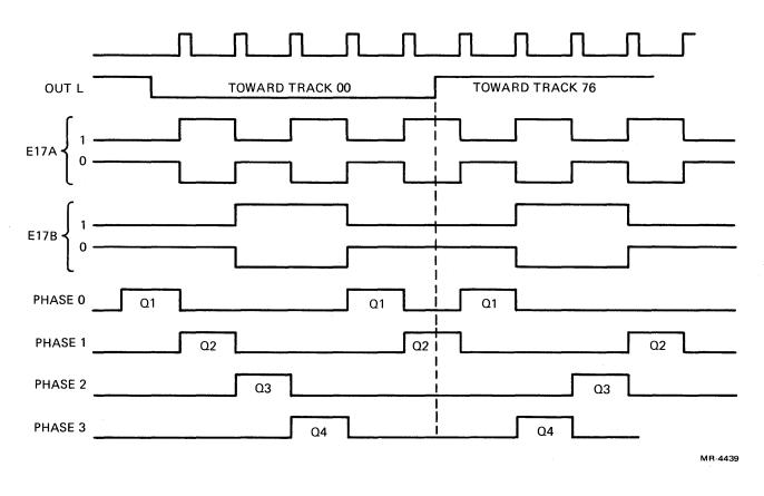
Figure 4-36 Stepper Motor Control and Drive Logic, Timing Diagram
