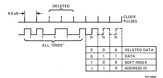
Figure 4-29 Double Frequency (FM) Address Mark Pattern
