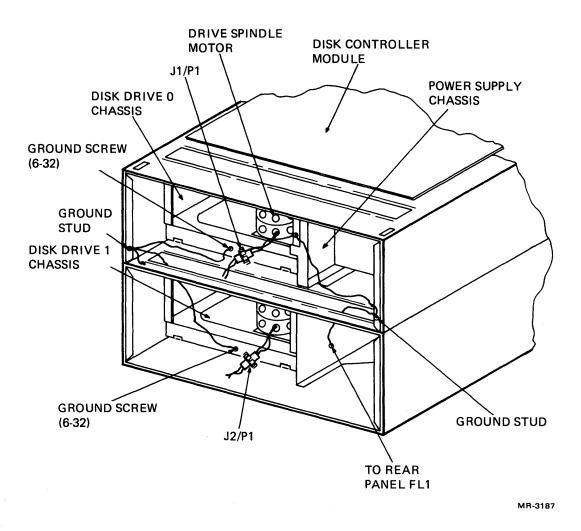
Figure 5-35 Disk Drive Ground Lead and ac Cable Connections
