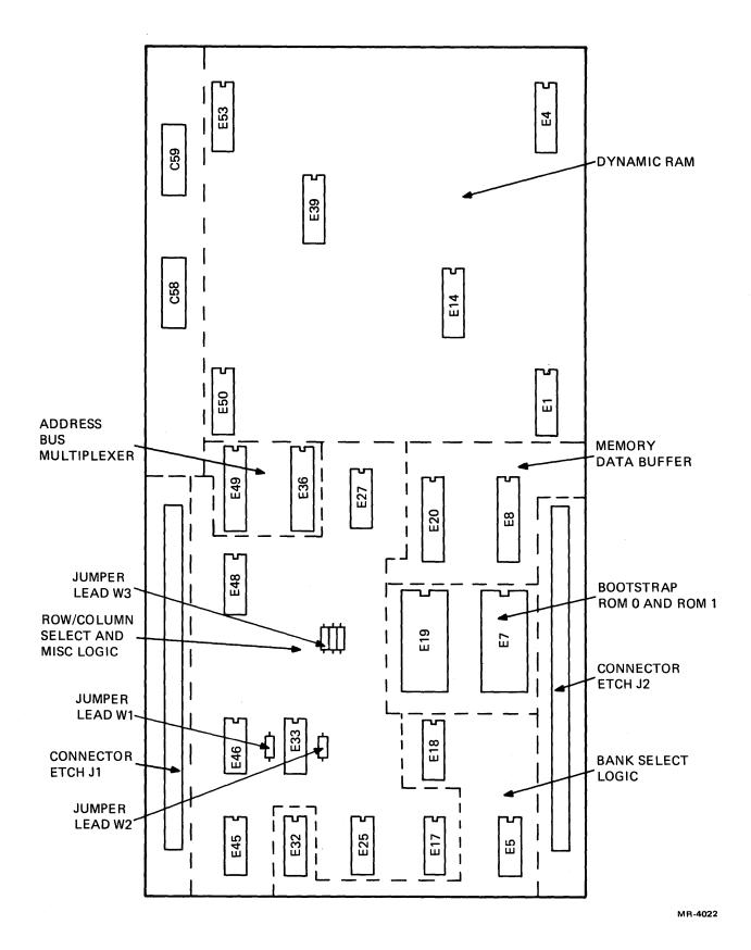
Figure 5-39 RAM Module, Functional Layout
