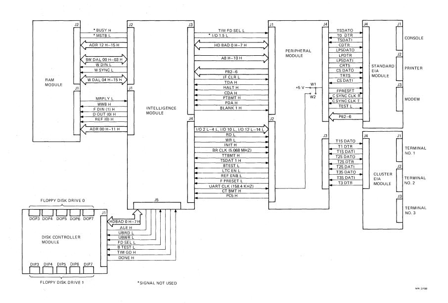
Figure 4-3 PDT-11/150 Internal Signal Distribution
