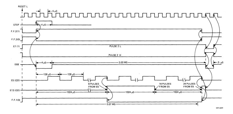
Figure 4-34 Step Generator Circuit, Timing Diagram
