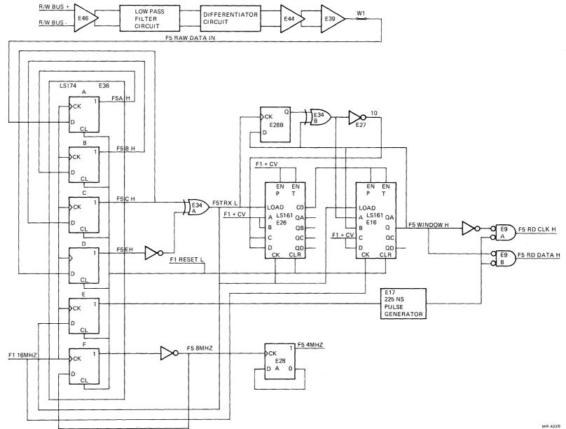
Figure 4-42 Read Amplifier and Data Separator Circuit (Revision L), Simplified Diagram
