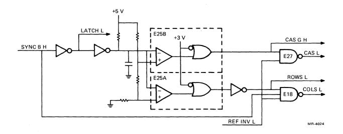
Figure 4-20 Row/Column and Address Multiplexer, Control Logic
