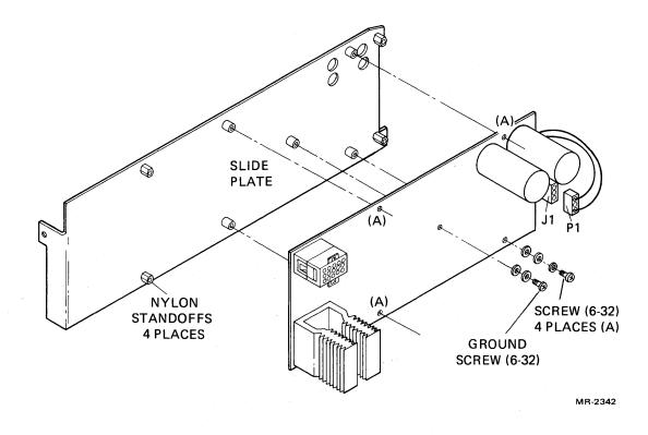
Figure 5-34 Power Supply Module, Removal and Replacement
