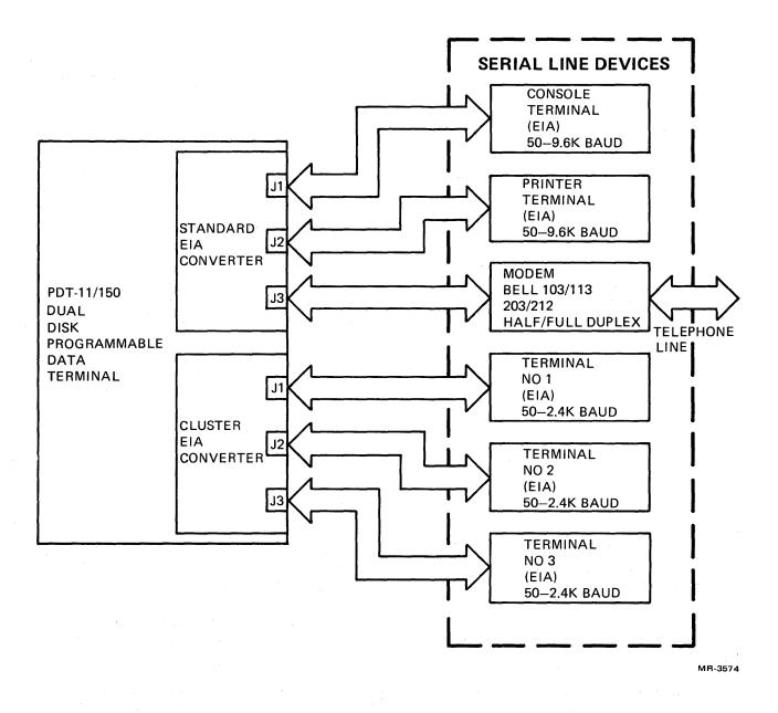
Figure 1-1 Typical PDT-11/150 Flexible (Floppy) Disk Operating System
