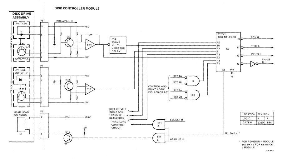
Figure 4-32 Head Load Control and Track and Index Hole Detection
