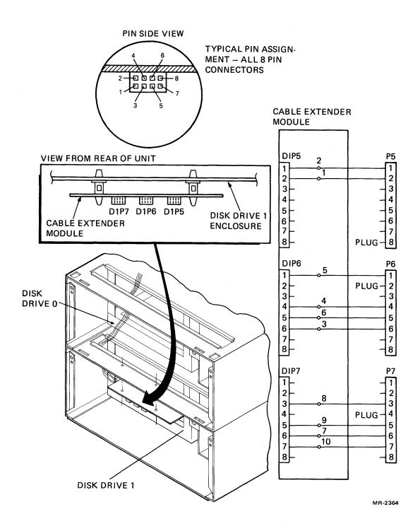
Figure 5-18 Cable Extender, Module Location and Connections
