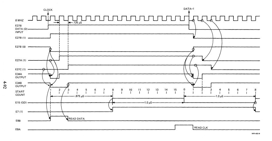
Figure 4-41 Data Separator Circuit (Revision K), Timing Diagram
