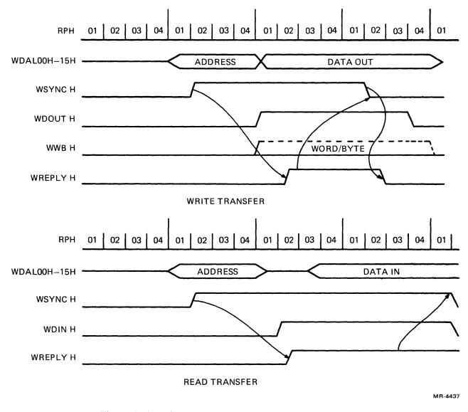
Figure 4-10 LSI-11 Microprocessor, I/O Transfer Timing (Sheet 1 of 2)
