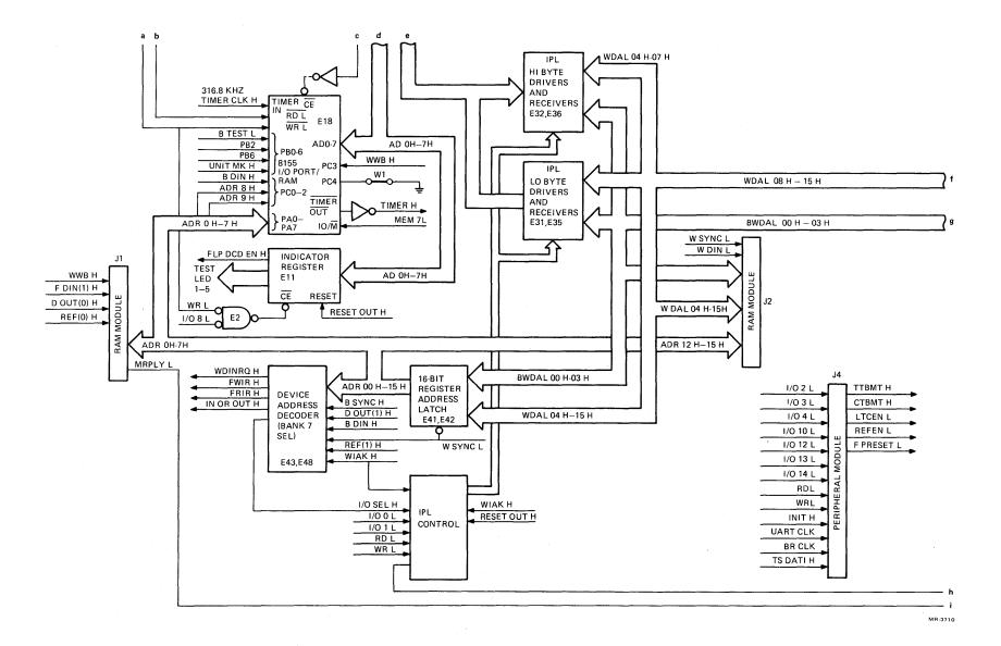
Figure 4-4 Intelligence Module, Simplified Function Diagram (Sheet 2 of 3)
