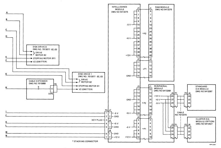
Figure 5-5 AC/DC Power Distribution, 60 Hz Units (Sheet 2 of 2)
