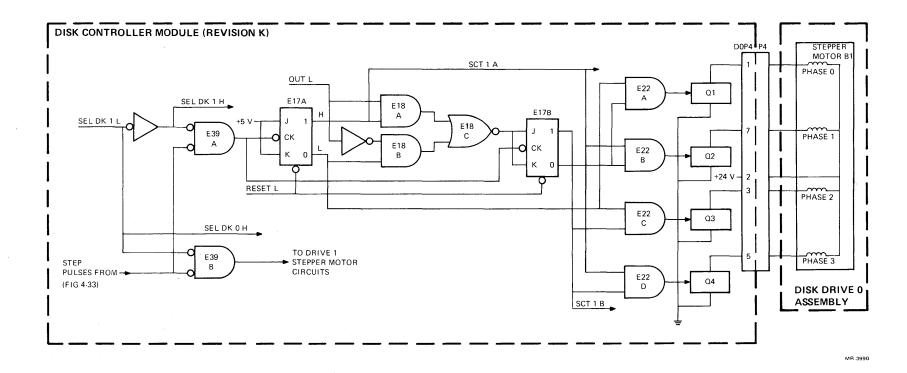
Figure 4-35 Stepper Motor Control and Drive Logic (Revision K), Simplified Diagram
