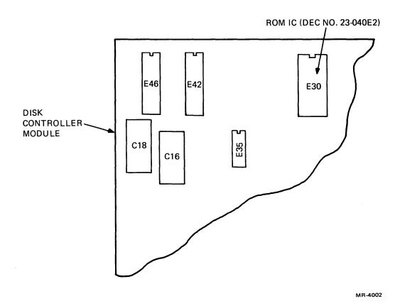
Figure 5-32 Disk Controller Module, ROM IC Location
