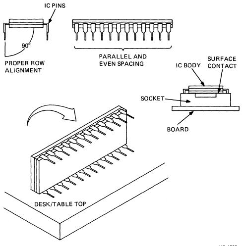
Figure 5-25 ROM IC, Pin Alignment and Mounting
