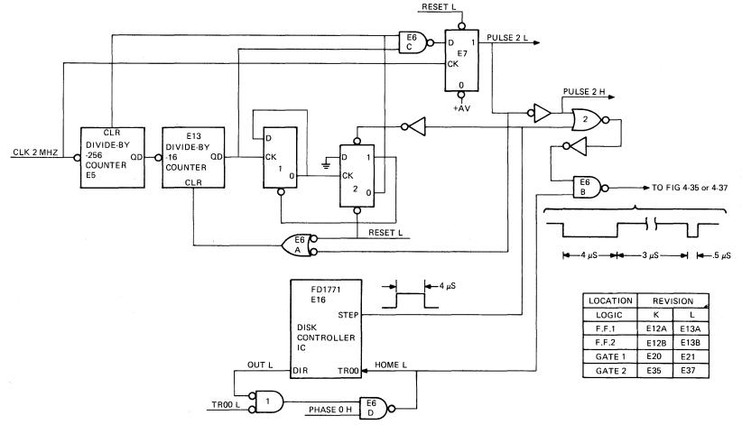
Figure 4-33 Step Generator Circuit, Simplified Diagram
