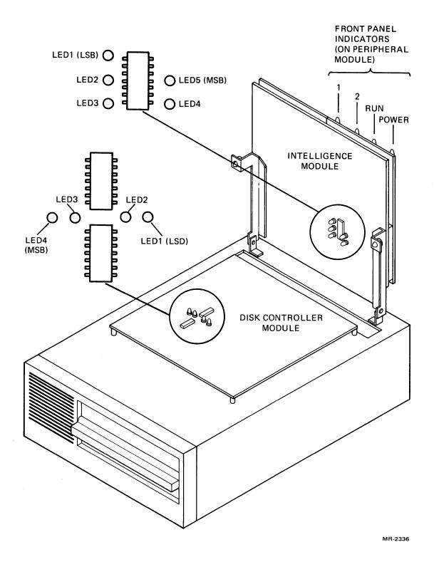
Figure 5-1 Self-Test LED Indicator Locations
