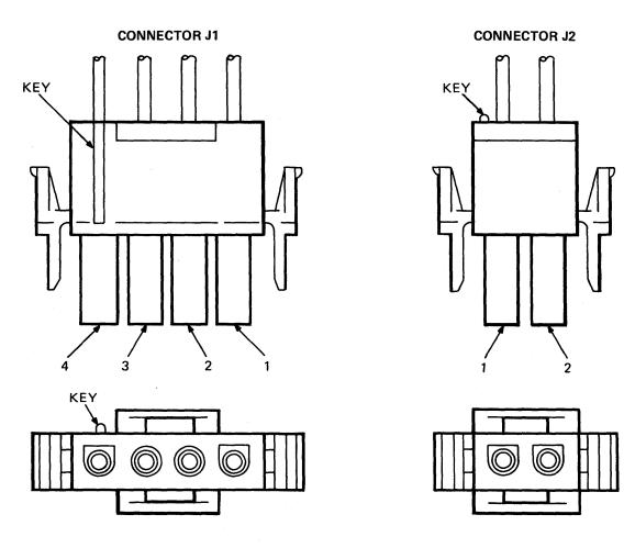
Figure 5-6 Rear Panel Assembly, ac Cable Pin Locations
