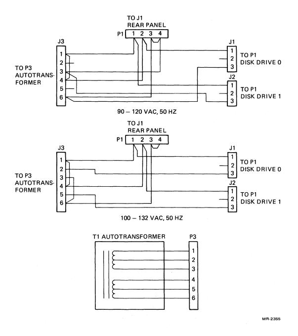
Figure 5-9 50 Hz Internal Cable Configurations (Sheet 2 of 2)
