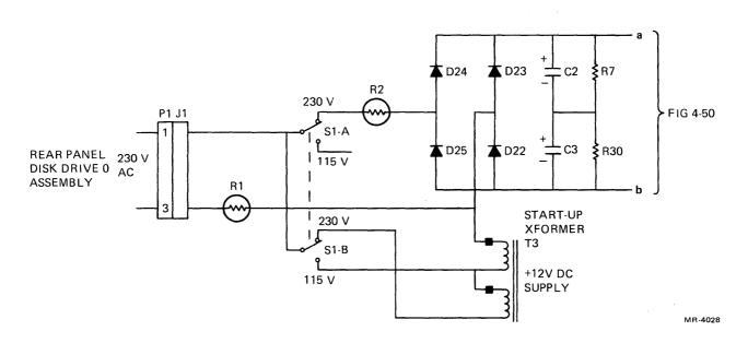
Figure 4-49 230 V ac, Full Wave Rectifier Circuit, Simplified Diagram
