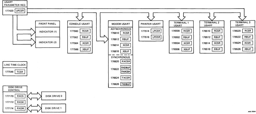
Figure 6-2 PDT-11/150 Device Register Address Assignments
