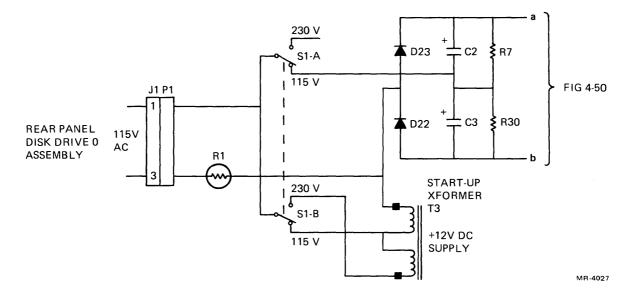
Figure 4-48 115 V ac, Voltage Doubler Circuit, Simplified Diagram
