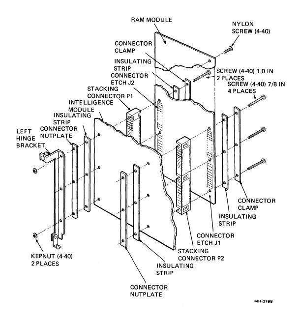
Figure 5-23 RAM Module, Removal and Replacement
