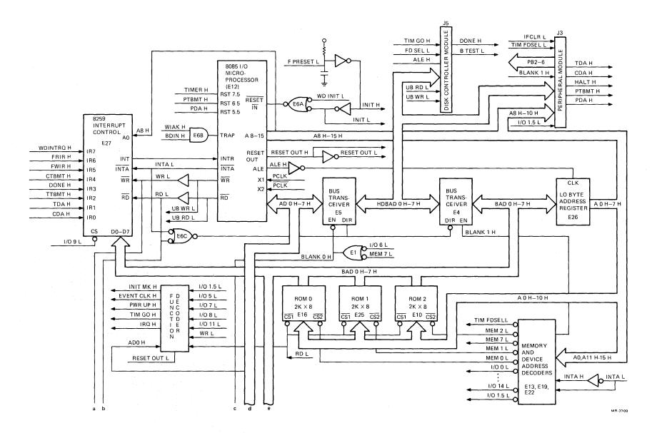
Figure 4-4 Intelligence Module, Simplified Function Diagram (Sheet 1 of 3)
