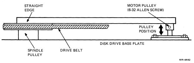
Figure 5-51 Pulley Alignment
