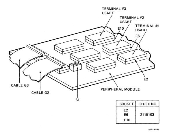
Figure 5-27 Peripheral Module, USART Locations
