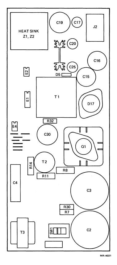
Figure 5-45 Power Supply Module, Component Locations
