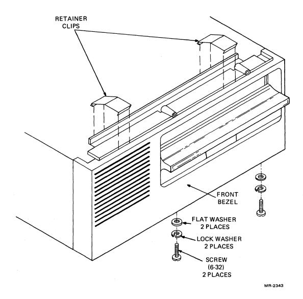
Figure 5-37 Front Bezel, Removal and Replacement
