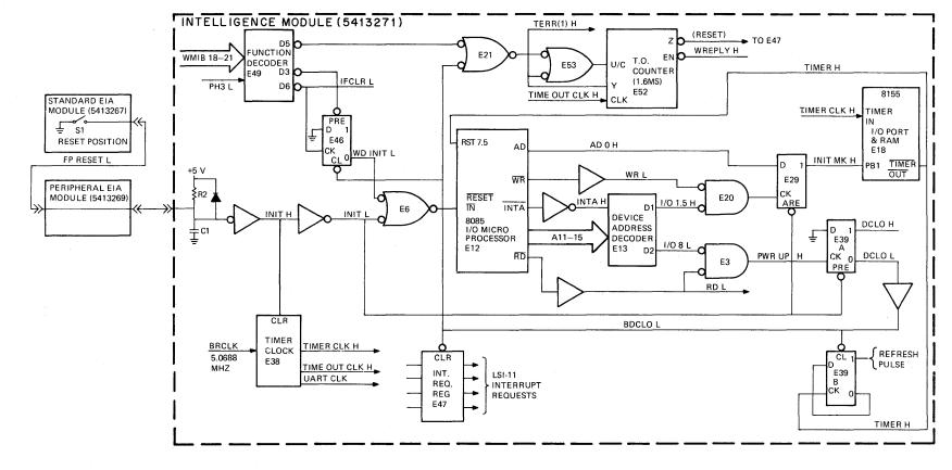
Figure 4-6 Power-up and Manual Reset, Simplified Diagram
