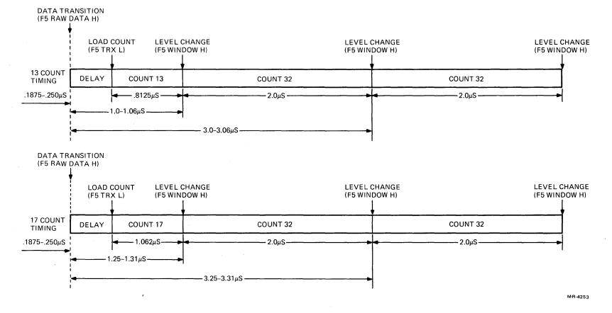
Figure 4-46 13- and 17-Count Intervals, Timing Diagrams
