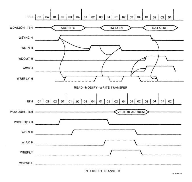
Figure 4-10 LSI-11 Microprocessor, I/O Transfer Timing (Sheet 2 of 2)
