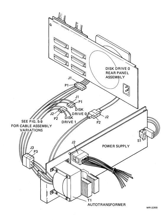
Figure 5-4 Internal ac Cables and Connectors, 50 Hz Units
