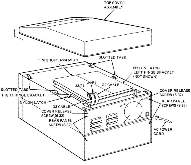
Figure 5-20 Top Cover and TIM Group Assembly, Removal and Replacement
