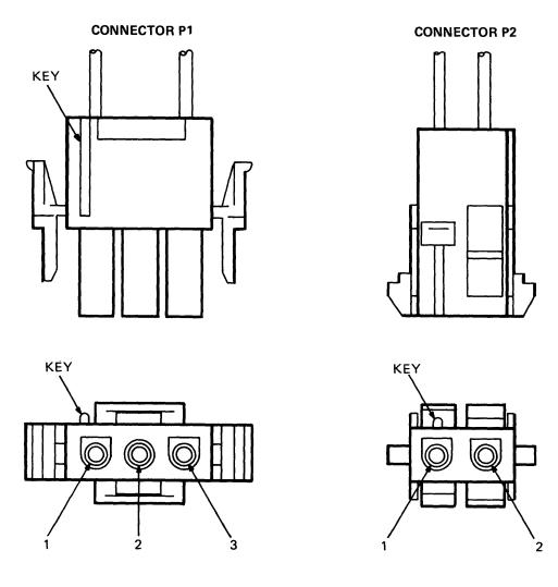
Figure 5-7 Power Supply ac Cable, Connector Pin Locations
