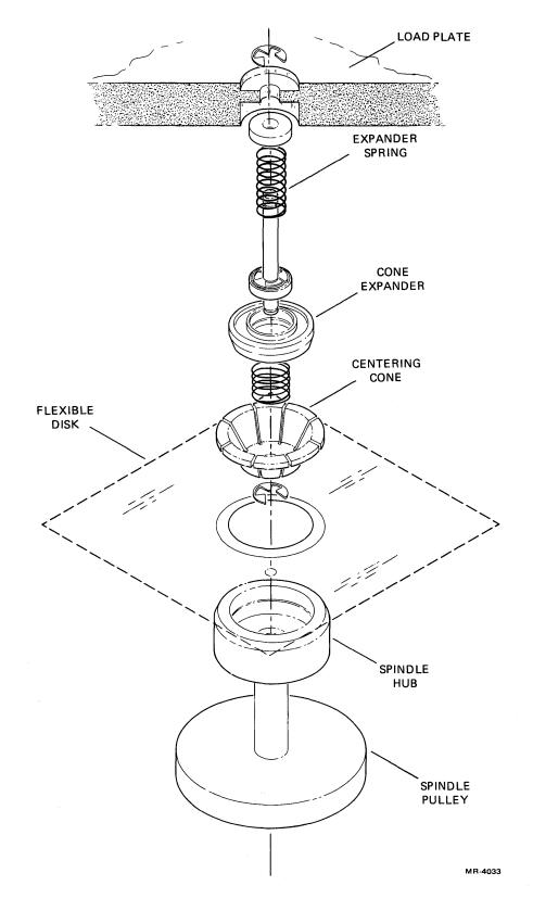
Figure 5-49 Centering Cone and Spindle Drive Components
