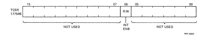
Figure 6-11 Line Time Clock (TCSR) Format
