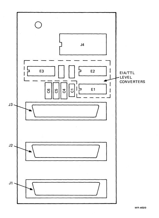
Figure 5-42 Cluster EIA Module, Functional Layout
