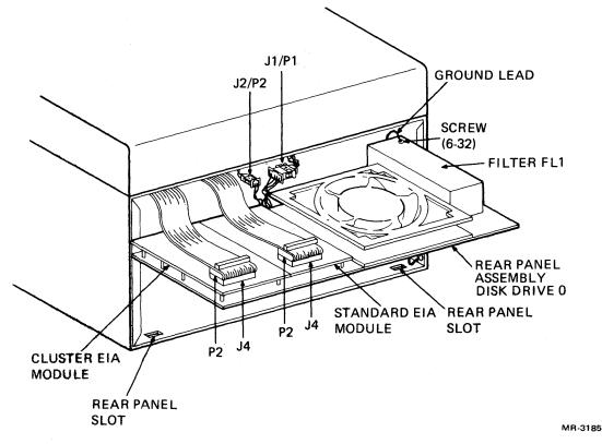
Figure 5-21 Rear Panel Assembly, Removal and Replacement
