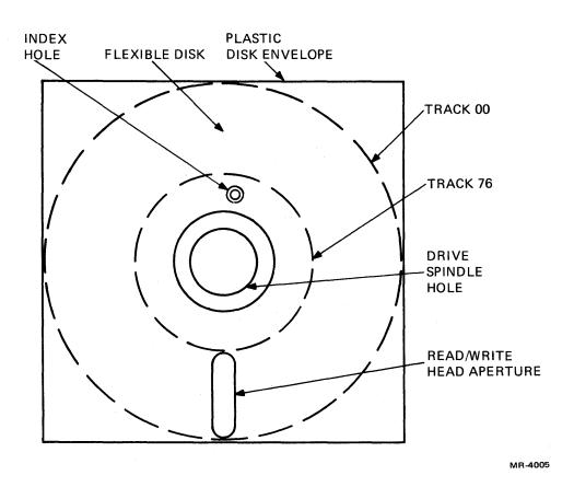
Figure 4-26 Flexible Disk and Envelope
