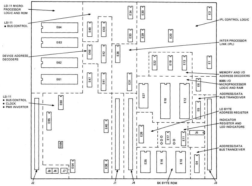
Figure 5-38 Intelligence Module, Functional Layout
