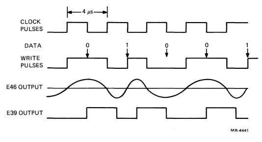
Figure 4-43 Read Amplifier and Differentiator Circuit (Revision K), Timing Diagram
