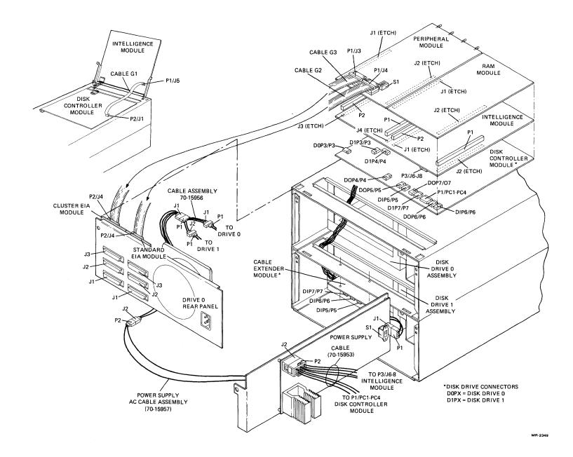
Figure 5-3 PDT-11/150 Internal Cables and Connectors
