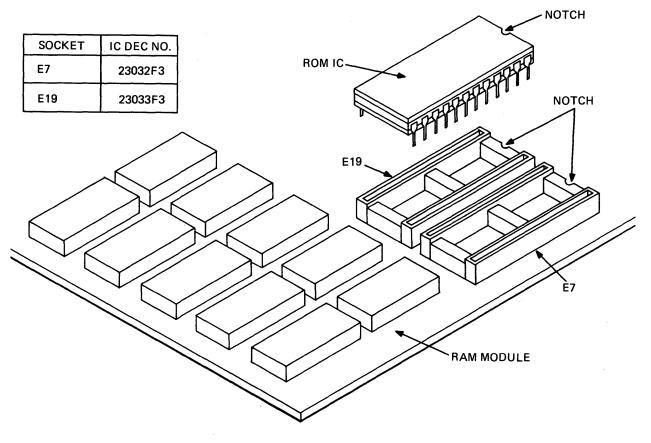
Figure 5-24 RAM Module, ROM IC Removal and Replacement
