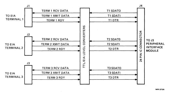
Figure 4-25 Cluster EIA Module, Simplified Diagram
