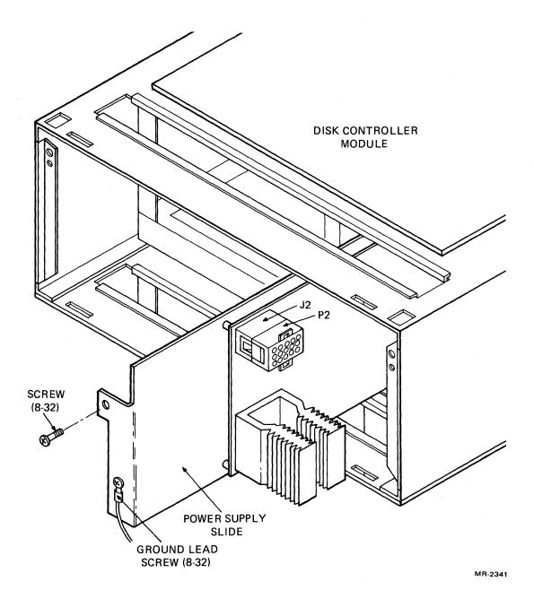
Figure 5-33 Power Supply Assembly, Removal and Replacement
