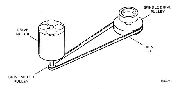
Figure 5-48 Spindle Rotation Mechanism
