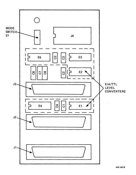
Figure 5-41 Standard EIA Module, Functional Layout
