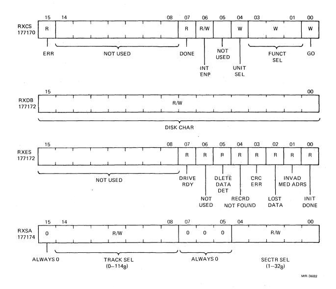
Figure 6-10 Disk Drive Interface Register Formats
