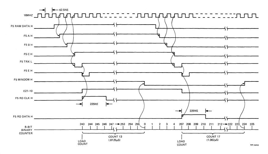
Figure 4-44 Data Separator Circuit (Revision L), Timing Diagram (Sheet 1 of 2)
