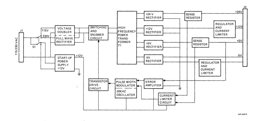
Figure 4-47 H7833 Power Supply, Simplified Block Diagram
