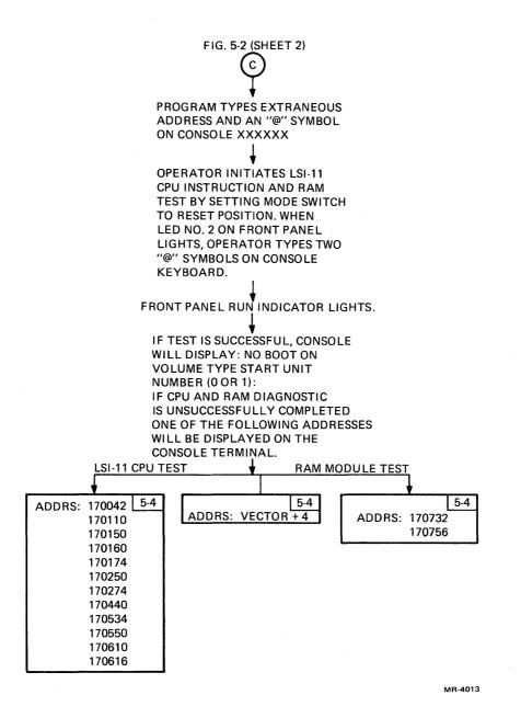
Figure 5-2 Self-Test Sequence Chart (Sheet 3 of 3)
