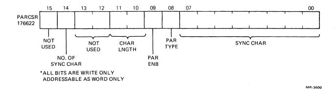
Figure 6-8 Synchronous Communications Parameter Control Register Format
