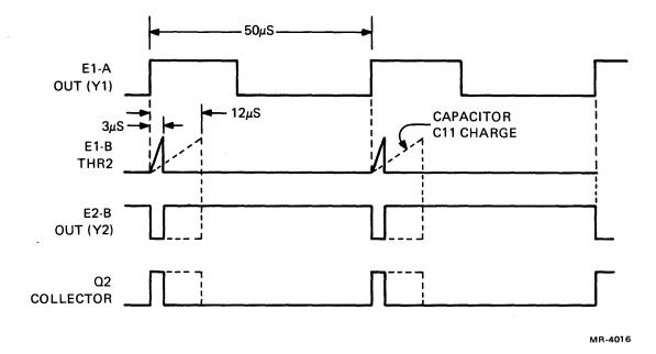
Figure 4-52 Control Circuit, Timing Diagram
