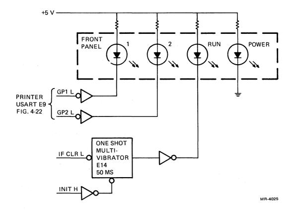
Figure 4-23 Front Panel Indicator Logic, Simplified Diagram
