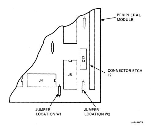
Figure 5-28 Peripheral Module, Jumper Lead Locations
