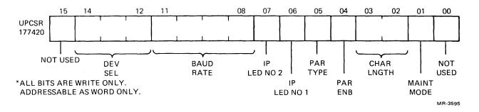
Figure 6-3 USART Parameter Control Register UPCSR Format
