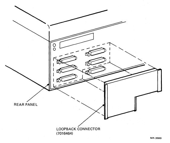
Figure 3-3 Loopback Connector Installation
