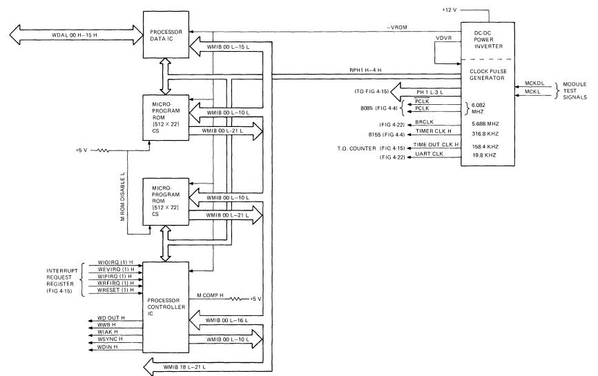
Figure 4-8 LSI-11 Microprocessor, Simplified Block Diagram
