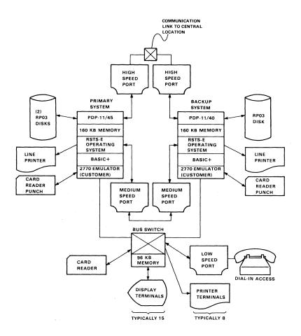
Figure A-7. A typical yard configuration.
