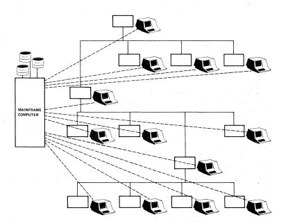
Figure 7-1. An information system can be built using a single, large computer connected to terminals by communication lines.
