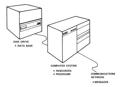
Figure 9-3. A computerized work station has the same components as a manual work station. Messages are received by electronic data communications. The resources are the processing and data storage subsystems. The local data base is on-line data storage. The well-defined procedures are computer programs.
