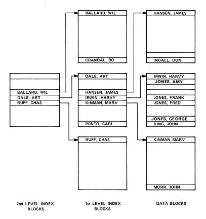
Figure 2-2. Internal file structure of an indexed file. Access to the data blocks is made by using the roadmap provided by the index blocks. Because each index block references many lower-level index blocks (or data blocks), the desired data is found quickly.
