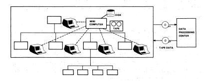
Figure 4-1. A local minicomputer serves the need of a specific department. In this example, data is exchanged with a large computer center in the form of magnetic tape reels.
