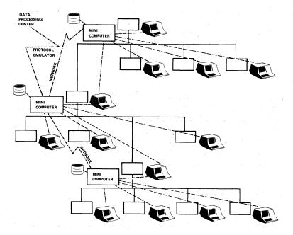
Figure 9-7. A network of interactive minicomputers is connected to a batch-oriented mainframe.
