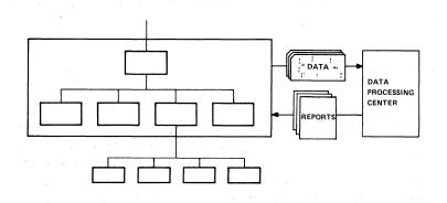
Figure 2-1. Processing needs are met by submitting processing jobs (punched-card decks) to a remote computer center and receiving printed reports.
