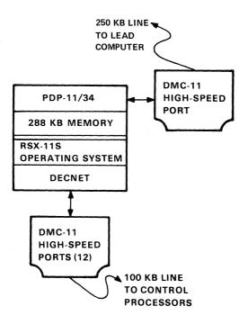
Figure A-11. Concentrator configuration.
