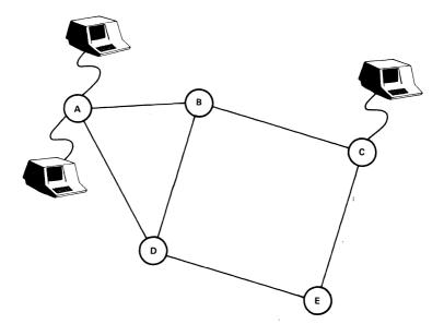
Figure 10-6. Virtual terminal communication services permit a terminal on System C to be used as if it were directly connected to System A.
