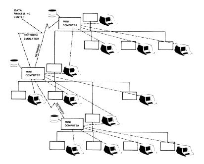
Figure 7-2. An information system can be built using many minicomputers, each serving local departmental needs. In this example, the departmental computers are interconnected into a network, and the network communicates with a central mainframe.
