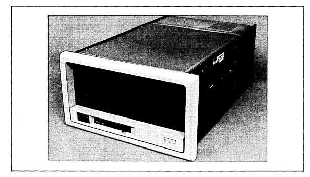
The PDP-11/44 is available in a 10.5 inch rack-mountable version. It offers memory expansion up to 4MB in the four pre-wired slots in the CPU backplane. The PDP-11/44 computer provides ample power and expansion space for configuration flexibility.
