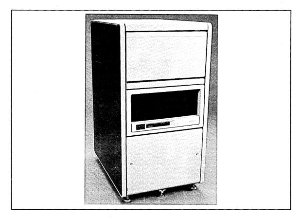
The PDP-11/44 is also available in a cabinet-mounted variation. This configuration is built around the 11/44-DA(DB) box product and housed in an H9642 CPU cabinet. The kernel is intended to provide a foundation for building system configurations tailored for unique applications.
