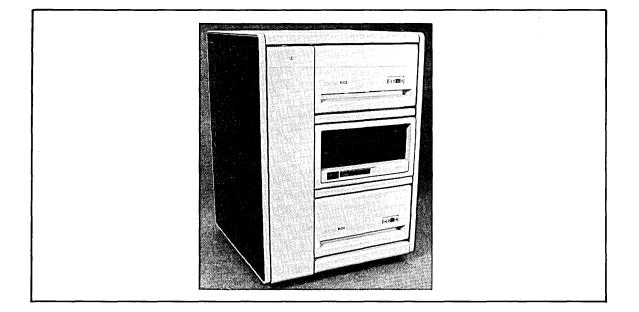
The PDP-11/44 Dual RL02 system configuration provides all the standard features of the PDP-11/44-DA(DB) and 20.8 MB of removable mass storage capacity.
