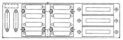
PDP-11/23-S I/O Connection Panel with Panel Insert Units
