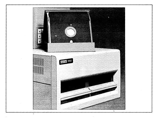
The RX02 double-density floppy disk drive provides an industry-compatible format and highly reliable operation. Direct memory access (DMA) is used to provide rapid data transfer and efficient utilization of the host processor. These subsystems include two RX02 0.5 MB drives (for a total of 1 MB) and a controller with interconnect cabling. The dual drives are packaged as a cabinet-mountable or tabletop unit.
