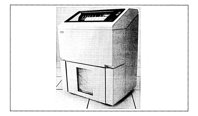
The LP27 band printer is a 132-column impact printer that prints fully formed characters. Print speed is 1200 lines per minute using a 64-character band or 910 lines per minute using a 96-character band. Printer bands are easily interchangeable and available in a variety of fonts.
