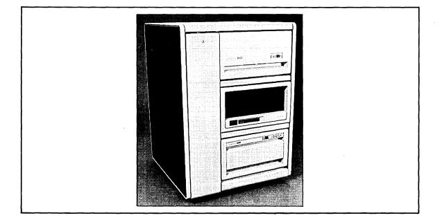
The PDP-11/44 RA80/RL02 system provides all the standard features of the PDP-11/44-DA(DB) box product plus an expansion backplane and 121 MB fixed and 10.4 MB removable disk storage.
