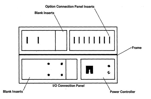
The shielded UNIBUS I/O Connection Panel, located at the back of the CPU cabinet, is comprised of two or more interlocking frames, option panel inserts and blank inserts that are used to maintain shielding continuity. The I/O connection panel is bolted horizontally on the back lowest section of the H9642 cabinet and is bolted vertically on the left rear of the H9645 wide cabinet.
