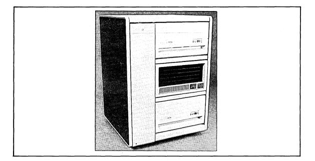
The PDP-11/24 Dual RL02 system configuration provides all the standard features of the PDP-11/24 DC(DD) box product plus 20.8MB of disk storage capacity.
