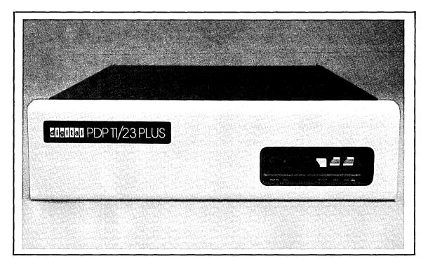
The PDP-11/23-PLUS is avaiable in two 5.25 inch rack-mountable variations. This box is expandable with a BA11-SE(SF) box and the BCV2A-03 expansion assembly. The PDP-11/23-PLUS rack-mountable CPU box includes:
