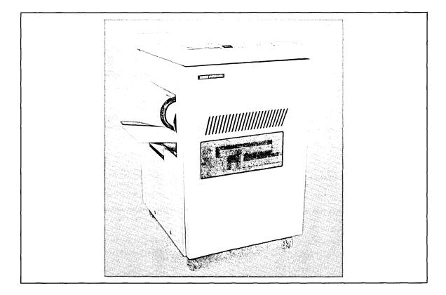
The LN01 page printer is a high-quality nonimpact printer that employs laser technology. The LN01 provides the speed of a lineprinter with exceptional print quality. Using electrophotographic imaging and xerographic printing, the LN01 prints one page at a time, twelve pages per minute. The print resolution of 300-by-300 dots per inch produces perfectly formed characters of even density and alignment. Since every page is an original, every copy is as crisp and clear as the first.
