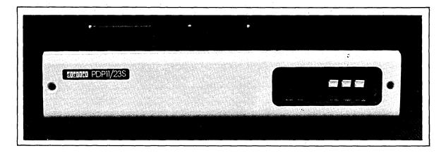
The PDP-11/23-S is a 3.5 in high, rack-mountable processor offered in two versions, one with RAM memory, the other with non-volatile CMOS memory. The I/O Connection panel (H3012) for this model accepts the same system options as the MICRO/PDP-11 and the PDP-11/23-PLUS.
