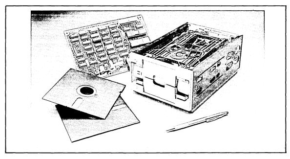
The RX50 dual diskette drive is a low-cost, compact, random access mass memory subsystem that stores data in fixed-length blocks on two 5.25-inch flexible diskettes with preformatted industry-standard headers.
