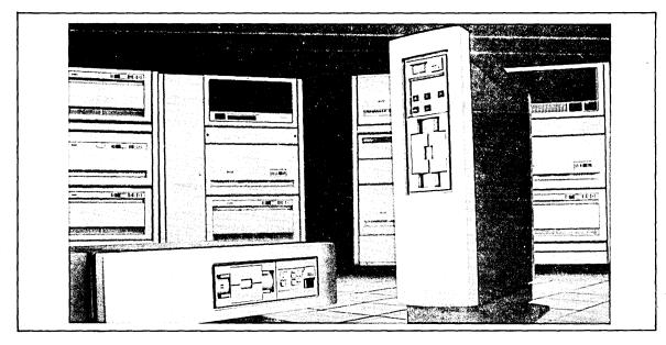
The MICRO/PDP-11 family of small, multiuser computers consists of both floppy-disk and fixed-plus-floppy systems. They are packaged to fit easily under a desk or worktable, on a tabletop, or as a rack mountable box enclosure, and can be expanded to support up to 10 users.
