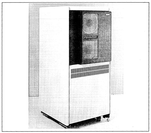
The TU77 magnetic tape subsystem includes the controller, a tape formatter, and one nine-track TU77 tape transport. The TU77 tape transport uses industry-compatible recording densities of 1600 b/in (Phase Encoded) and 800 b/in (Non-Return to Zero Inverted) selectable under program control. The subsystem is available with controllers for UNIBUS PDP-11 systems. The TU77 tape transport is available mounted in a 60 in (152.4 cm) H9602 single-width high cabinet.
