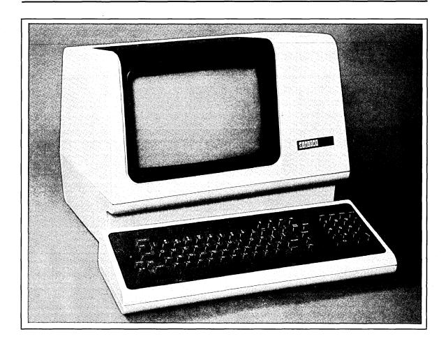
The VT100 family of video display terminals is designed to make the first-time user feel comfortable. A sculptured typewriter-like detachable keyboard connects to the video display unit by means of a 1.9 m (6-foot) coiled cord. The keyboard is used to set the terminal's functions. You can customize the display—set up tab stops, reverse the video image, and change the cursor from underline to block—to suit your application.
