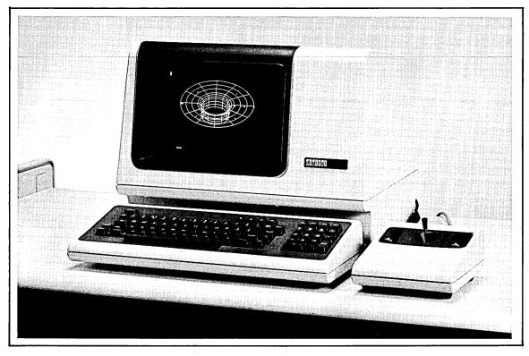
The VS11 comprises a family of video graphic subsystems: the VSV11 for an LSI-11 bus host and the VS11 for a UNIBUS host. The basic elements of these systems are an image processor, image memory and sync generator. They are all quad-sized modules designed to plug into an LSI-11 bus C-D interconnect-type backplane. Included with the VS11 is a SW11-BK bus converter for use on a UNIBUS host.
