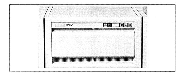
The RA80 disk subsystem uses Winchester fixed-disk technology to provide 121 MB of storage in a 10.5-inch high package. The RA80 uses the high-performance, high-reliability microprocessor-based controller, the UDA50. The RA80 disk offers exceptional throughput performance, the result of an advanced mechanical design, which incorporates a rotary servo-motor, computer-designed positioner arms, and lightweight Winchester head suspension.
