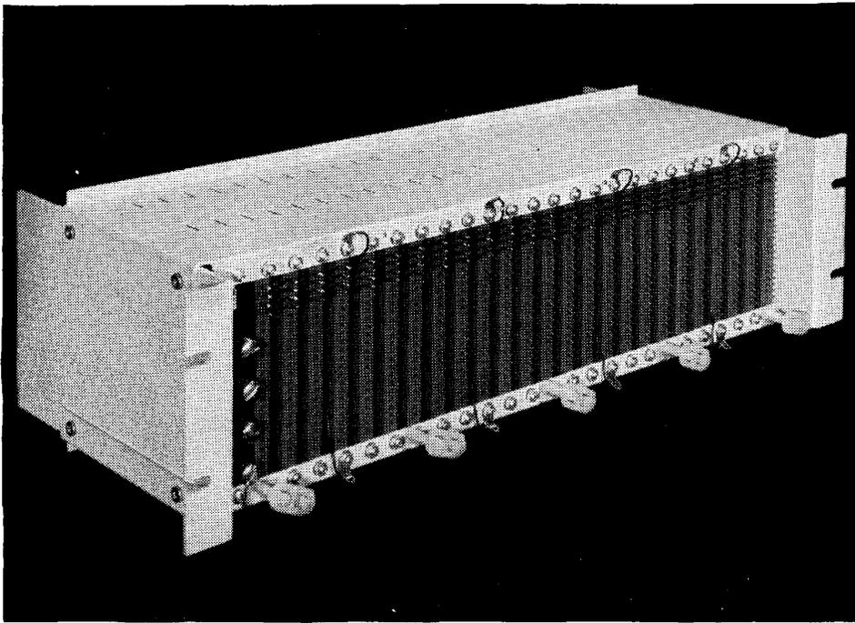
FRONT VIEW OF DEC SYSTEM MODULE MOUNTING PANEL
