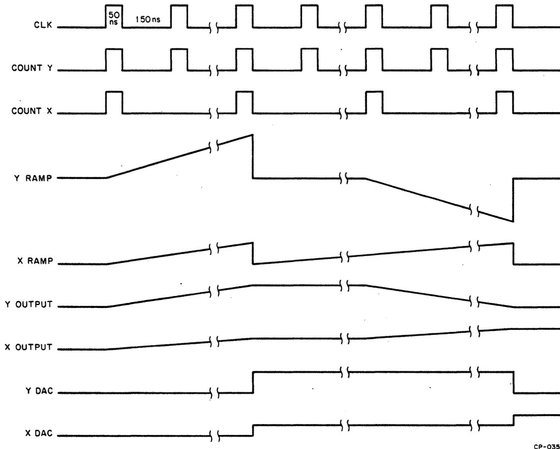
Figure 3-25 Vector Generator, Timing Diagram
