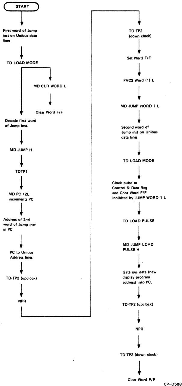
Figure 3-13 Jump Instruction Flow Diagram
