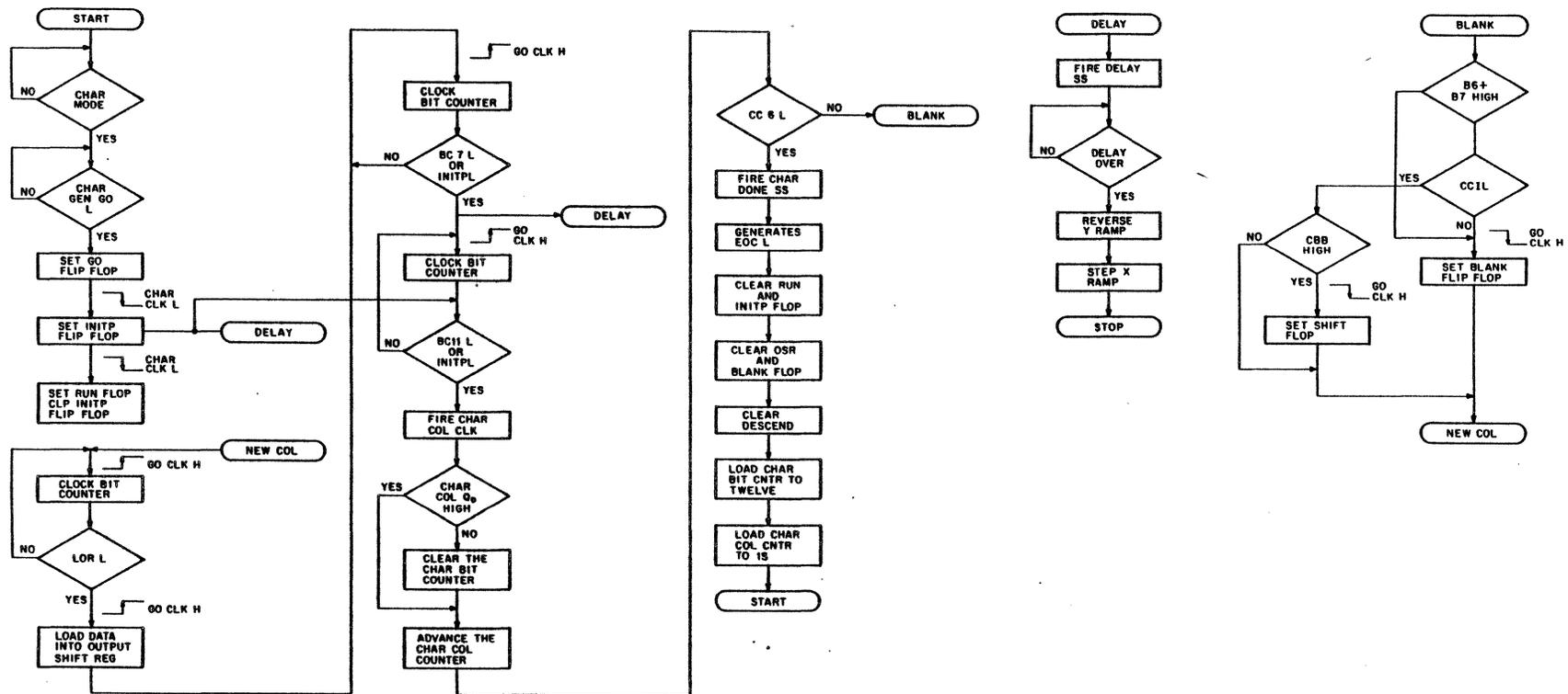
Figure 3-30 Character Generator, Flow Diagram
