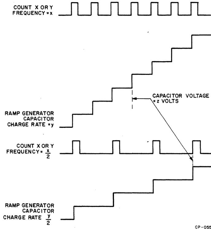
Figure 3-24 Relationship of Clock Frequency to Ramp Generator Output
