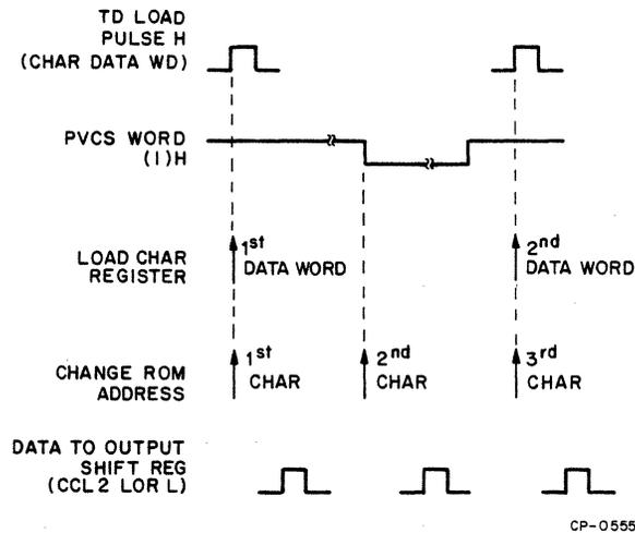
Figure 3-34 Word Selection and ROM Addressing, Timing Diagram
