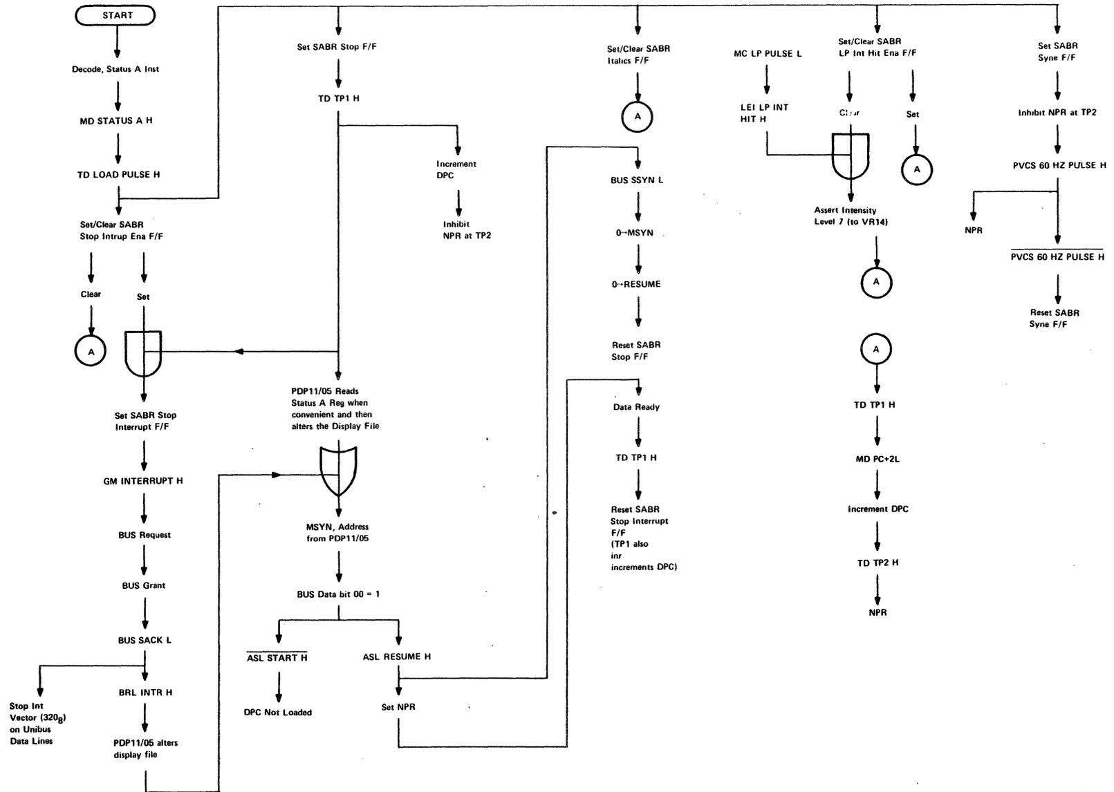
Figure 3-9 Status A Instruction Flow Diagram
