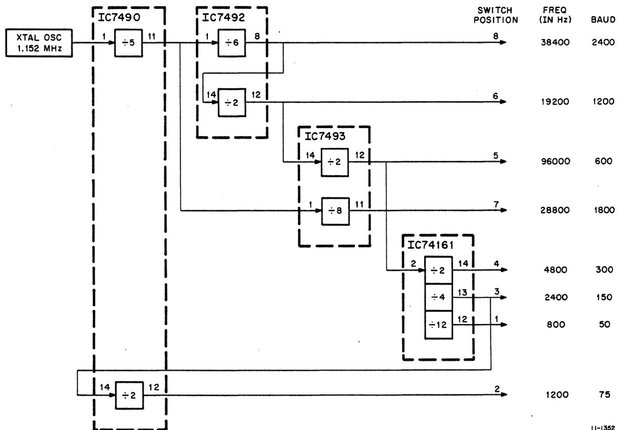
Figure 3-63 Frequency Divider Logic, Simplified Diagram
