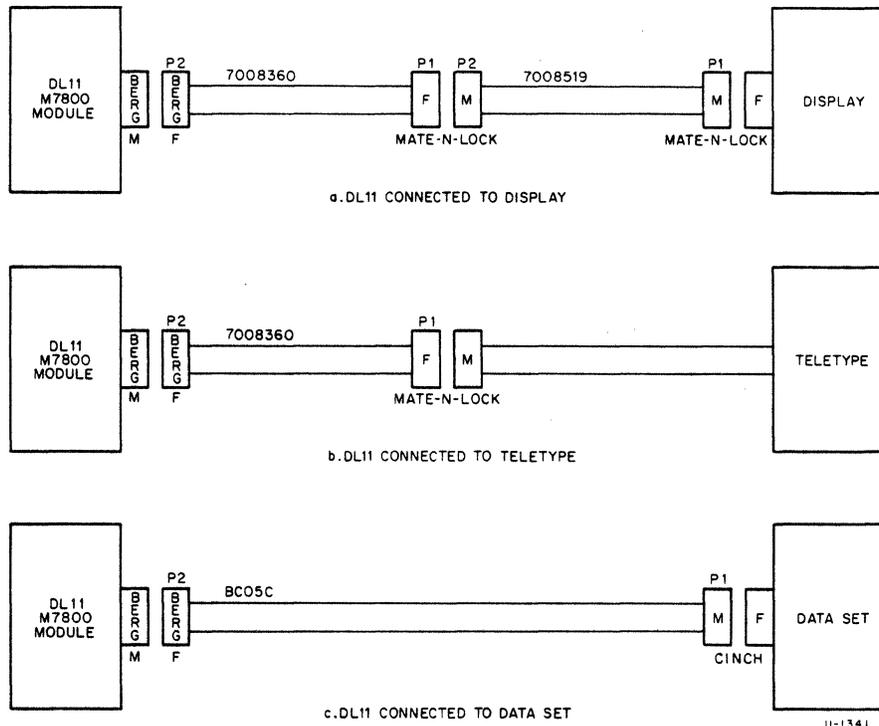
Figure 3-48 DL11 Cable Connections
