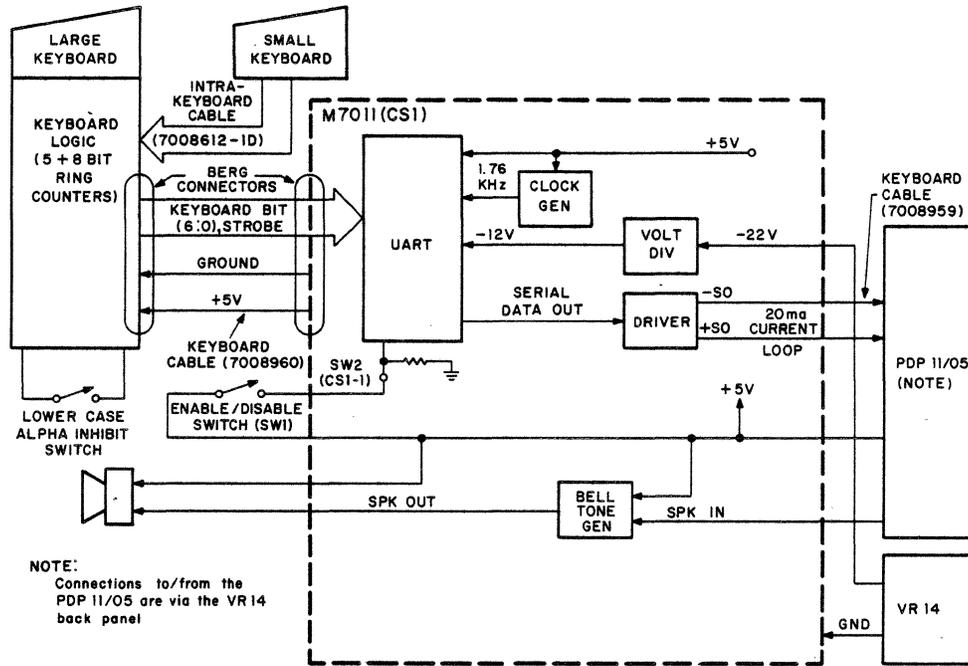
Figure 3-66 LK40 Keyboard, Block Diagram
