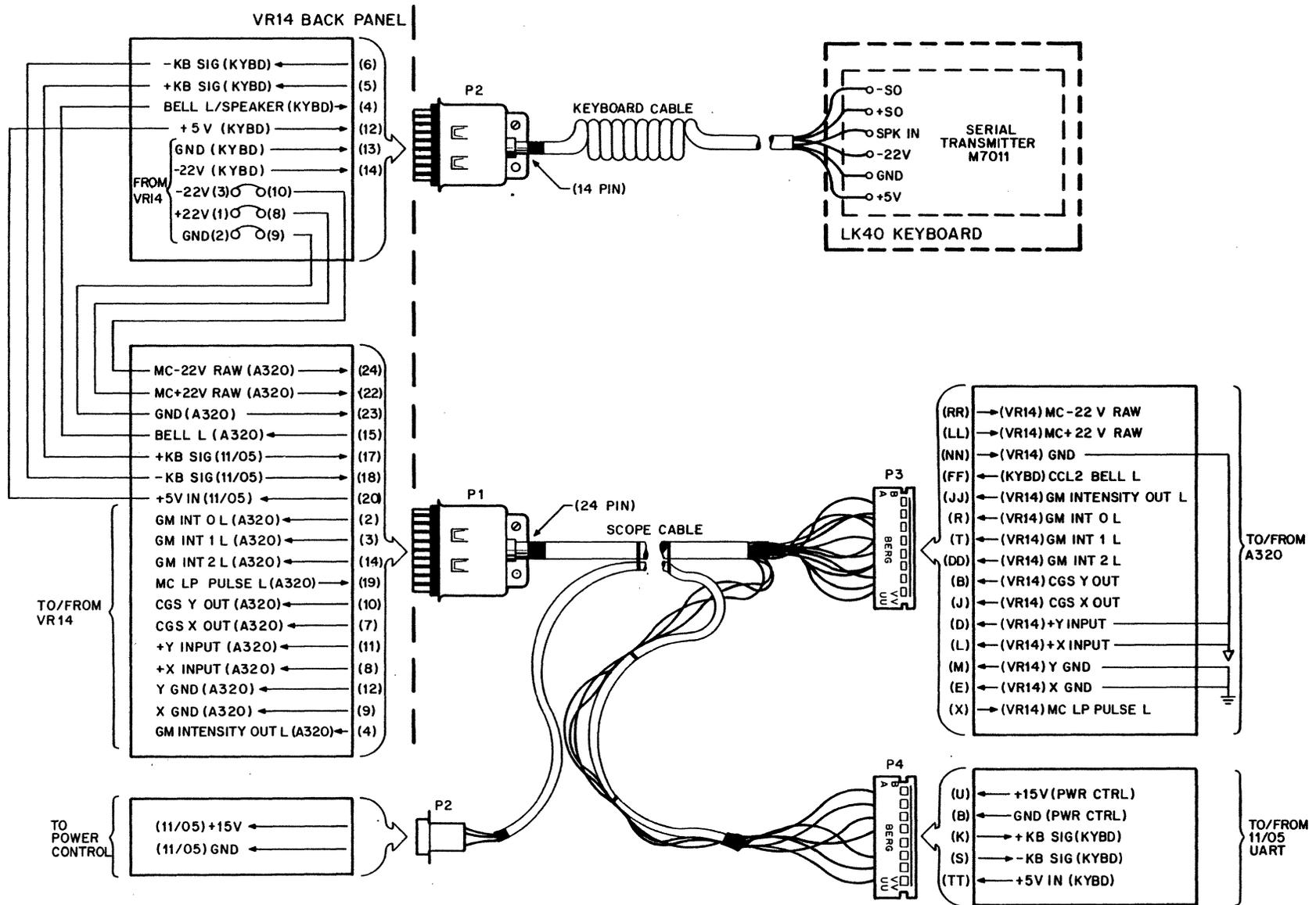
Figure 3-70 Scope and Keyboard Cables
