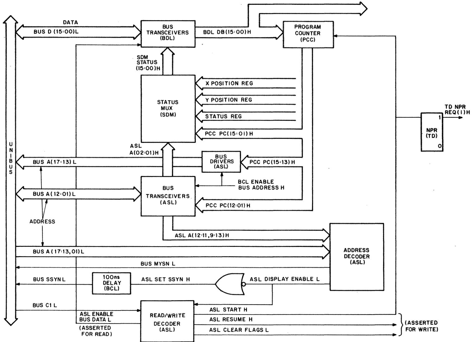
Figure 3-1 Unibus Address and Data, Block Diagram
