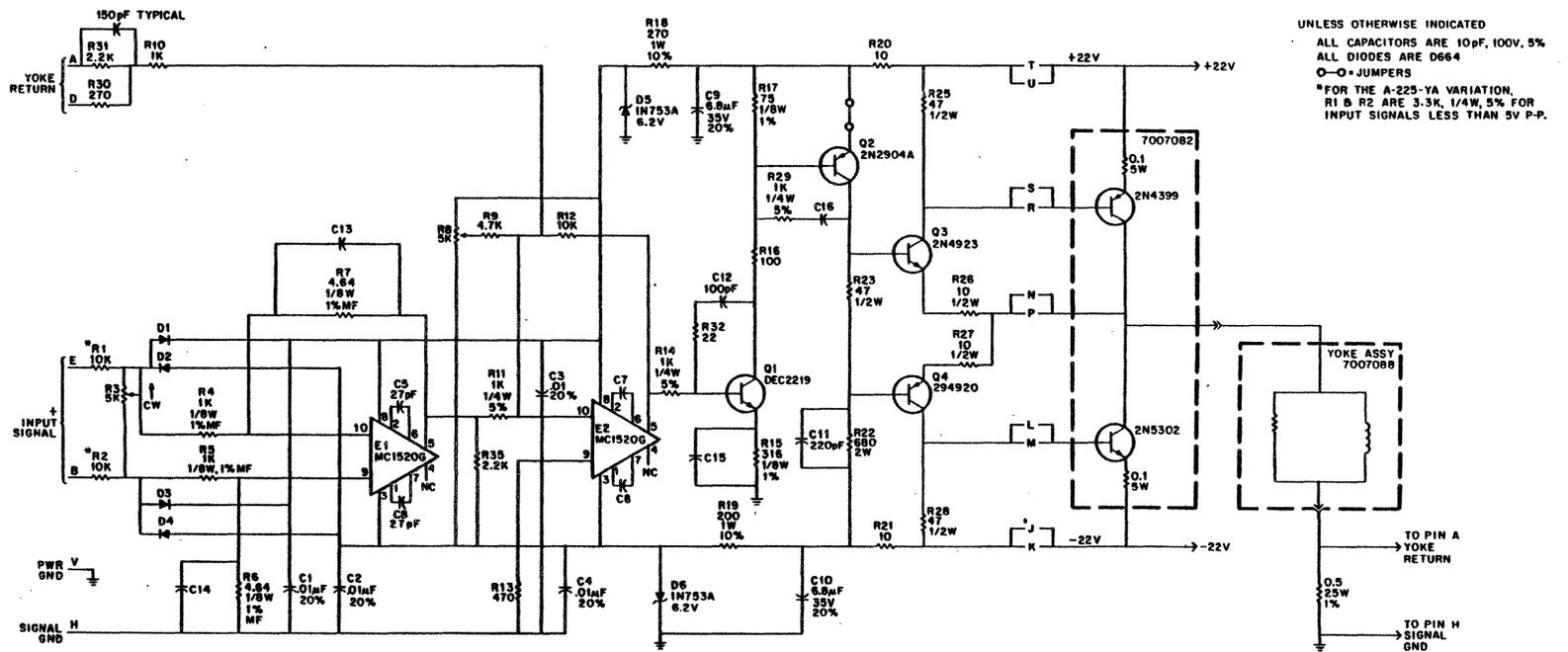
Figure 3-71 X and Y Deflection Circuit
