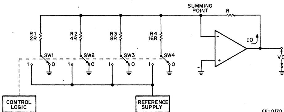
Figure 3-45 Typical Current Summing Ladder
