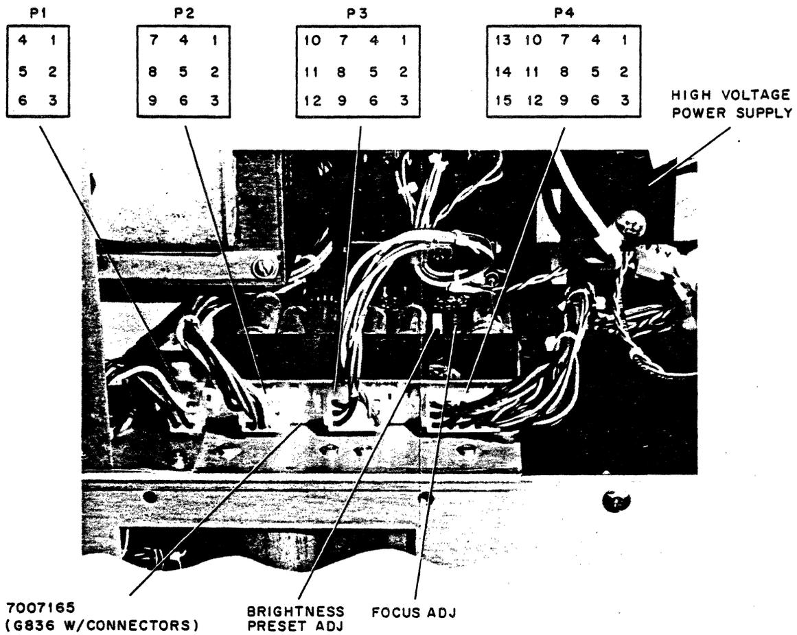
Figure 4-30 VR14 CRT Display Interior View, Top
