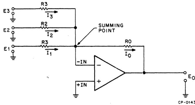
Figure 3-46 Summing Amplifier Configuration
