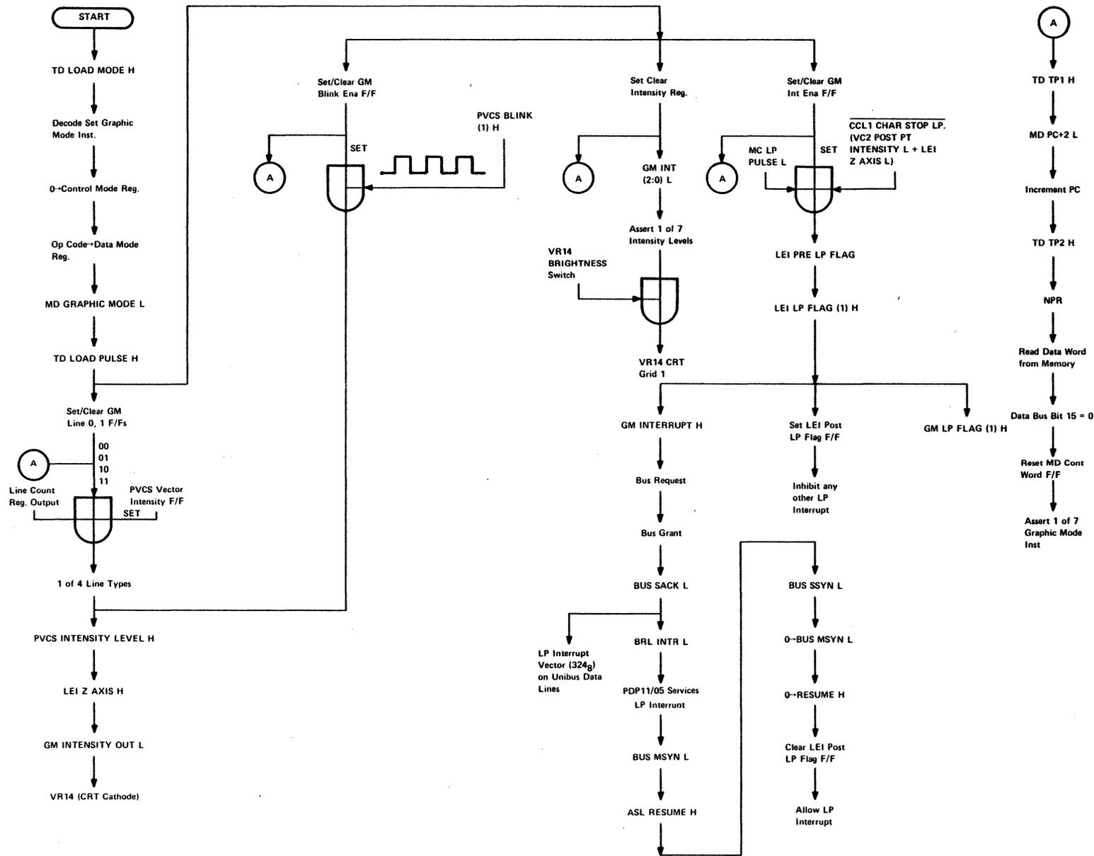
Figure 3-14 Set Graphic Mode Instruction, Flow Diagram
