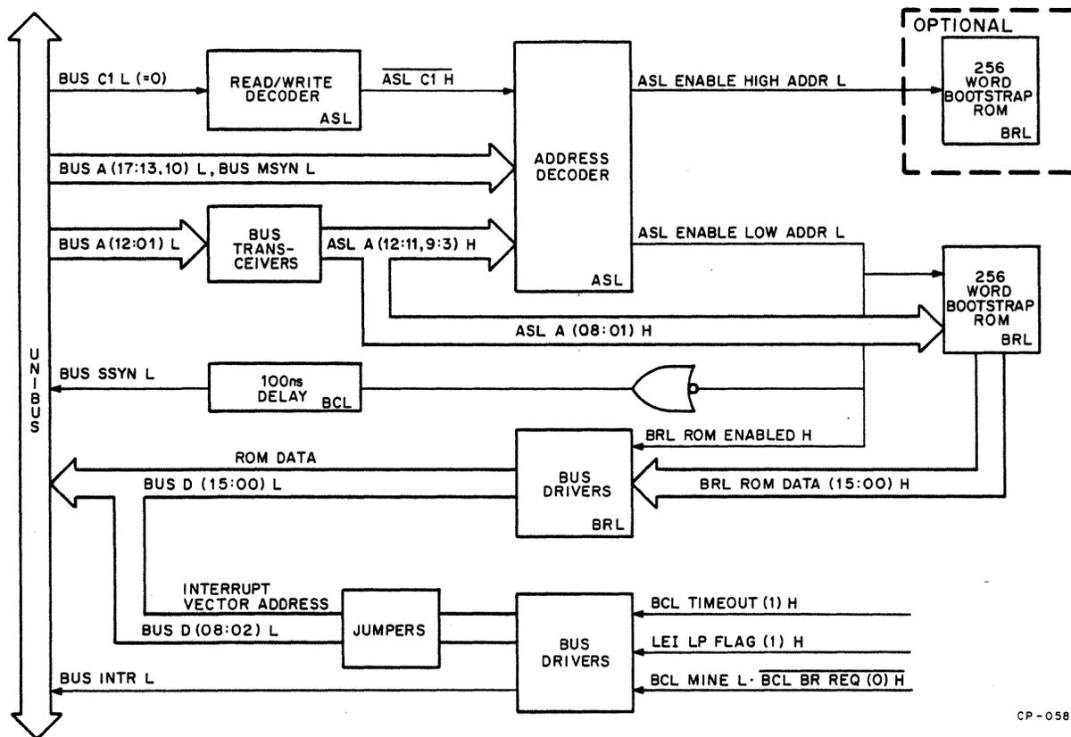
Figure 3-47 Unibus ROM and Interrupt Vector Address and Data, Block Diagram
