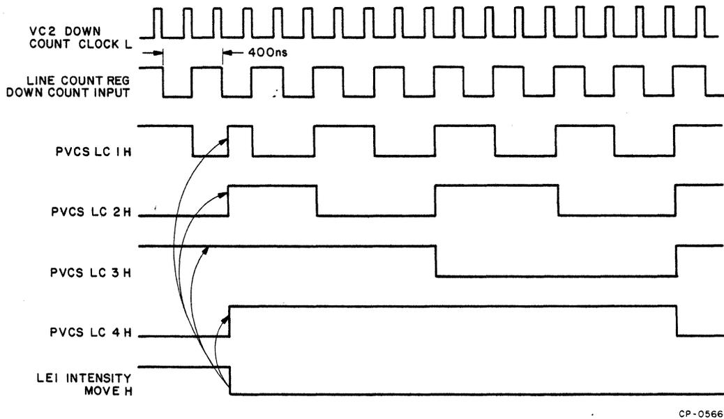
Figure 3-15 Line Count Register, Timing Diagram
