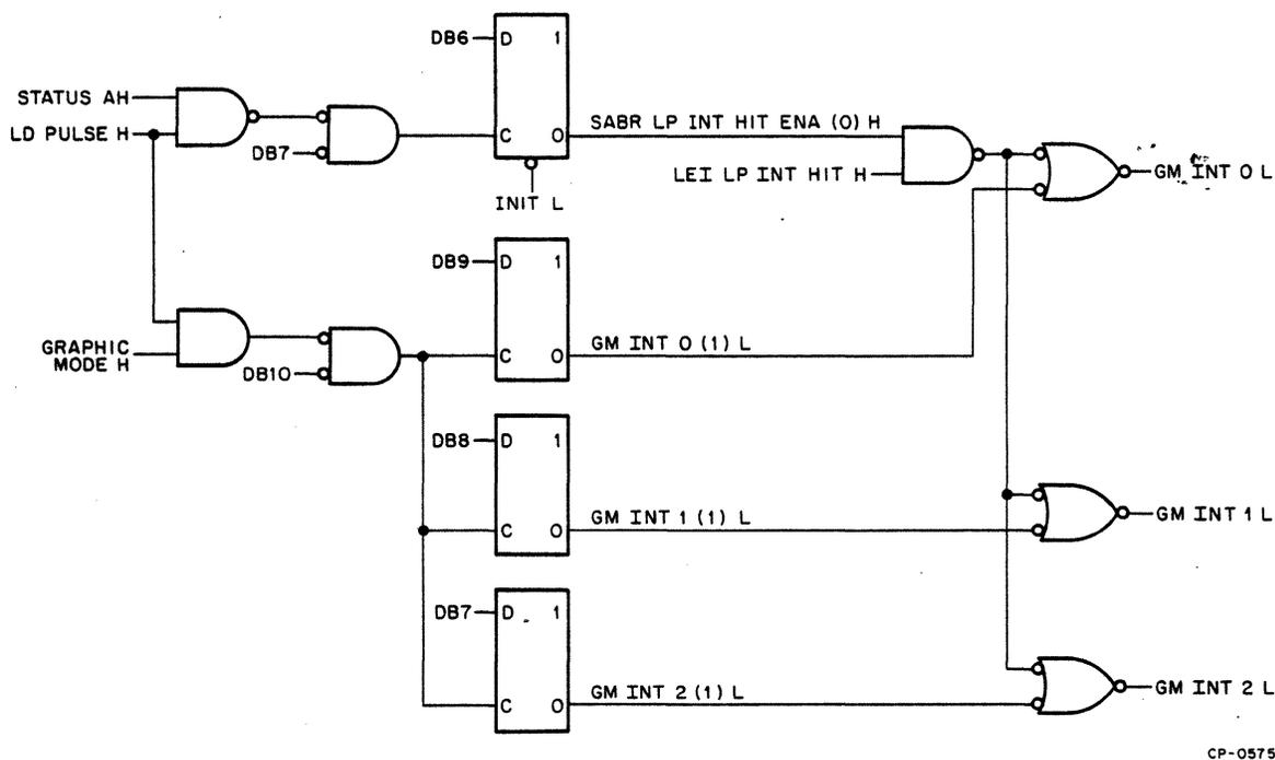
Figure 3-10 M7013 Intensity Level Control
