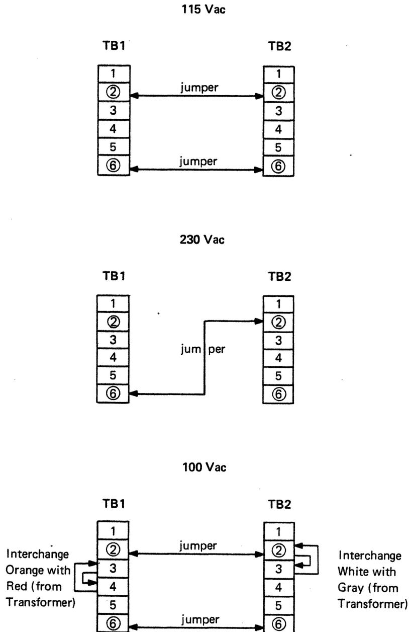
Figure 3-69 Input Power Jumper
