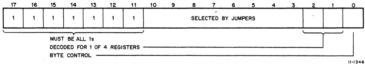
Figure 3-53 Interface Address Format
