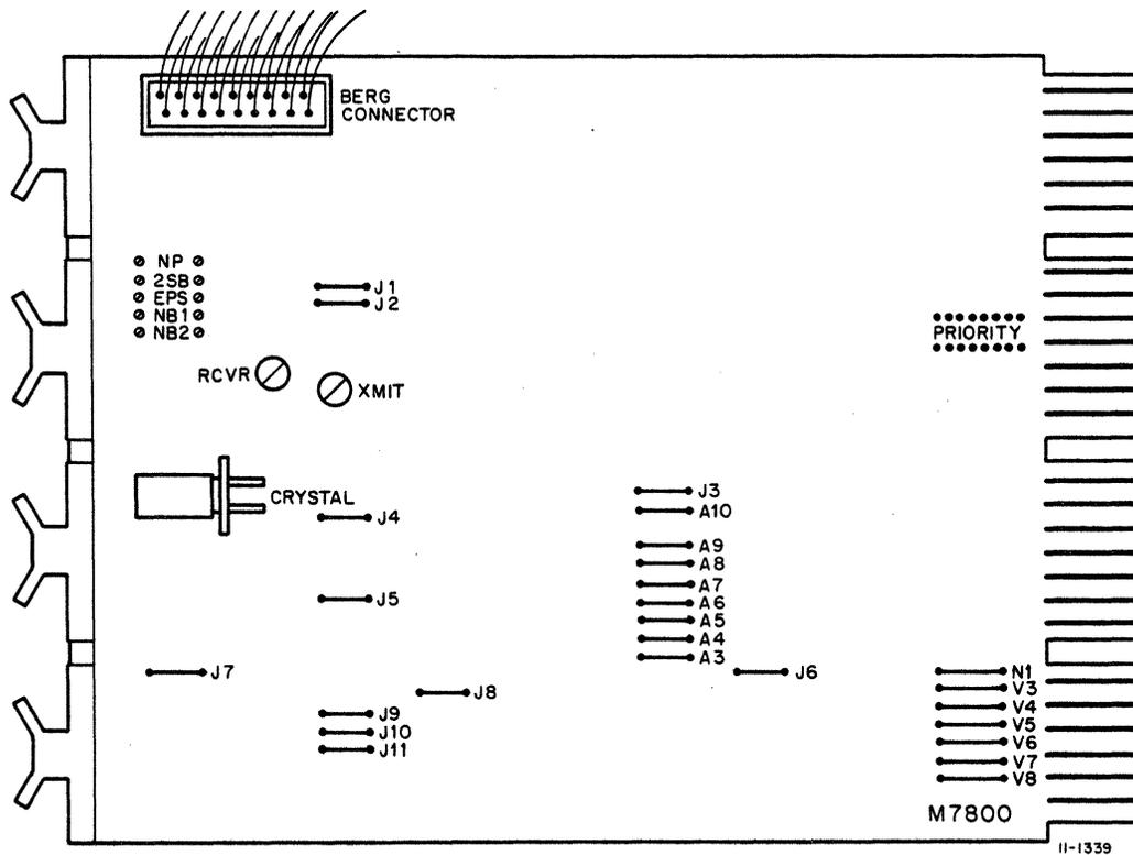
Figure 3-51 Crystal Switch and Jumper Locations, M7800 Module
