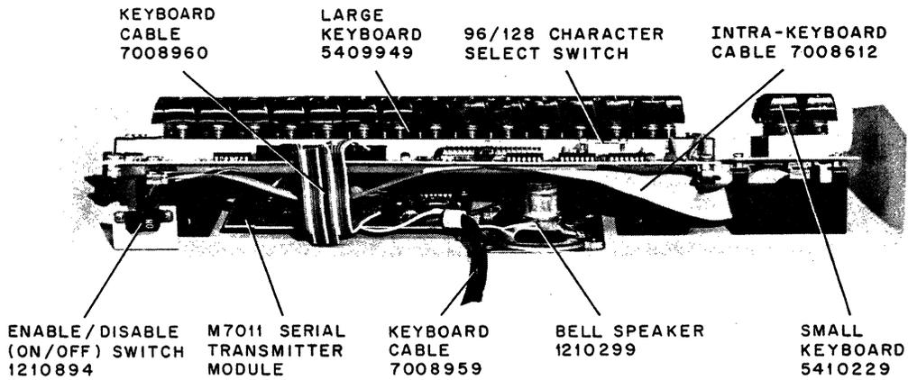
Figure 4-29 LK40 Keyboard Interior View, Rear
