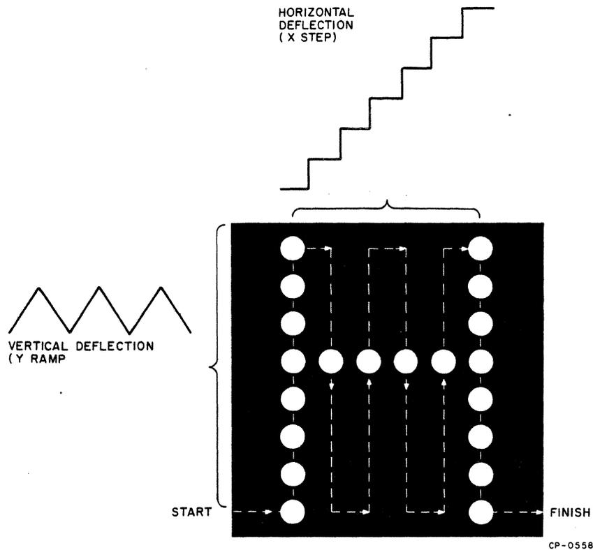
Figure 3-28 Path of Electron Beam as Influenced By X and Y Deflection Signals
