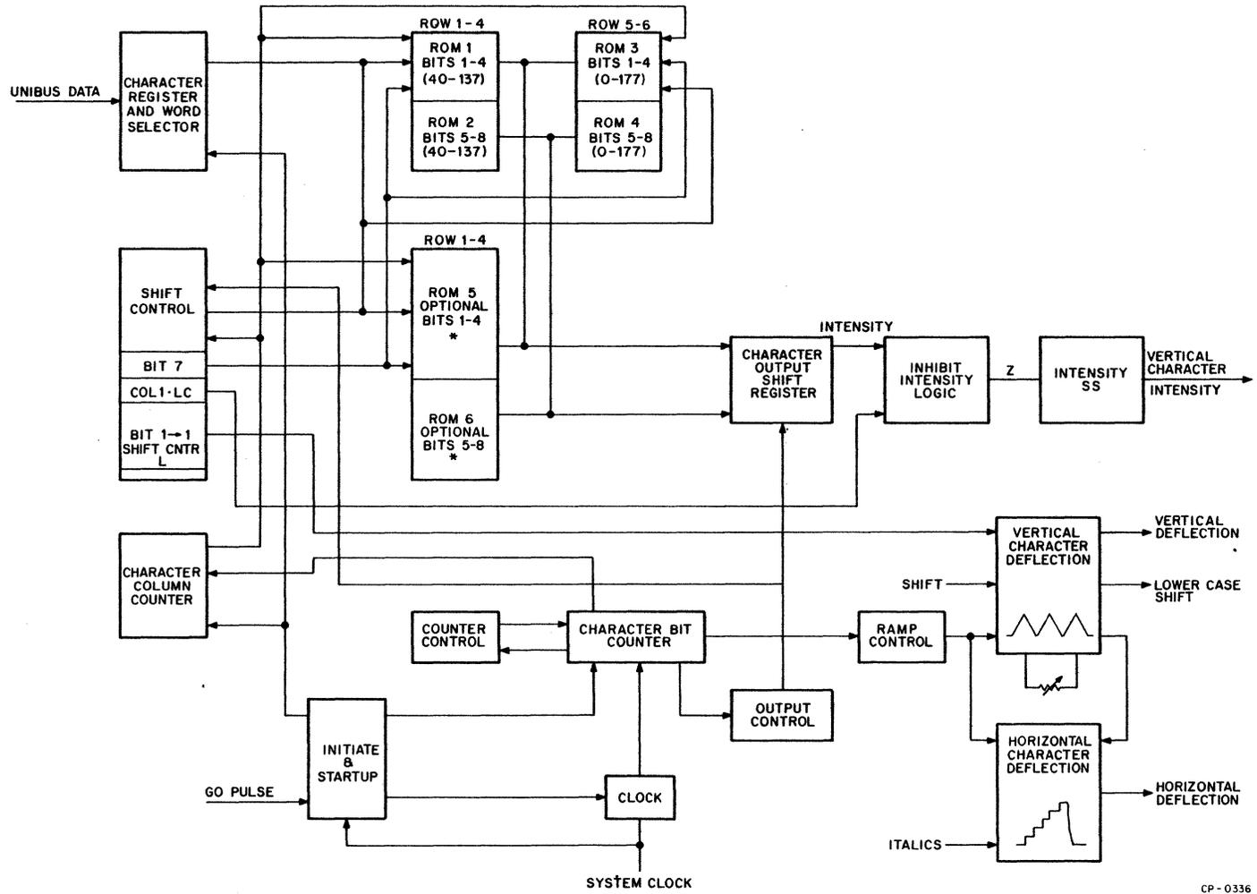
Figure 3-29 Character Generator, Block Diagram
