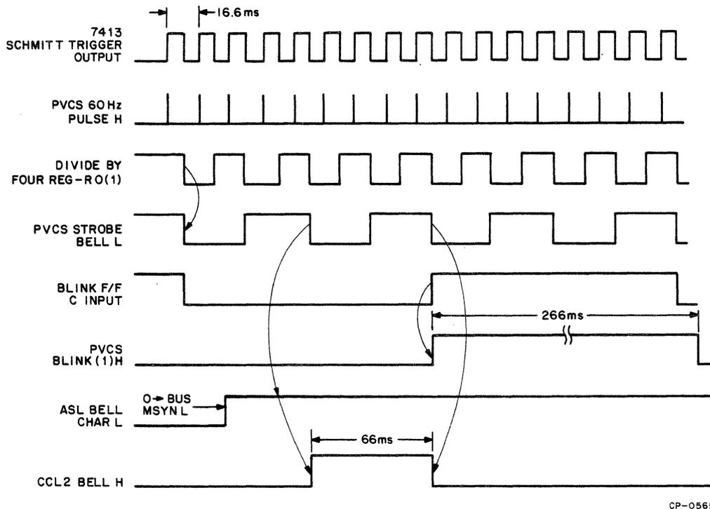
Figure 3-16 Bell Tone and Blink Timing Diagram
