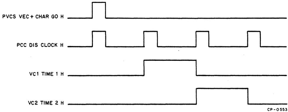
Figure 3-38 Time Shift Register, Timing Diagram (M7014-VC1)
