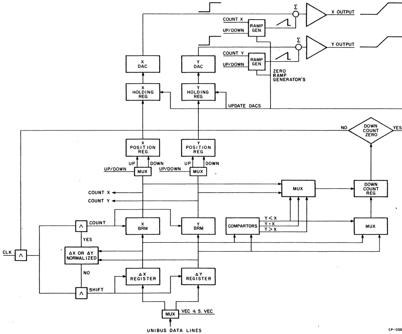
Figure 3-23 Vector Generator, Block Diagram
