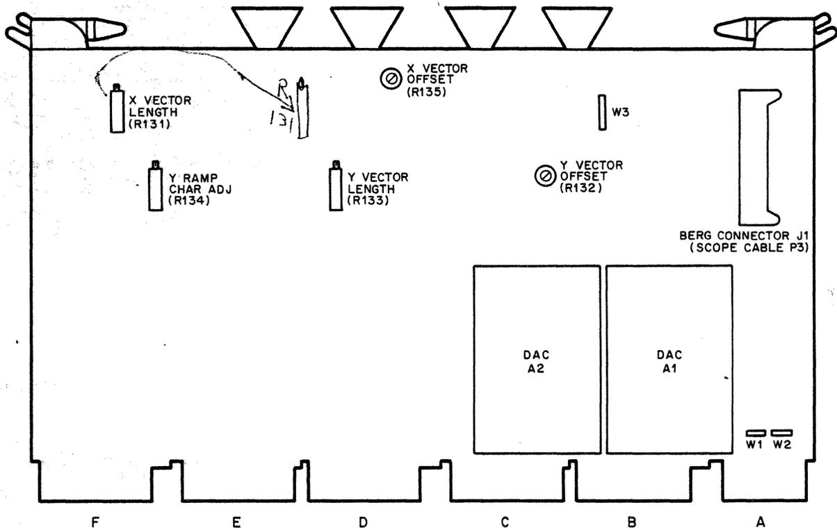
Figure 4-1 Adjustment Locations, A320 Module
