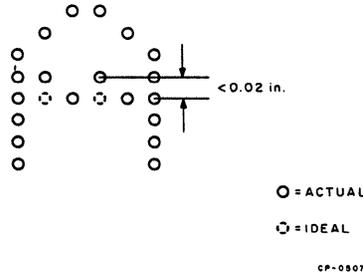
23. Two adjustments, R9 on the M7013 module and R134 on the A320 module, control character display. Their function is described in Paragraph 4.2.5.1.
