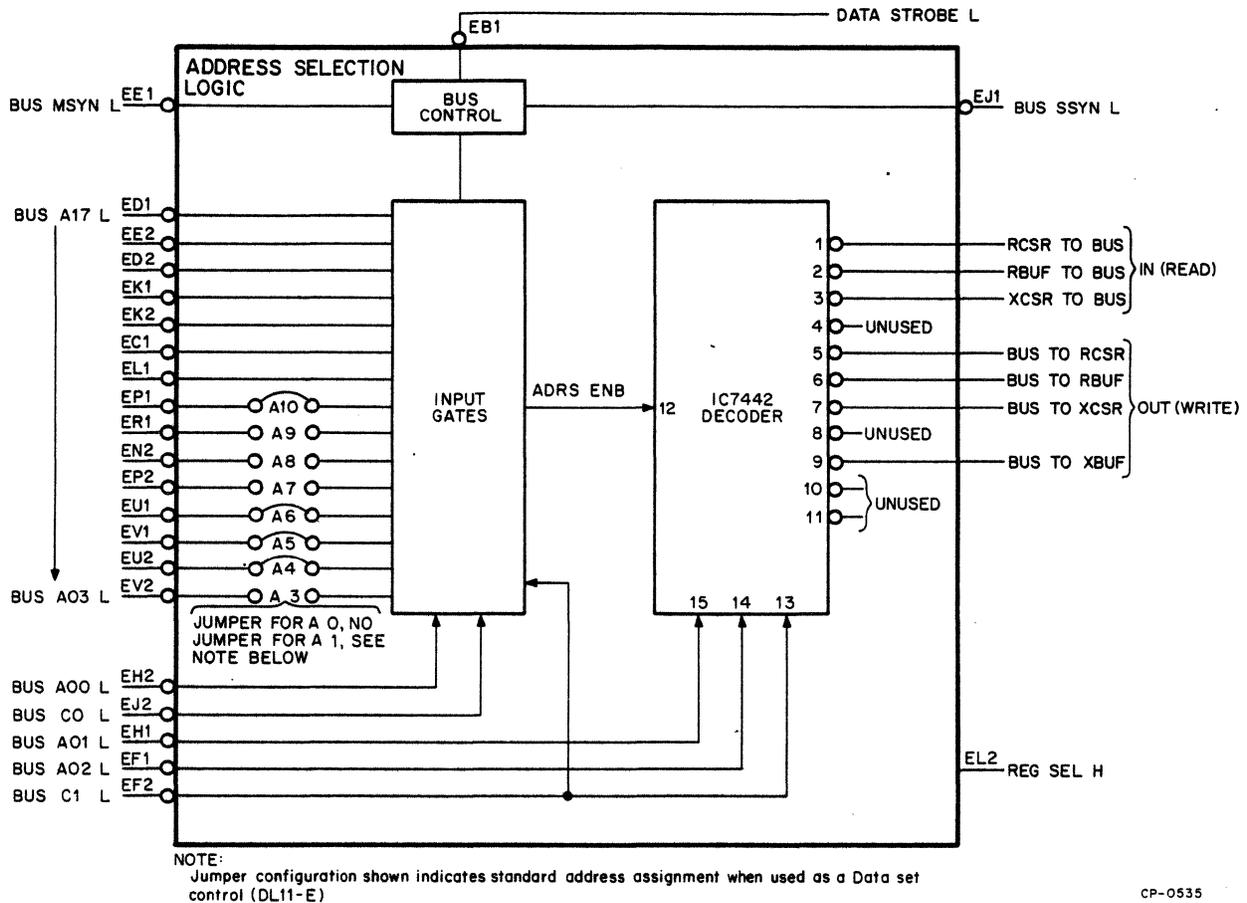
Figure 3-52 Address Selection Logic, Simplified Diagram
