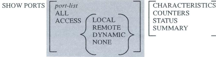
*port-list* Displays information about the specified port(s) only. You can specify from 1 to 128 (1 to 16 for DECserver 510 hardware) individual ports separated by commas, a range of ports connected by a hyphen, or a combination of both (for example, 2,5-20,40-64,32). If you do not specify a port list, information is displayed for your port.
