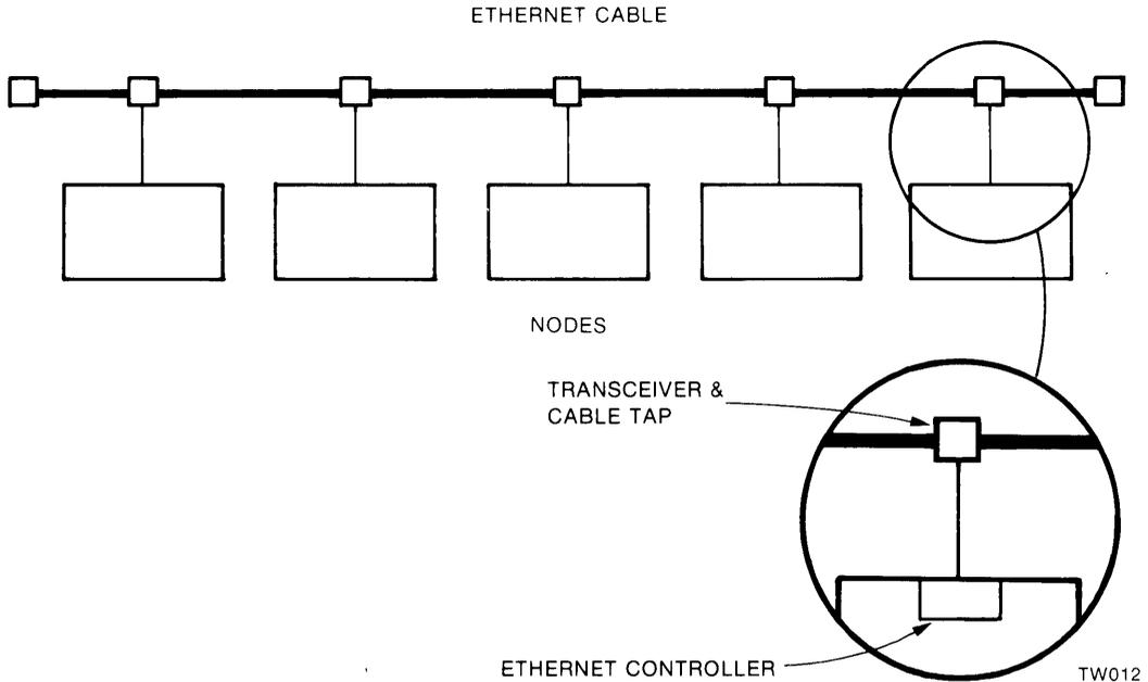
**Figure 1-5: Example of an Ethernet Local Area Network Configuration**
