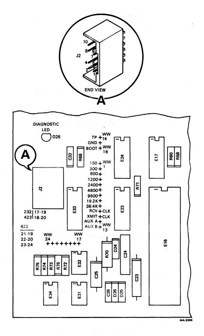
Figure 4-20 Interface Selection Jumper Pin Locations
