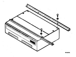
Figure 4-2 Installing Support Brackets
