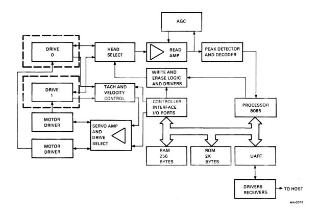
Figure 1-3 TU58 Block Diagram
