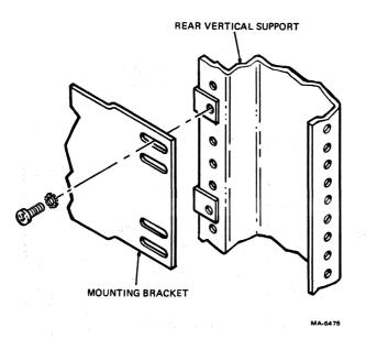
Figure 4-6 Rear Vertical Support U-Nut Retainers
