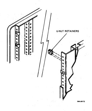
Figure 4-4 Front Vertical Rail U-Nut Retainers
