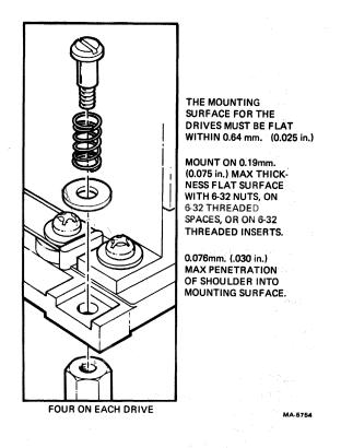
Figure 4-18 TU58 Drive Mounting Hardware
