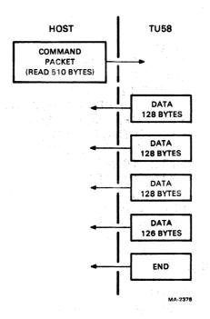
Figure 3-1 Read Command Packet Exchange
