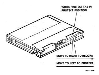
Figure 2-4 Write Protect Tab
