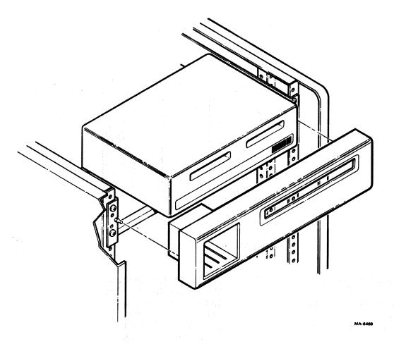
Figure 4-8 Installing the Bezel
