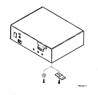
Figure 4-13 Mounting the TU58-EA and -EB
