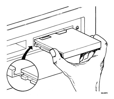
Figure 2-3 Cartridge Loading
