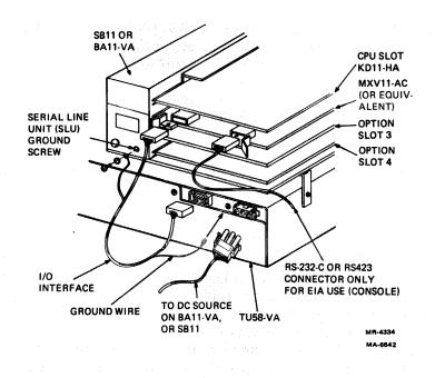
Figure 4-15 Interfacing the TU58-VA
