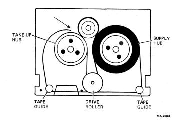
Figure D-5 Threading the Plastic-Base Cartridge
