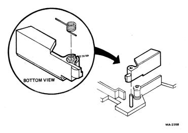
Figure D-3 Head Gate and Spring
