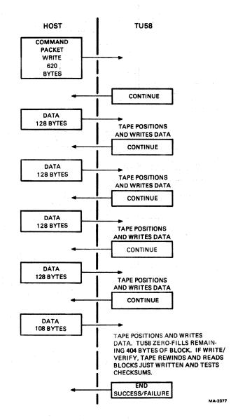
Figure 3-2 RSP Write Transaction
