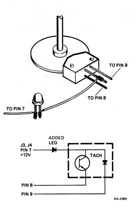
Figure 5-1 Installation of Run Indicator
