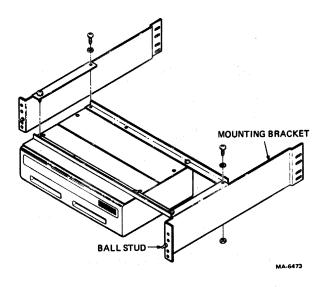
Figure 4-3 Installing Mounting Brackets
