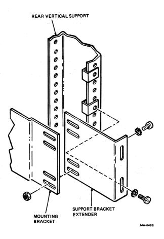
Figure 4-7 Fastening Support Bracket Extenders
