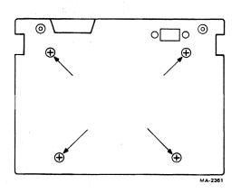
Figure D-1 Baseplate Screw Locations
