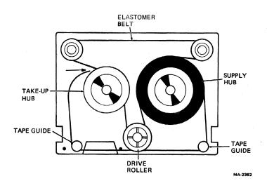
Figure D-2 Threading the Metal-Base Cartridge
