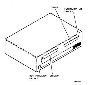
Figure 2-2 TU58-EA, -EB, and -VA Front Panel
