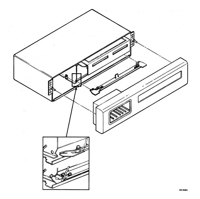
Figure 4-12 Installing Cage and Retainer Bar
