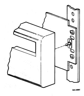
Figure 4-9 Bezel and Ball Stud
