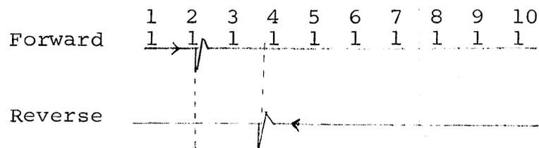
When the tape is moving forward, the sync pulse is generated when the flag for the second data flag is raised.
