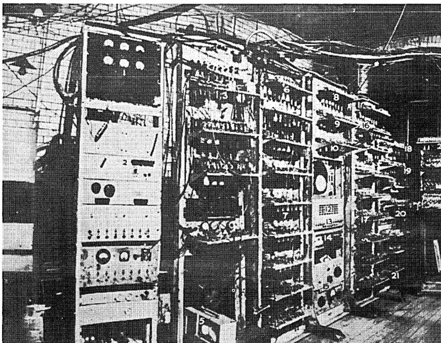
Fig. 7.1 Part of the Manchester University Mark I computer as extended in 1949. The prototype, operational in June 1948, occupied the centre six racks in the photograph and is believed to be the world's first stored-program computer. The Mark I was built out of war-surplus components with an enthusiasm that left little time for tidiness! Incredibly, it worked for long enough at a time for some useful computation to be carried out. It also contained some novel ideas, for example index registers.
