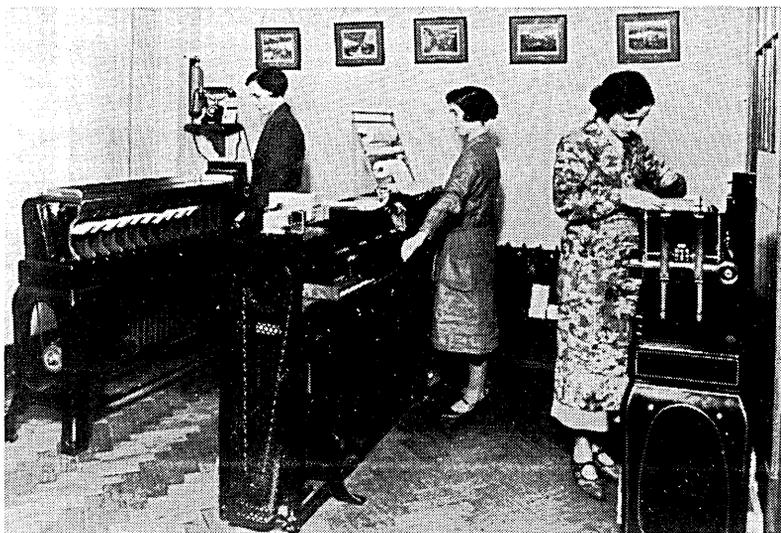
Fig. 2.2 Punched card equipment of the 1930s. Tabulators and sorters of the type shown above were widely used in commerce and administration. Note the Queen Anne legs!
