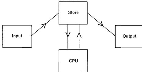
The *output* unit could be an electric typewriter, or a *lineprinter*. Alternatively, a *visual display unit* (VDU) could be used where a direct presentation of results is required.
