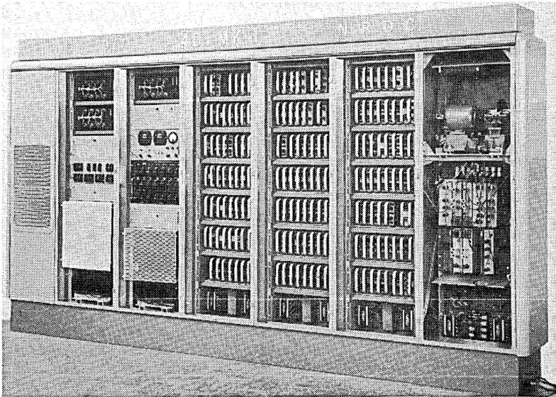
Fig. 11.3 The Elliott 401 computer (1953), built under a National Research Development Corporation contract to promote modular circuit techniques. The resulting plug-in packages here give the appearance of books in a book-case. The magnetic disc store and its motor may be seen in the upper right compartment in the photograph. The 401 was the progenitor of a family of successful Elliott and Ferranti modular computers.
