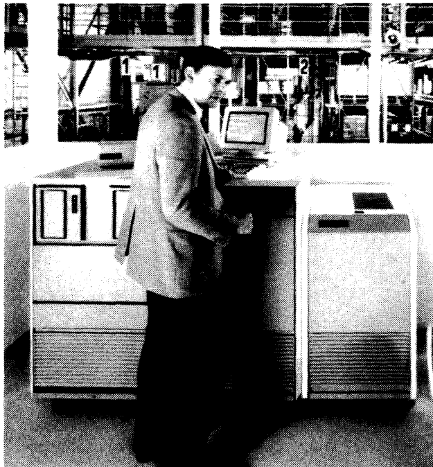
The Model 30 of the DPS 7000 range is configured with eight 500-megabyte mass storage units, a 900 lines-per-minute printer, and a 1600/6250 bits-per-inch magnetic tape subsystem.
