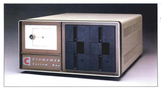
The Z-80A based System One is a desktop computer which is ideal for users who need bus structured expandability in an affordable small computer. The availability of a large base of software written for the Z-80A processor and the ability to handle multiple jobs and multiple users, make the System One an effective solution to a wide range of personal and business applications.
