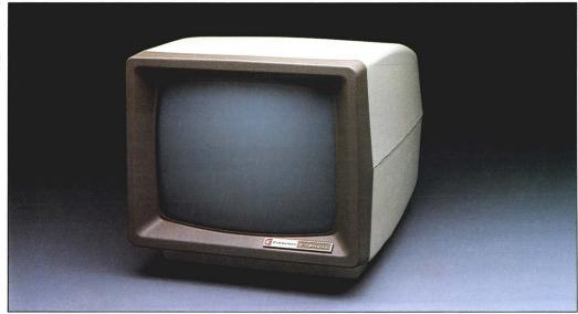
The Model C-1 video display is a high-resolution 12" CRT which can be used for professional quality displays and graphics presentations. The Model C-1 uses the P-31 green phosphor standard and has a display capability of 80 columns and 25 lines.
