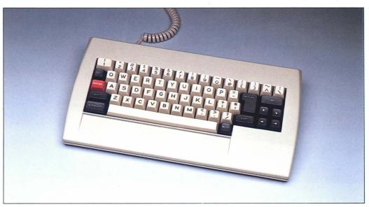
The Model CKBA is an intelligent keyboard which is designed to accommodate all of the special functions that are assigned to separate function keys on more expensive keyboards. The CKBA includes a standard four-wire coiled modular telephone cable which connects to the Model C-1 CRT terminal or the Model C-10 Personal Computer.
