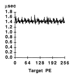
FIGURE 2. Measured inter-node latency as a function of node number.
