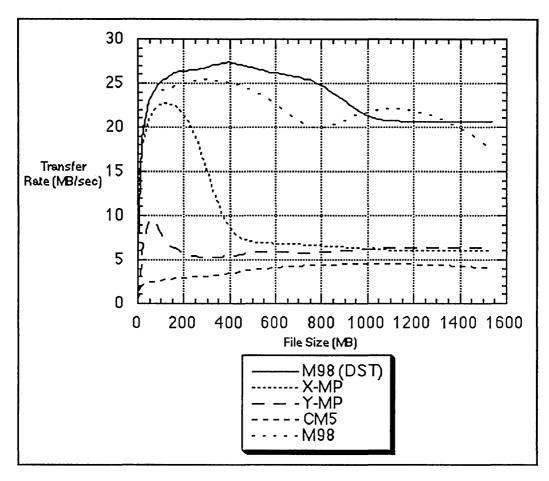
Figure 4. Transfer rates for writing data from the HPDS client to the Disk Array.
