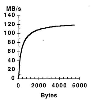
FIGURE 4. Internode communication rate as a function of message size.
