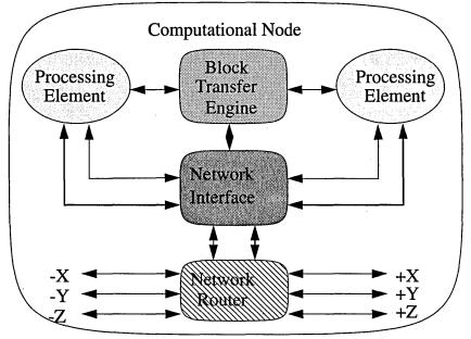
Figure 3: Computational node of Cray T3D.
