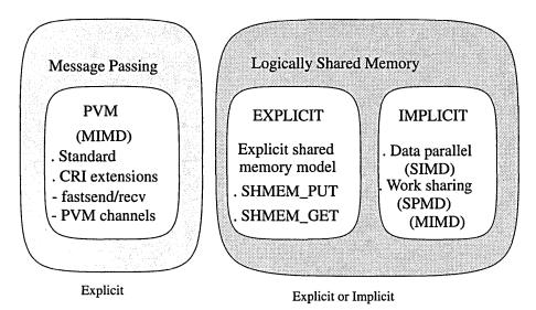
Figure 6: CRAFT programming model available on Cray T3D.
