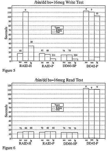
hardware, although sm cache degrades RAID-H and RAID-P performance by 10%.
