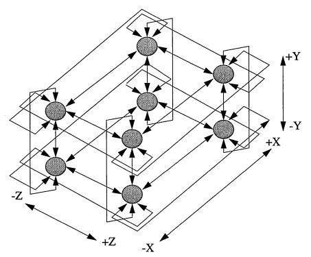
Figure 4: Interconnect topology for Cray T3D.
