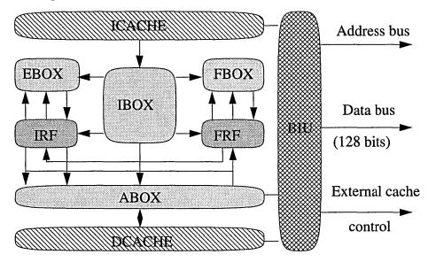
Figure 2: Block diagram of DECchip 21064 Alpha Microprocessor.
