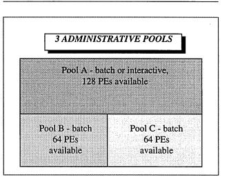
As applications are assigned a partition and downloaded from the Cray PVP front-end machine to the Cray T3D system, sharing will occur. (See figure 1.)
