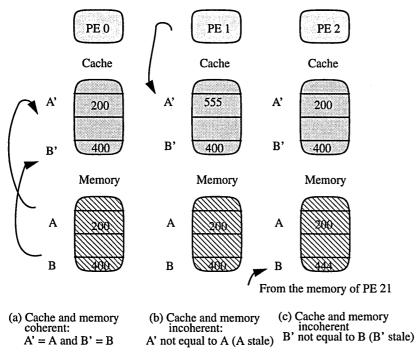
Figure 7: Cache coherency and invalidation of data cache.
