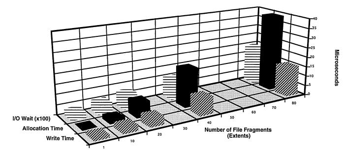
Figure 1. Effect of Number of File Fragmentation on Write, Allocation and I/O Wait Times
