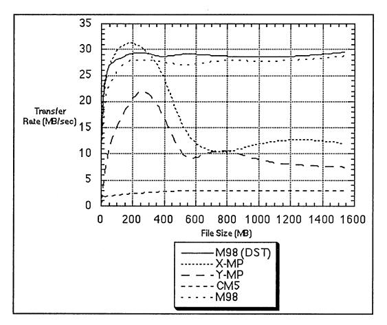
Figure 3. Transfer rates for reading data from the disk array onto the HPDS client.
