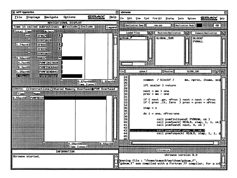
Figure 2: MPP Apprentice tool working cooperatively with Xbrowse
