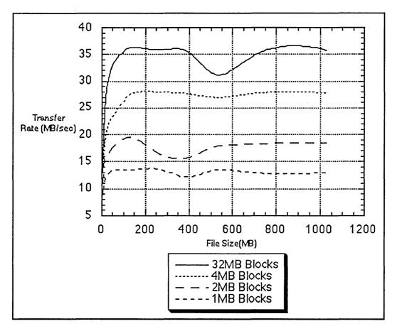
Figure 5. Transfer rates for reading data from the disk array to the Cray M98.
