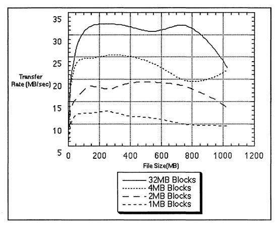
Figure 6. Transfer rates for writing from the Cray M98 to the disk array.
