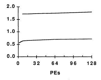
FIGURE 3. Synchronization time as a function of number of PEs. The lower curve is for synchronization without deadlock detection. The upper curve is for synchronization with deadlock detection.
