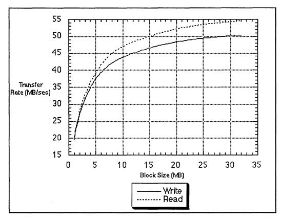
Figure 2. Raw transfers using a HIPPI tester without HPDS overhead.
