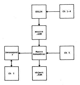
Figure 4. Overview of Macro Assembler Operation
