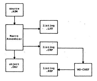
Figure 6. Files That Macro Assembler Produces
