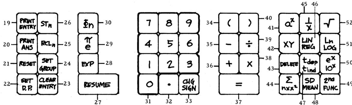
19. PRINT ENTRY causes the contents of the entry register to be printed with the number of places indicated by the decimal point setting, but without rounding. Digits beyond the number of places called for will simply be ignored.
