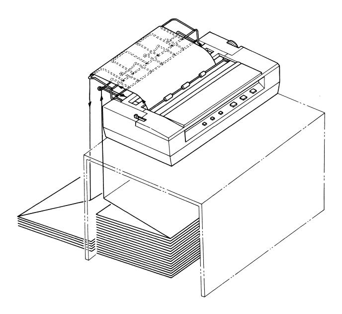
Fig. 12 Example of Paper Guide Separator Application
