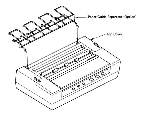
Fig. 11 Mounting the Paper Guide Separator
