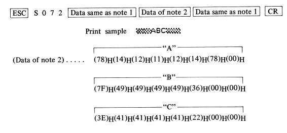
(EX. 2) Vertical Line Print Close the DIP switch (SW2-8) to select the single directional printing, eliminating the divergence in the line.
