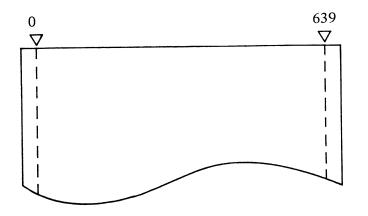
(c) Dot base addressing is done using relative addresses with the left margin set position as 0.
