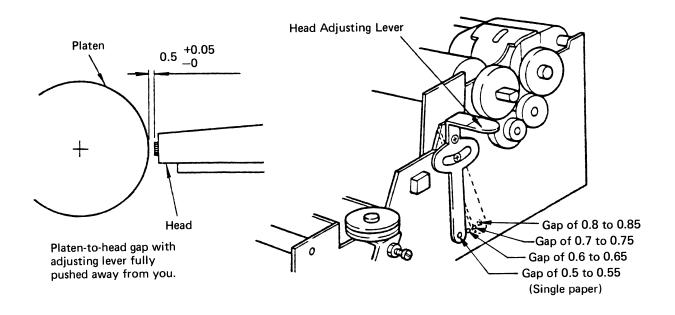
Fig. 13 Gap Adjustment between Dot Head and Platen
