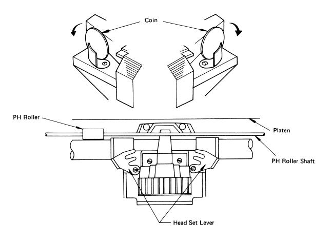
Fig. 28 Head Removal
