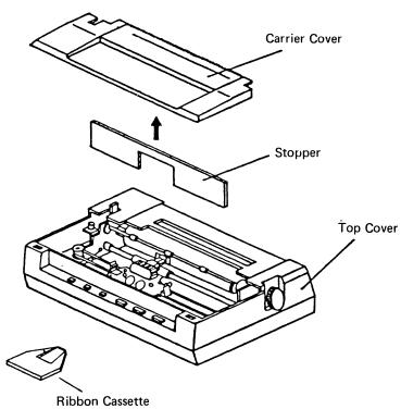
5. Remove the carrier cover from the top cover. Then remove the stopper that is provided to retain the head. (See Fig. 3.)
