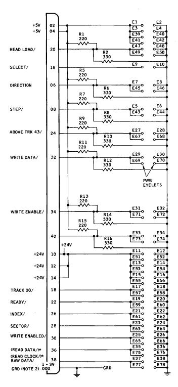
() \*USED WITH SINGLE DENSITY RECORDING (FM) NOTES: 1. PART NO. 12084-001 SHOWN; PART NO. 12084-002 DOES NOT HAVE TERMINATING RESISTORS 2. ALL ODD-NUMBERED PINS ON P1 ARE GROUNDED
