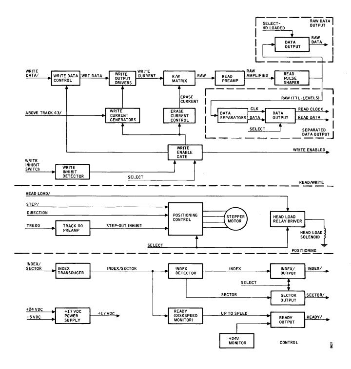
Figure 3-17. Detailed Block Diagram
