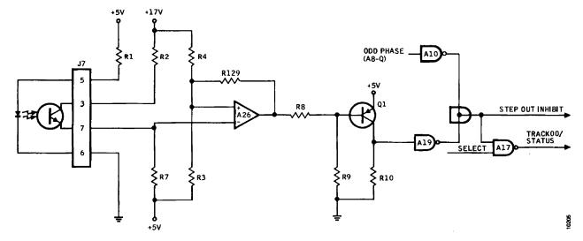
Figure 3-28. Track 00 Detector Circuit
