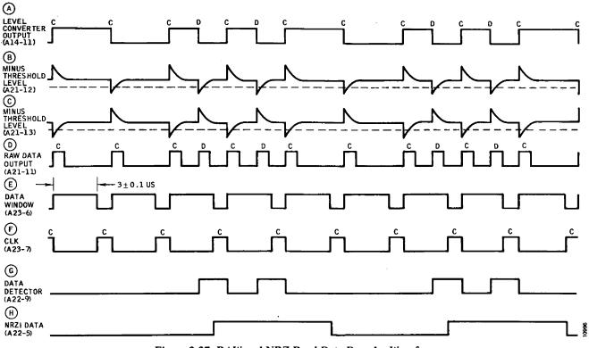
Figure 3-37. RAW and NRZ Read Data Decoder Waveforms
