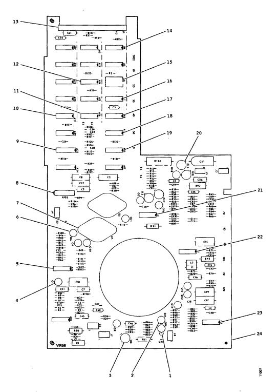
Figure 5-4C. Data and Control Board Assembly, VR58
