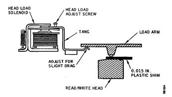
Figure 4-12. Head Load Check and Adjustment
