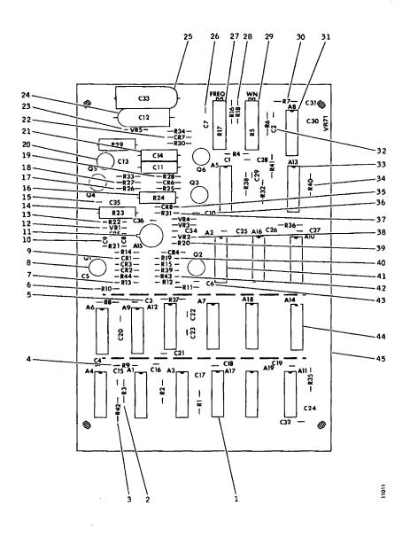
Figure 5-5. Data Decoder with PLO Board Assembly, VR71
