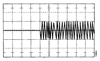
Figure 4-8. Index Pulse with Hard-Sector Option Timing Waveform
