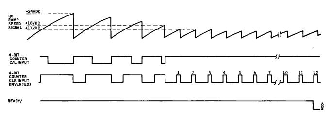
Figure 3-21. Power-On to Ready Transition Period Waveforms
