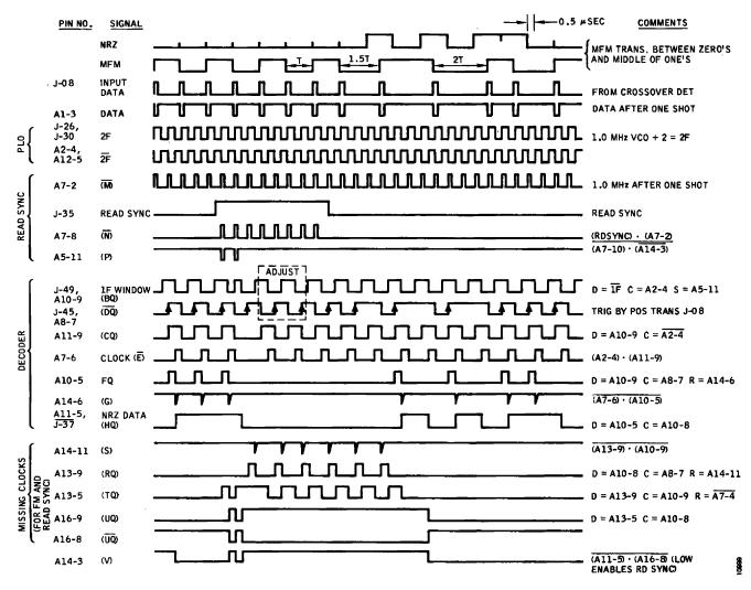
Figure 3-46. Composite MFM Data Decoder Waveforms
