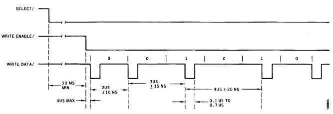
Figure 3-8. MFM Write Data Timing
