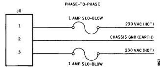
Figure 2-2. Ac Power Cable Wiring
