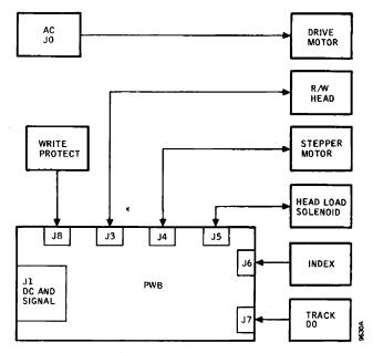
Figure 4-3. Disk Drive Interconnecting Cabling Diagram
