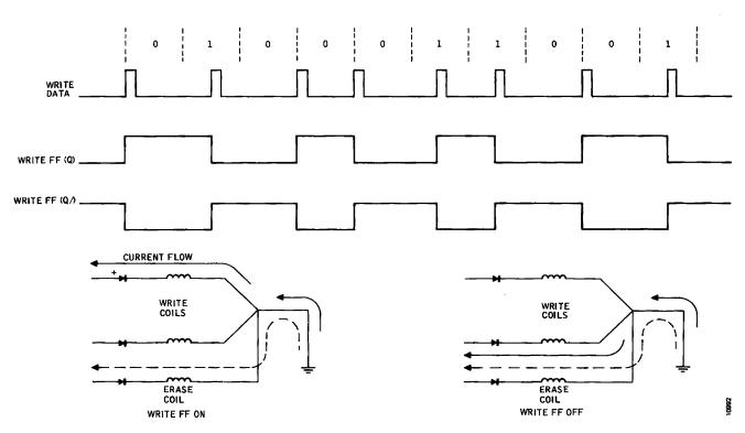
Figure 3-31. MFM Write Control and Write Coil Current Flow
