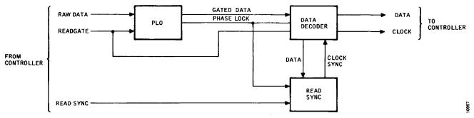
Figure 3-38. Read Decoder with PLO Block Diagram
