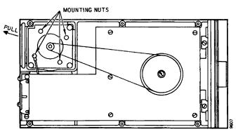
Figure 4-5. Drive Belt Checks and Adjustments
