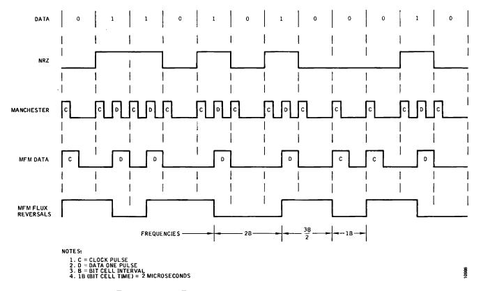
Figure 3-2. Code Format Comparisons and MFM Characteristics
