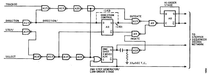
Figure 3-25. Stepper Motor Position Control Simplified Logic Diagram
