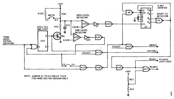
Figure 3-18. Index Pulse Detection on Speed Monitor, Simplified Logic Diagram
