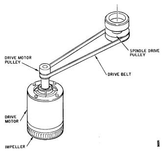
Figure 4-4. Drive System Component Identification
