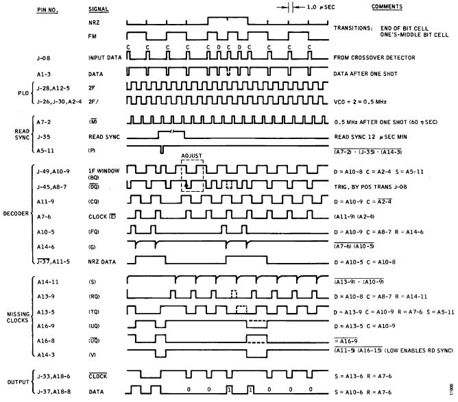
Figure 3-47. Composite Double Frequency Data Decoder Waveforms
