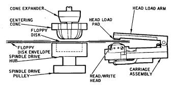
A. CENTERING CONE AND READ/WRITE HEAD UNLOADED
