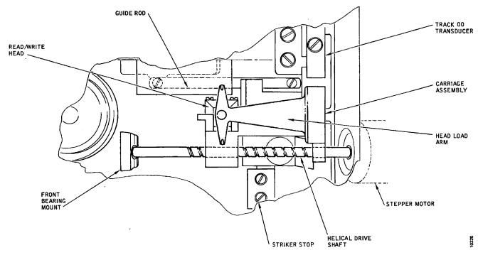
Figure 3-15. Positioning Mechanism
