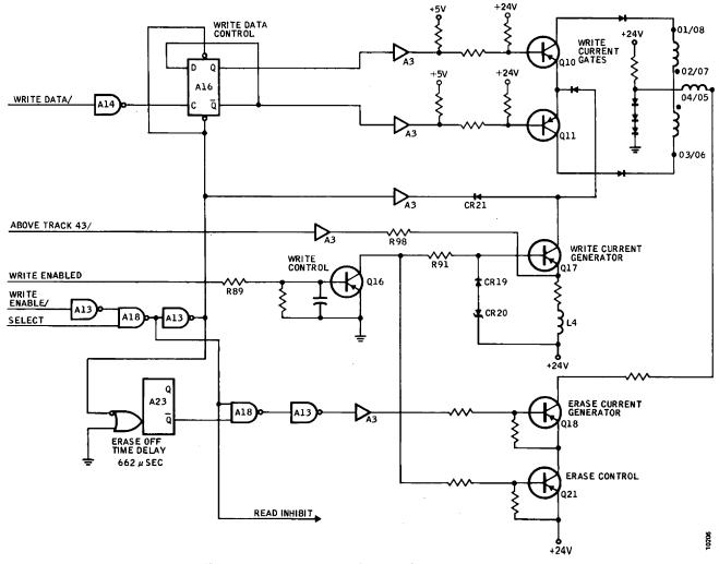
Figure 3-29. Write Channel, Simplified Logic Diagram
