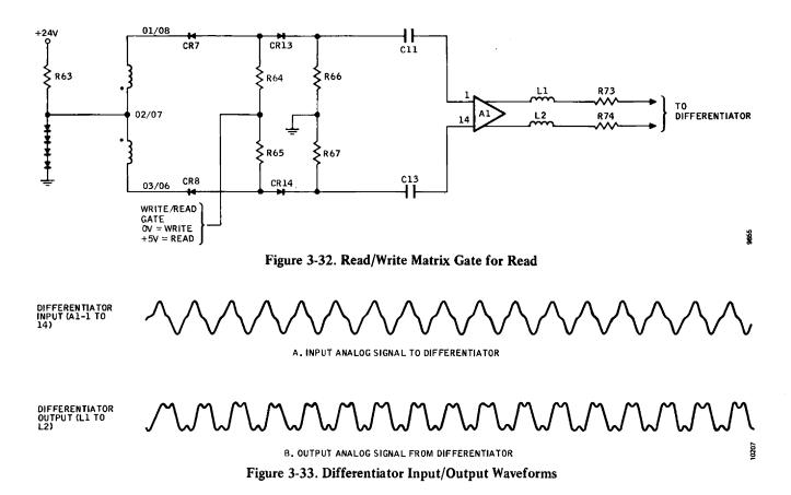
sharpens the rise and fall times. At this time, the analog signal is shaped into a digital signal; each transition represents a flux change sensed by the read/write head. The pattern is then restored to TTL logic levels.
