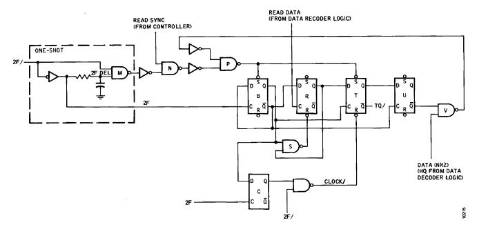
Figure 3-45. Read Data Decoder Sync, Simplified Logic Diagram
