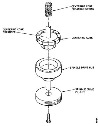
Figure 4-9. Spindle System Component Identification
