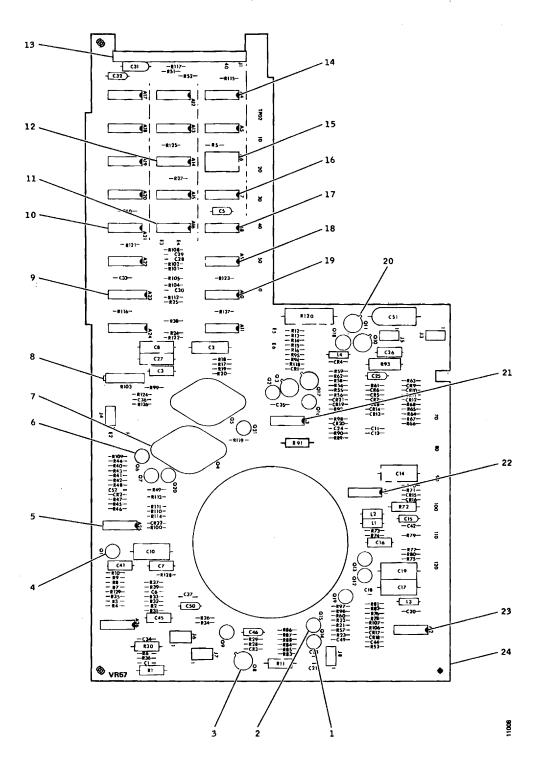
Figure 5-4B. Data and Control Board Assembly, VR57
