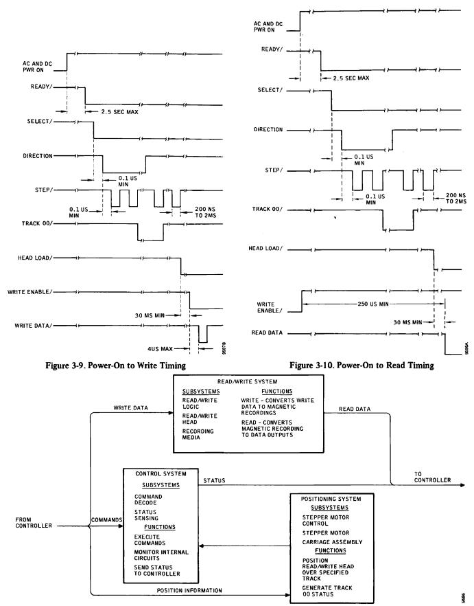
Figure 3-11. Disk Drive General Block Diagram
