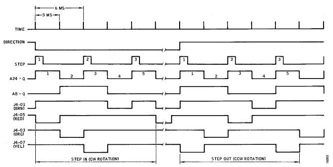
Figure 3-26. Stepper Motor Direction Sequencing
