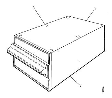
Figure 5-1. Model 140 Series and 142 Disk Drive Unit (Sheet 1 of 2)
