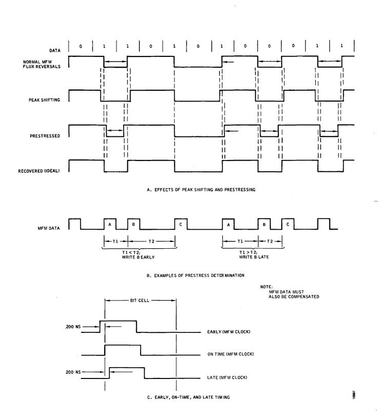
Figure 3-3. Peak Shifting and Precompensation Conditions
