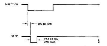
Figure 3-23. Single-Track Positioning Time Waveforms
