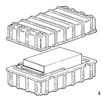
Figure 2-1. Disk Drive Shipping Configuration
