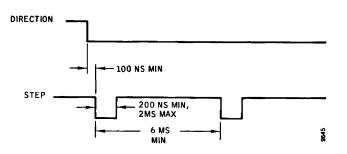
Figure 3-24. Multiple-Track Positioning Time Waveforms
