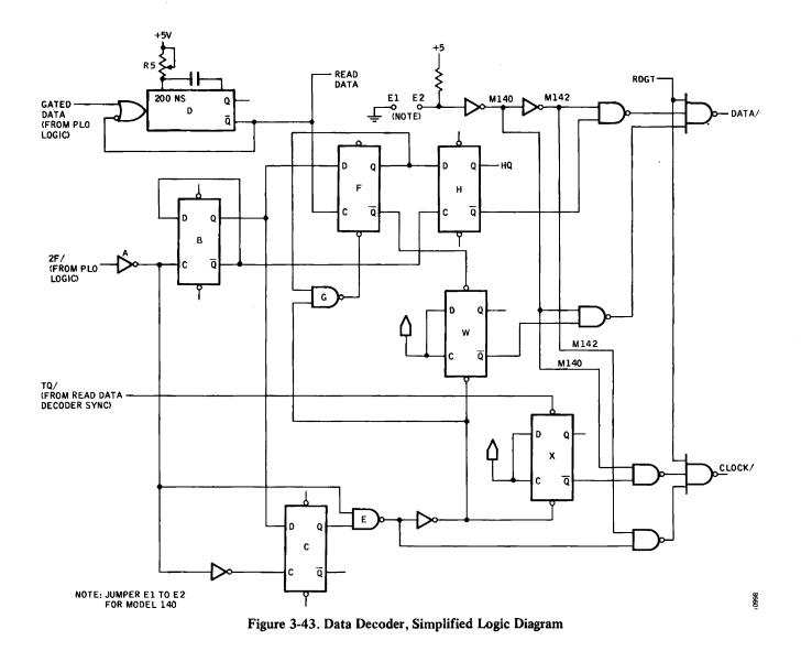
The CLOCK/ output to the controller is developed at gate E by ANDing the Q output of flip-flop C (which is 1F/ shifted 500 nanoseconds late) with 2F to create a 500nanosecond-long pulse whose leading edge is coincident with the beginning of each bit cell time (see Figure 3-44).
