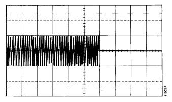
Figure 4-7. Index Pulse Timing Waveform
