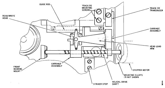
Figure 4-10. Positioning System Component Identification
