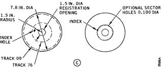
Figure 3-1. Flexible Disk Construction
