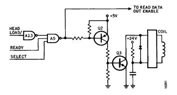
Figure 3-22. Head Load Relay Driver
