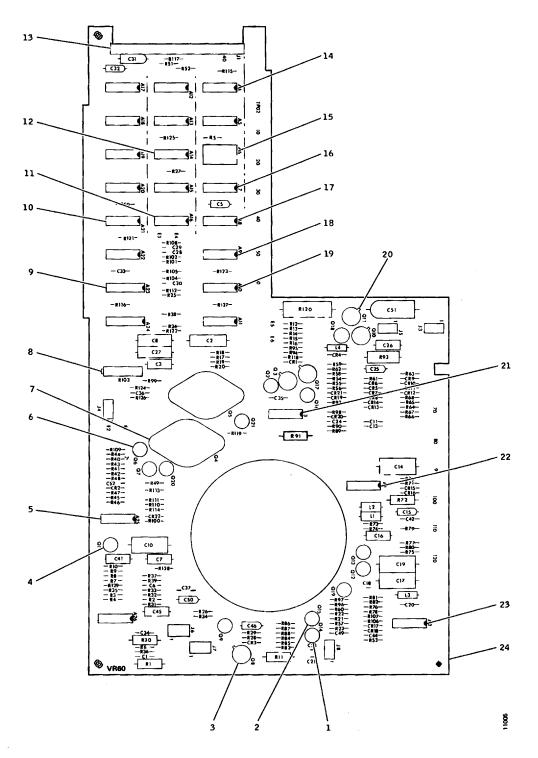
Figure 5-4D. Data and Control Board Assembly, VR60
