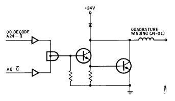
Figure 3-27. Decode and Current Drivers for 00 Code
