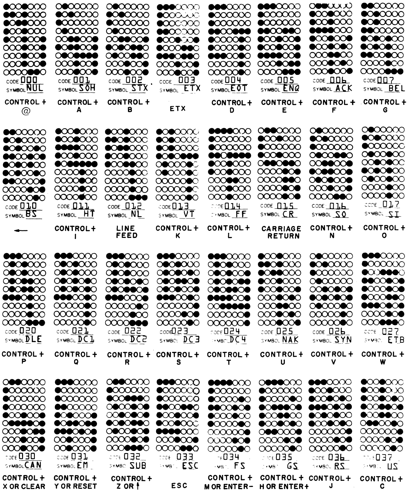
Figure CRT2. Control Code Dot Matrix Formations and Octal Codes*
