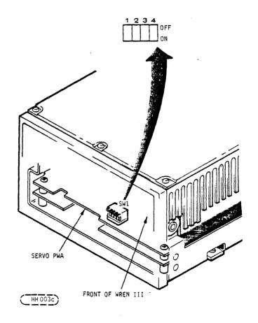
FIGURE 13. CONFIGURATION SWITCH LOCATIONS (See Table 6.)
