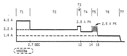
FIGURE 3A. TYPICAL WREN III +12 V CURRENT PROFILE
