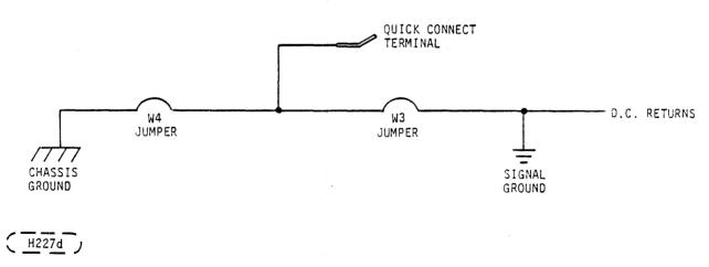
FIGURE 11a. SCHEMATIC DIAGRAM OF W3 AND W4
