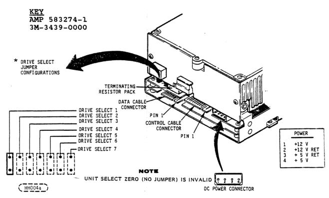
The position of this jumper when drive is shipped is determined by a customer configuration document.
