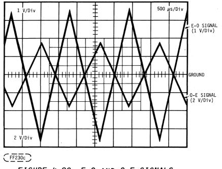
FIGURE 4-28. E-O AND O-E SIGNALS (CDC AND SEAGATE INTERFACES)
