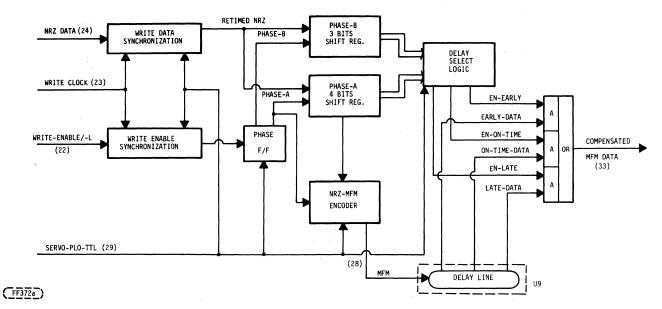
FIGURE 4-30. MFM ENCODER-COMPENSATOR INSIDE THE READ/WRITE LSI (CDC INTERFACE)
