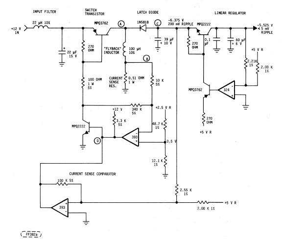
FIGURE 4-41. WREN I DC-DC CONVERTER (CDC AND SEAGATE INTERFACES)
