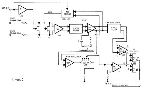
FIGURE 4-33. DATA PWA READ ANALOG FUNCTION (CDC INTERFACE)
