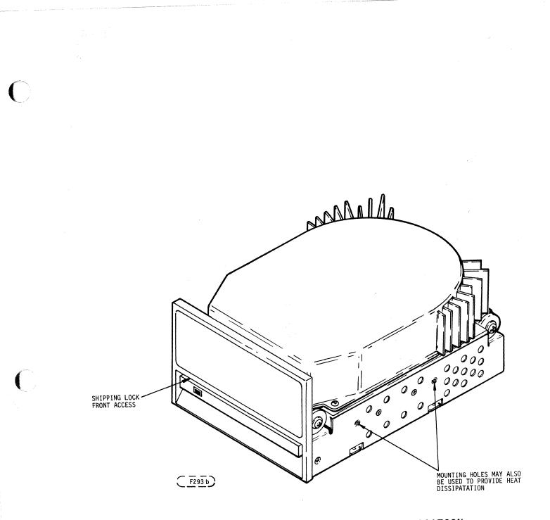
FIGURE 3-3. HEAT SINK MOUNTING HOLE LOCATION
