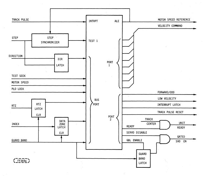
FIGURE 4.5. WREN I MICROCOMPUTER BLOCK DIAGRAM (CDC INTERFACE)
