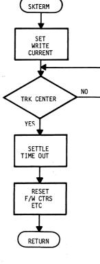
FIGURE 4-20. SEEK TERMINATE (CDC AND SEAGATE INTERFACES)
