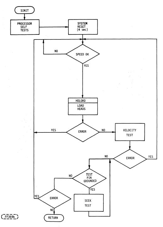
FIGURE 4-13. SYSTEM INITIALIZE (CDC AND SEAGATE INTERFACES)
