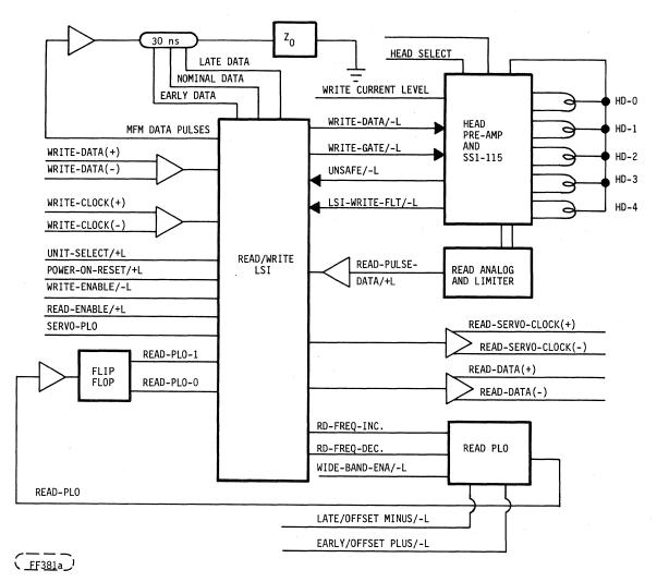
FIGURE 4-29. WREN I DATA BLOCK DIAGRAM (CDC INTERFACE)
