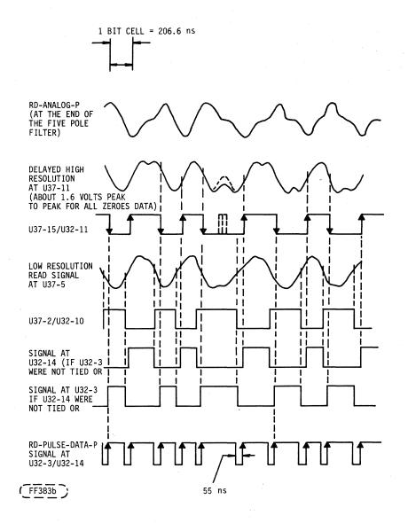
FIGURE 4-34. READ ANALOG TIMING DIAGRAM (CDC INTERFACE)
