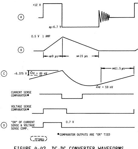
FIGURE 4-42. DC-DC CONVERTER WAVEFORMS (CDC AND SEAGATE INTERFACES)
