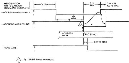
LEADING EDGE INDICATES THE LOCATION OF THE END OF AN ADDRESS MARK.
