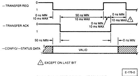
ONE BIT TRANSFER TIMING - FROM DRIVE FIGURE 52
