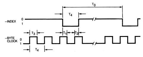
$\begin{array}{l} T_0 = \text{DISK ROTATIONAL PERIOD} = \text{INVERSE OF DISK REVOLUTIONS PER SECOND} \\ T_1 = (0.16) \times (T_4) \text{ TO } (0.25) \times (T_4) \\ T_2 = (0.25) \times (T_4) \text{ TO } (0.33) \times (T_4) \\ T_3 = (0.40) \times (T_4) \text{ TO } (0.6) \times (T_4) \\ T_4 = 8 \text{ TIMES THE REFERENCE CLOCK PERIOD (T)} \\ \text{NOTE: TIMING IS NOMINAL AND MAY VARY DUE TO SPEED VARIATIONS.} \end{array}$
