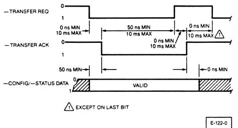
ONE BIT TRANSFER TIMING — FROM DRIVE FIGURE 13
