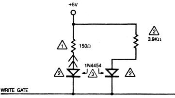
$\bigtriangleup$  part of the terminator resistor pack in the last drive of the daisy chain.
