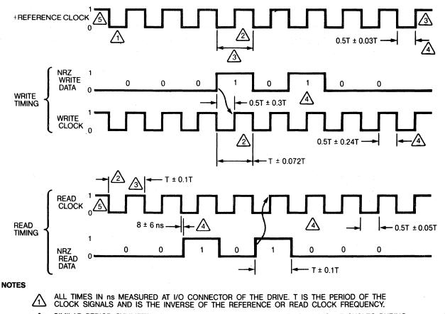
SIMILAR PERIOD SYMMETRY SHALL BE IN ± 4ns BETWEEN ANY TWO ADJACENT CYCLES DURING READING OR WRITING.
