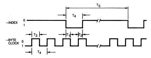
$\begin{array}{l} T_0 = \text{DISK ROTATIONAL PERIOD} = \text{INVERSE OF DISK REVOLUTIONS PER SECOND} \\ T_1 = (0.16) \times (T_4) \text{ TO } (0.25) \times (T_4) \\ T_2 = (0.25) \times (T_4) \text{ TO } (0.33) \times (T_4) \\ T_3 = (0.40) \times (T_4) \text{ TO } (0.6) \times (T_4) \\ T_4 = 8 \text{ TIMES THE REFERENCE CLOCK PERIOD (T)} \\ \end{array}$
