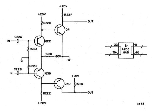
Figure 4-1. Typical Discrete Component Circuit Schematic
