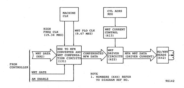
Figure 3-66. Write Circuits Block Diagram
