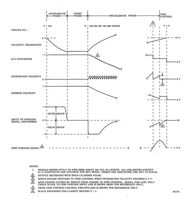
Figure 3-45. Direct Seek Coarse Position Control Signals
