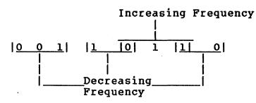
The outputs from the pattern decode logic enable either the Early, Late or Nominal gate (depending on the input frequency) to provide compensated Write data as follows:
