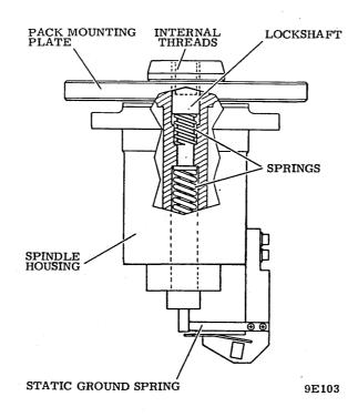
Figure 3-14. Spindle Assembly
