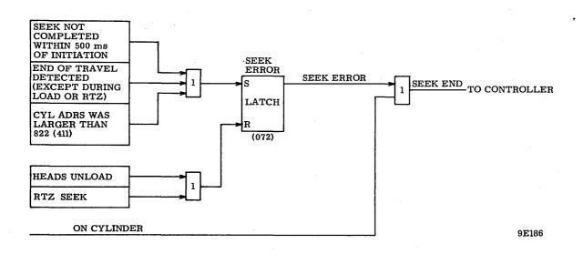
Figure 3-54. Seek End and Seek Error Detection Logic
