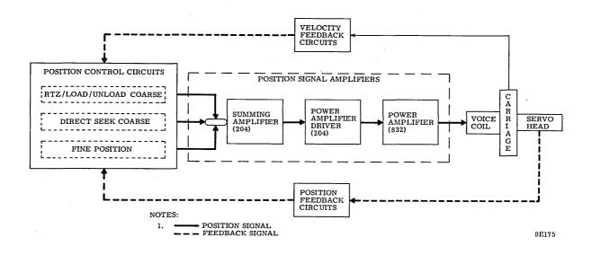
Figure 3-42. Position Signal Amplifier Circuits
