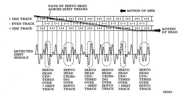
Figure 3-36. Servo Preamp Output
