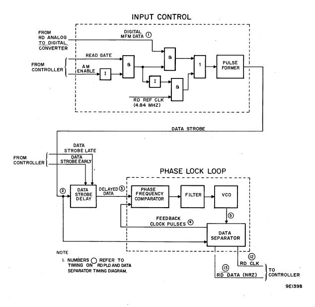
Figure 3-75. Read PLO and Data Separator Circuits
