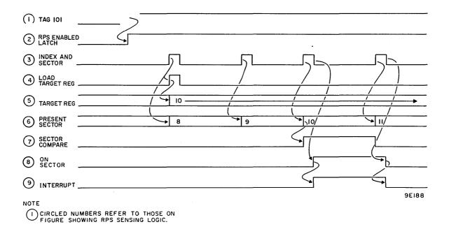
Figure 3-64. Rotational Position Sensing Timing
