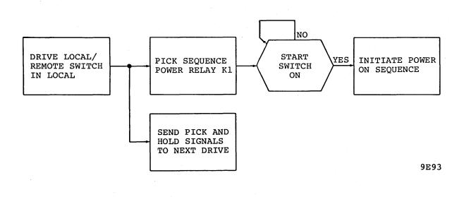
Figure 3-4. Local Mode Power Sequencing
