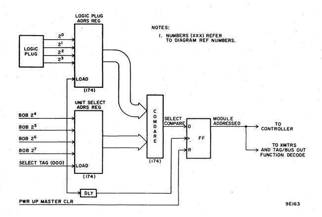
Figure 3-29. Unit Select Logic
