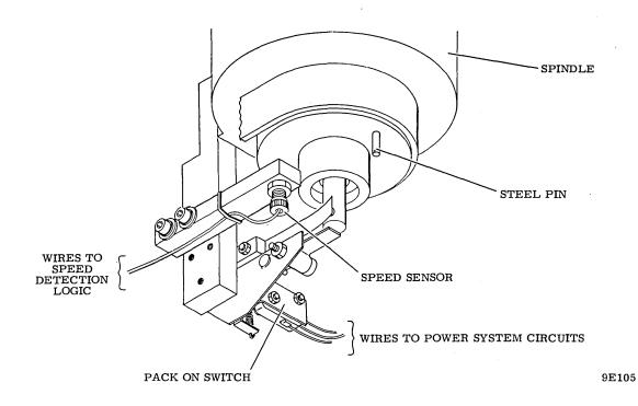
Figure 3-16. Speed Sensor and Pack On Switch Assemblies
