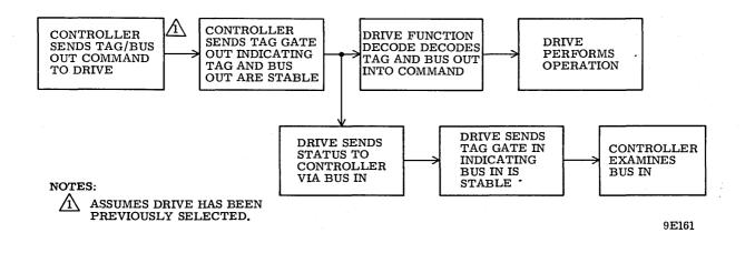
Figure 3-28. Tag/Bus Out Command Sequence Flow Chart
