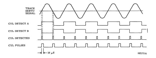
Figure 3-39. Cylinder Pulse Detection
