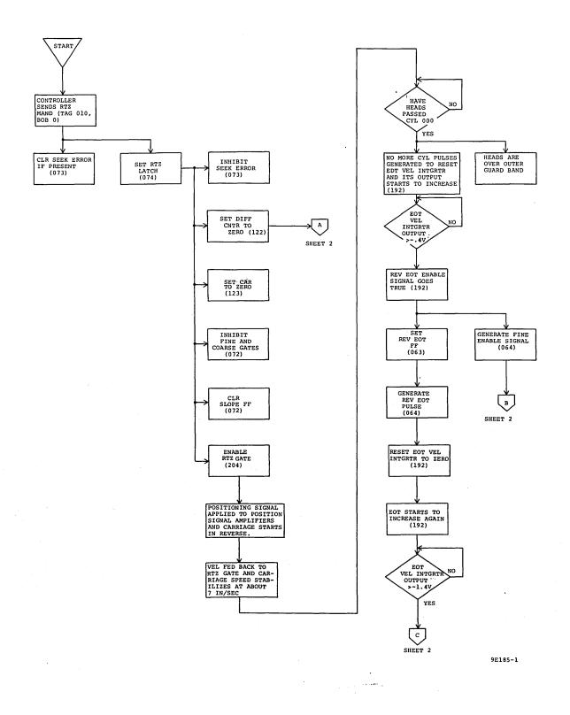
Figure 3-53. Return to Zero Seek Flow Chart (Sheet 1 of 2)
