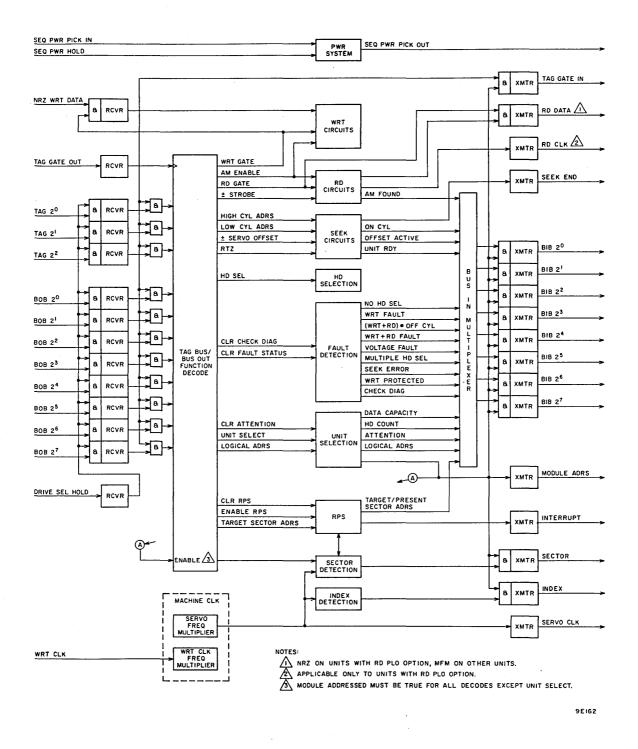
Figure 3-27. I/O Signal Processing Logic
