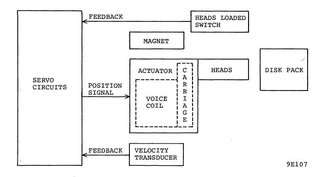
Figure 3-18. Head Positioning Functional Block Diagram
