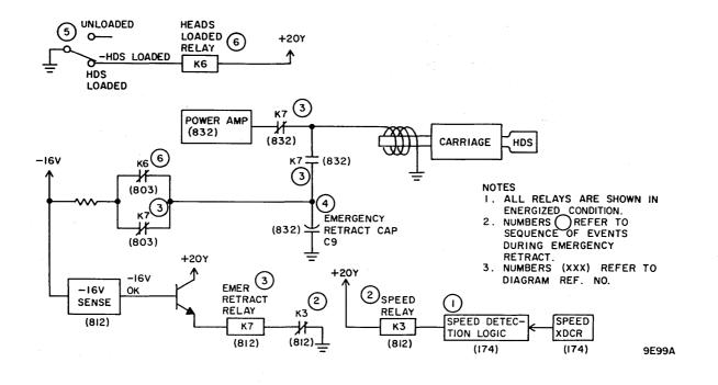
Figure 3-10. Emergency Retract Circuits
