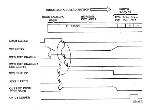
Figure 3-51. Load Seek Timing
