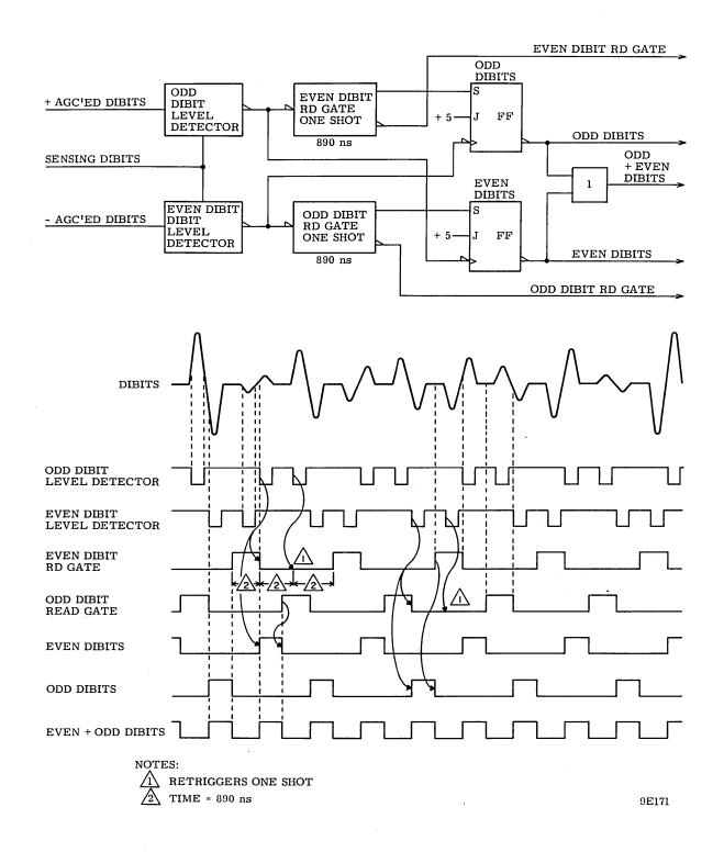
Figure 3-38. Odd/Even Dibits Clock - Logic and Timing
