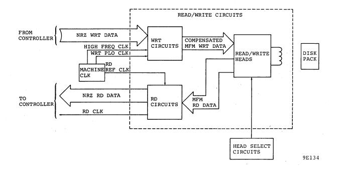
Figure 3-65. Read/Write Circuits Block Diagram
