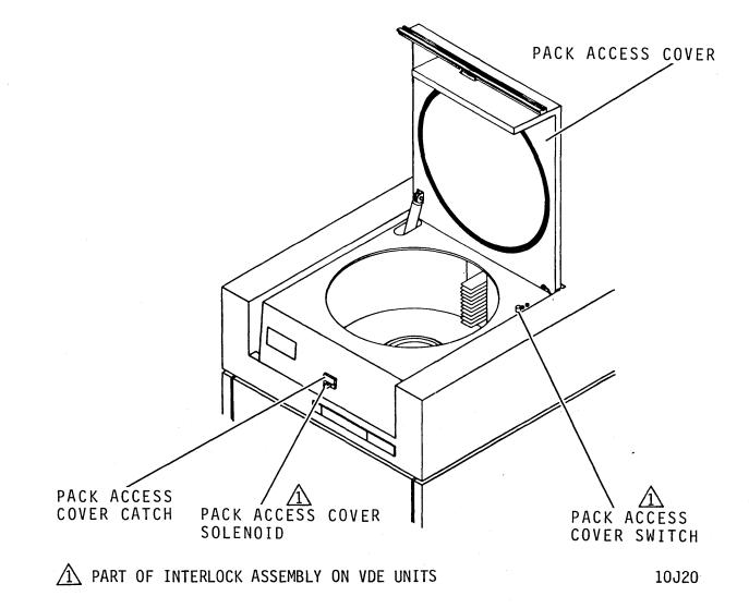
Figure 3-17. Pack Access Cover Switch and Solenoid
