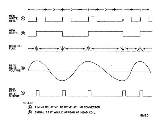
Figure 3-67. MFM Recording - Waveforms and Timing
