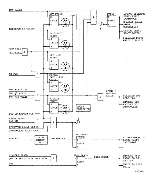
Figure 3-78. Fault and Error Detection Logic
