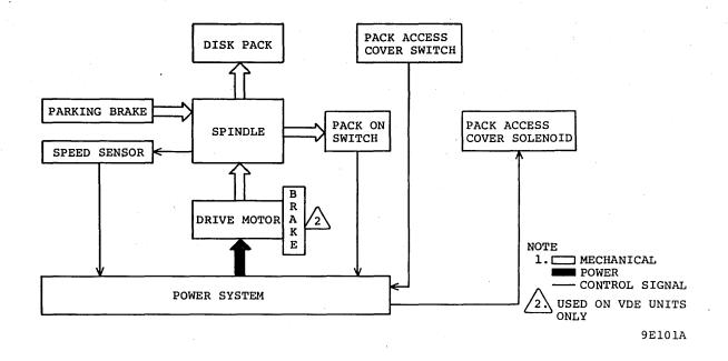
Figure 3-12. Disk Pack Rotation Functional Block Diagram
