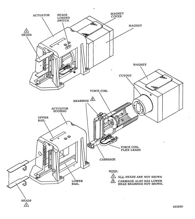
Figure 3-19. Actuator and Magnet Assembly
