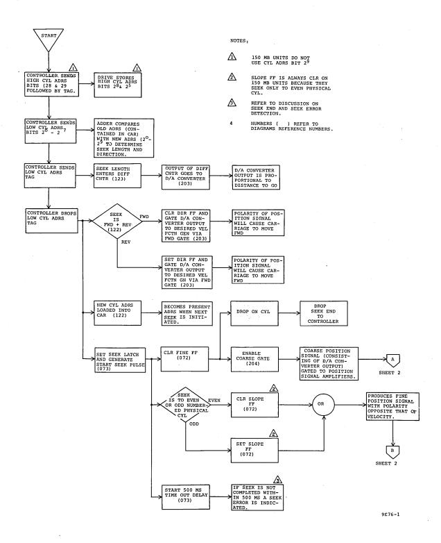
Figure 3-43. Direct Seek Flow Chart (Sheet 1 of 2)
