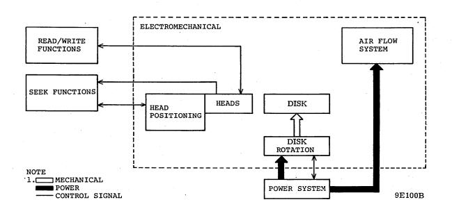
Figure 3-11. Electromechanical Functions Block Diagram
