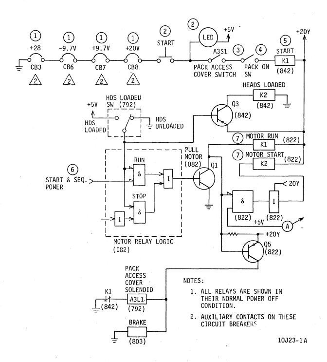
Figure 3-81. Power On Circuit (Sheet 1 of 2)
