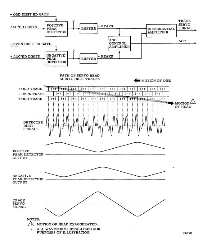
Figure 3-37. Track Servo Amplifier Circuit and Signals
