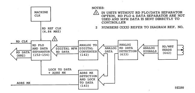
Figure 3-71. Read Circuits Block Diagram
