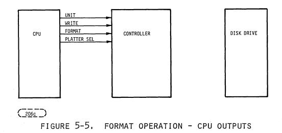
The CPU will send the controller interface signals to select the desired unit (unit).
