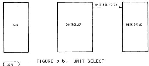
The controller in turn will issue a unit select to the desired disk. This signal will then enable all the input and output lines to and from the selected drive. All other drives will be disabled. The controller can then examine the status lines from the disk drive.
