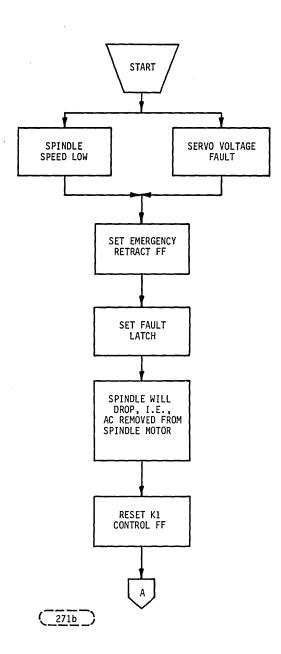
FIGURE 12-6. EMERGENCY RETRACT FLOW CHART (SH 1 OF 2)
