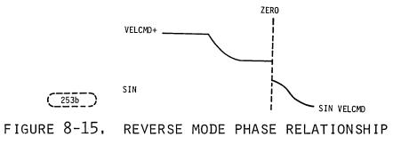
In the reverse direction VELCMD(+) is used for the coarse signal. This positive signal would require sin to be positive during the fine mode, however, sin is positive for some cylinders and negative for others.
