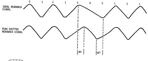
A general rule of thumb is that when the frequency varies, the peaks tend to shift toward the lower frequency.
