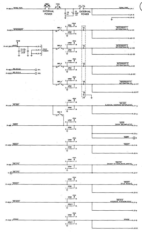
FIGURE 15-3. WINCHESTER I/O BOARD (RACK) (SHEET 7 OF 8)
