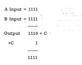
The output would then be 1110 with a carry. The carry bit is added back to the adder input C for a plus 1 which gives us the correct absolute difference of 1111. Plus or minus is not important at this time.
