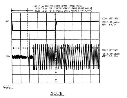
Measurement to be made at the peak of the leading pulse regardless of polarity. Some CE modes produce pulses inverted to pulse shown in Figure.
