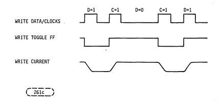
FIGURE 11-4. WRITE CURRENT TIMING
