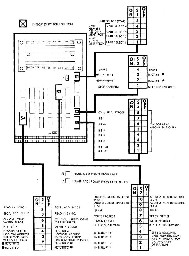
\* WITH HEAD SELECT SWITCHES SET TO UNINVERTED POSITIONS, HEADS ARE NUMBERED 0, 1, 2, 3 FROM TOP TO BOTTOM. WITH HEAD SELECT SWITCHES SET TO INVERTED POSITIONS, HEADS ARE NUMBERED 0, 1, 2, 3 FROM BOTTOM TO TOP. H.S. BIT 2 IS EQUIVALENT TO DISK SELECT. H.S. BIT 1 SELECTS THE TOP OR BOTTOM SURFACE OF THE SELECTED DISK.
