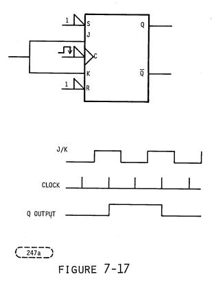
If the J/K Flip Flop has both inputs tied high, then the clock input will be divided by two and made symmetrical.
