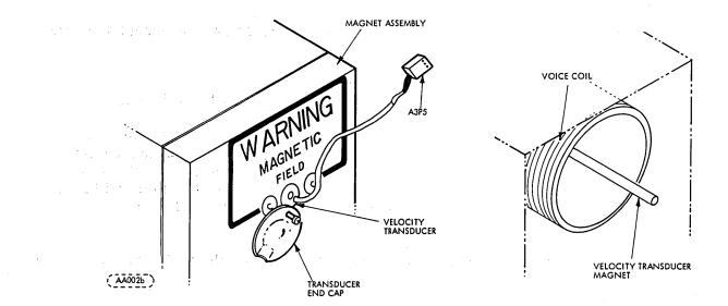
FIGURE LE2-2, VELOCITY TRANSDUCER LOCATION
