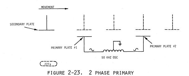
If a second primary plate was added with the opposite polarity signal applied and the secondary plate was again swept from left to right, the signal would be like that shown in Figure 2-24.
