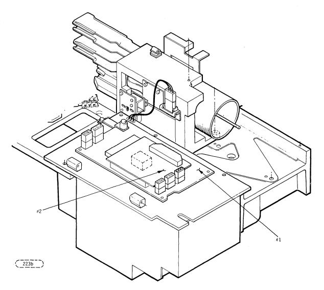
FIGURE 2-7. POWER SUPPLY BOARDS 1 AND 2
