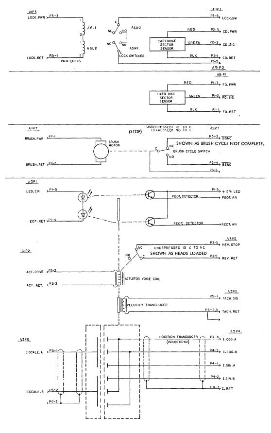
FIGURE 15-18. BASEPLATE ELECTRONICS
