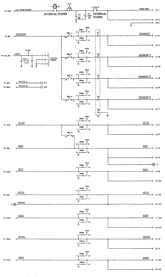
FIGURE 15-2. 3M - I/O BOARD (RACK) (SHEET 7 OF 8)
