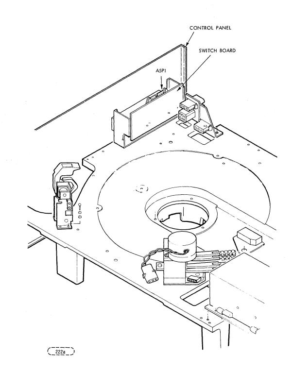
FIGURE 2-6. SWITCH ASSEMBLY
