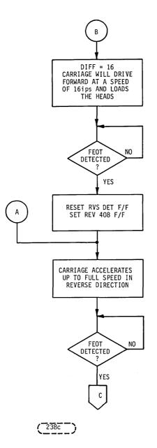
When the first even track count pulse occurs the Rev 408 F/F will reset, resetting the EOT Det F/F which will remove the preset from the counter, allowing it to count. The carriage is at cylinder 408, the counter is at 408 and free to count. Now that both are in sync, the count pulses will continue to count the counter down as the carriage moves toward zero.
