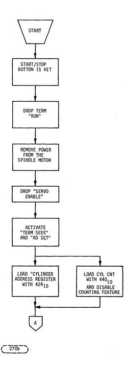
FIGURE 12-4. NORMAL RETRACT FLOW CHART (SH 1 OF 2)
