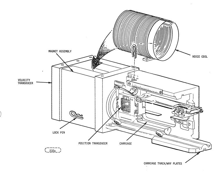
FIGURE 2-12. THE ACTUATOR ASSEMBLY
