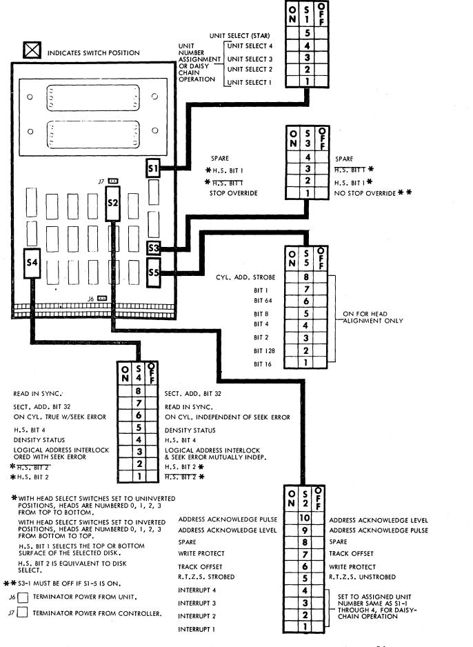
FIGURE 15-3. WINCHESTER I/O BOARD (RACK) (SHEET 1 OF 8)
