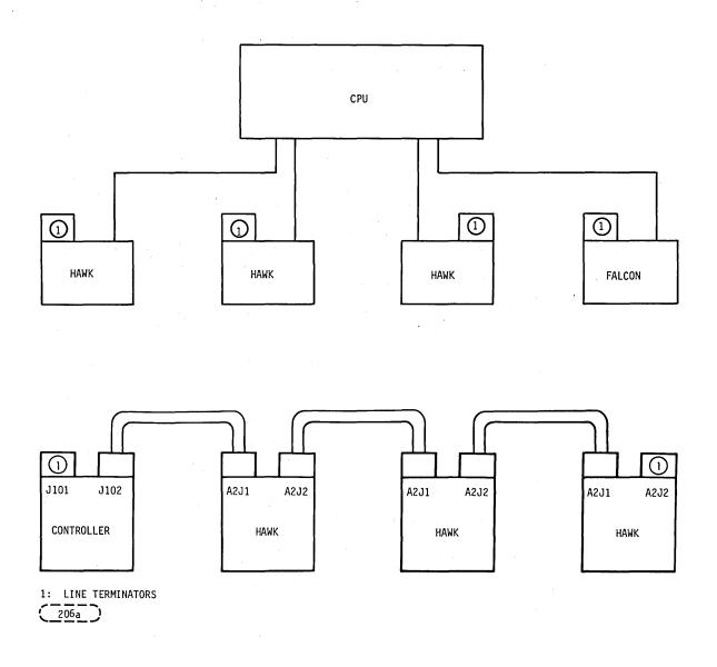
FIGURE 5-3. DISK CONFIGURATIONS
