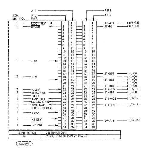
FIGURE 15-13. POWER SUPPLY BOARD NO. 2 (5-22) (SHEET 1 OF 4)
