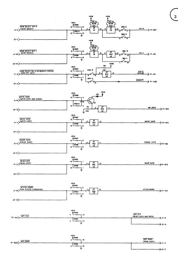
FIGURE 15-3. WINCHESTER I/O BOARD (RACK) (SHEET 6 OF 8)
