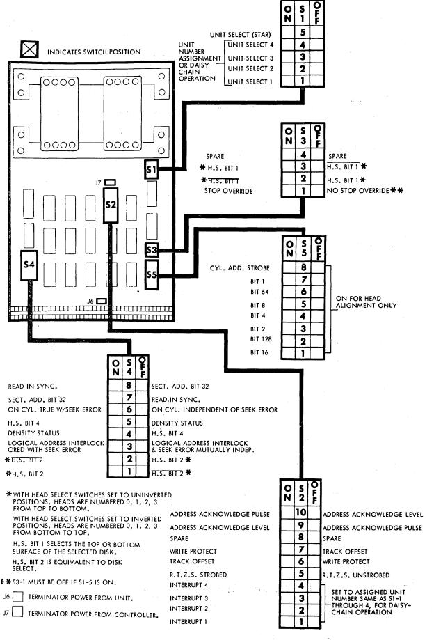
FIGURE 15-4. AMP I/O BOARD (RACK) (SHEET 1 OF 8)
