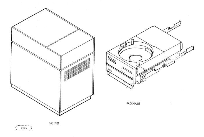
FIGURE 1-1. CABINET AND RACK MOUNT VERSION(9427H)
