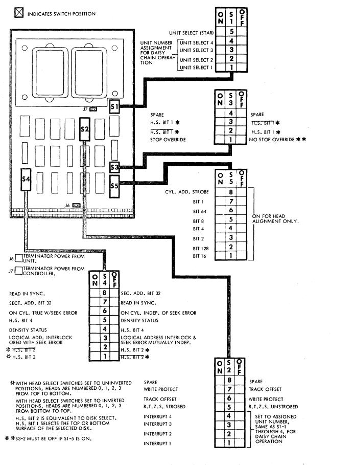
FIGURE 15-5. ELCO I/O BOARD (RACK) (SHEET 1 OF 8)
