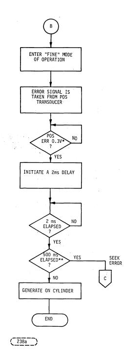
\*Equivalent to 200 micro inches off center of track. \*\*Since address strobe occurred If half a second of time-out occurs before "ON Cyl" is generated, the "Seek Error" latch will be set and the signal "SKER" (seek error) will be transmitted to the controller. The controller may then issue a RTZS command. (Refer RTZS Operation).
