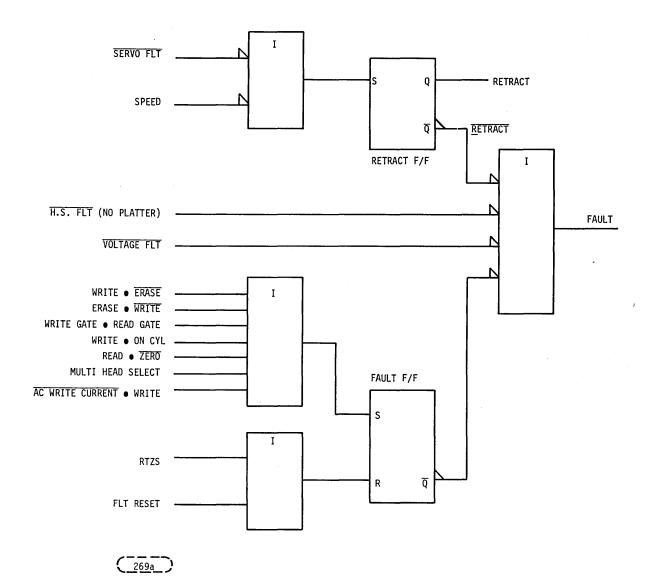
FIGURE 12-1. FAULT LOGIC
