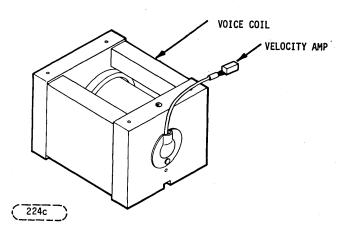
FIGURE 2-19. MAGNET ASSEMBLY
