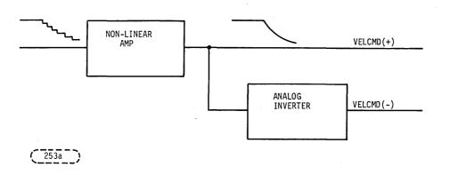
FIGURE 8-12. ANALOG AMP AND INVERTER
