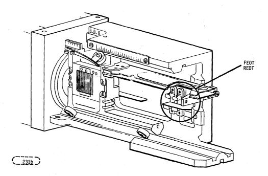
FIGURE 2-28. FEOT & REOT SENSORS
