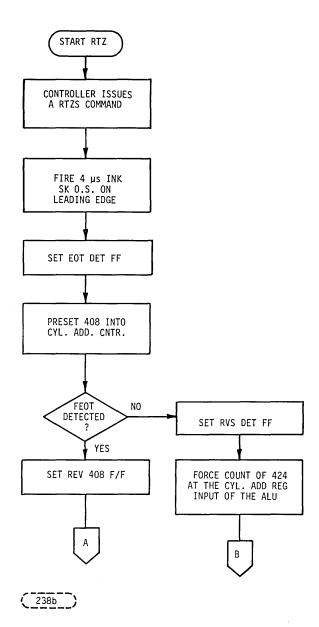
The D/A converter will thus produce a constant error signal in accordance with a difference of 16. The carriage will move forward at an estimated speed of 16 IPS. The heads will load over the disk surface and continue until the forward end of travel is sensed at track position 408. U32/8 will go low when Fwd EOT is sensed.
