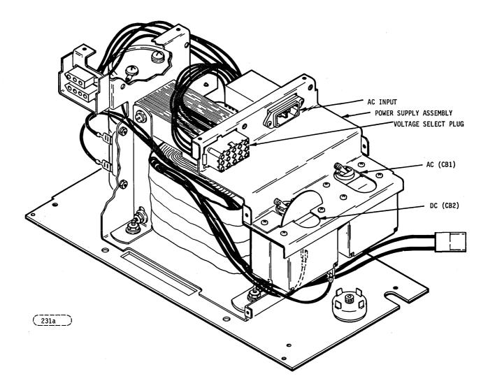
FIGURE 2-30, POWER SUPPLY SWITCHES
