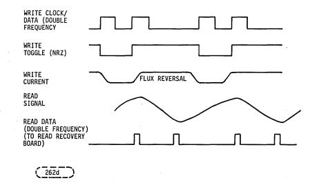
FIGURE 11-9, READ VOLTAGE ILLUSTRATION
