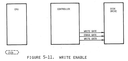
After the Write and Erase logic have been enabled in the drive, (remember that the head is already selected) the controller will send clock pulses from the write clock generator every 400 nsec on the Write Data line.
