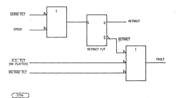
FIGURE 12-3. NON-RESETTABLE FAULTS
