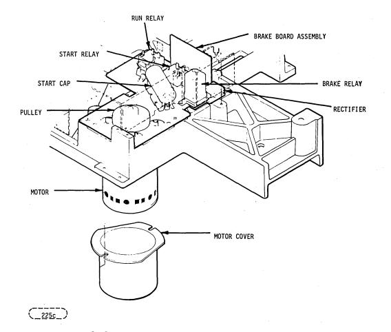
FIGURE 2-9, THE DRIVE MOTOR ASSEMBLY
