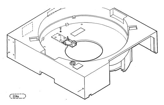
FIGURE 2-16. INDEX/SECTOR TRANSDUCER CARTRIDGE
