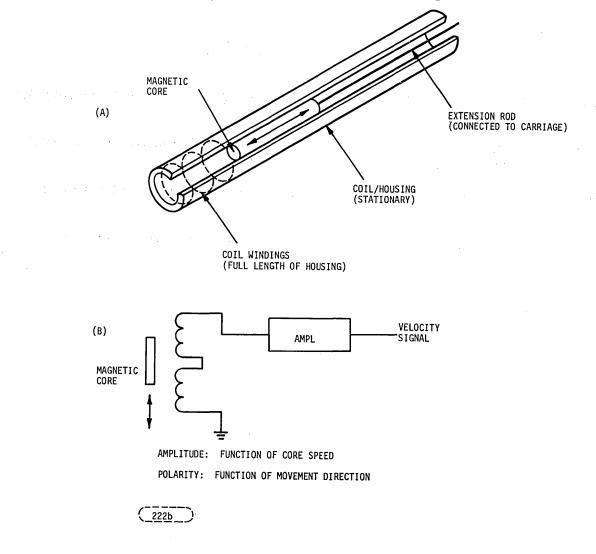
FIGURE 2-18. THE VELOCITY TRANSDUCER
