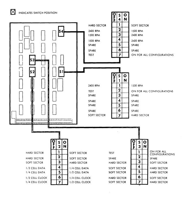
FIGURE 15-9. DATA RECOVERY BOARD (5-18) (SHEET 1 OF 6)
