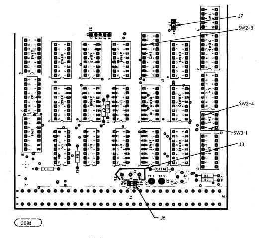
FIGURE 5-2. TERMINATOR CHIPS
