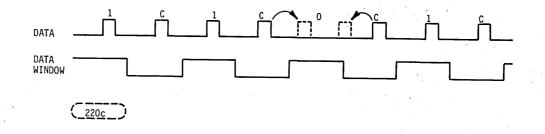
FIGURE 3-15. EFFECT OF PEAK SHIFT-READ ERROR
