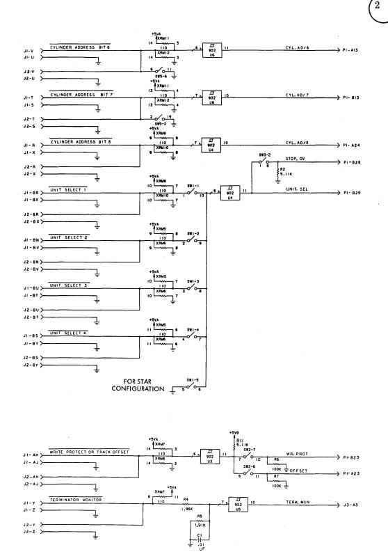
FIGURE 15-5. ELCO I/O BOARD (RACK) (SHEET 5 OF 8)
