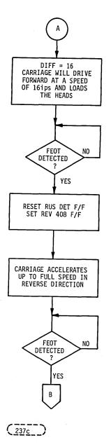
When the first even track count pulse occurs the Rev 408 F/F will reset, resetting the EOT Det F/F which will remove the preset from the counter, allowing it to count. The carriage is at cylinder 408, the counter is at 408 and free to count. Now that both are in sync, the count pulses will continue to count the counter down as the carriage moves toward zero.
