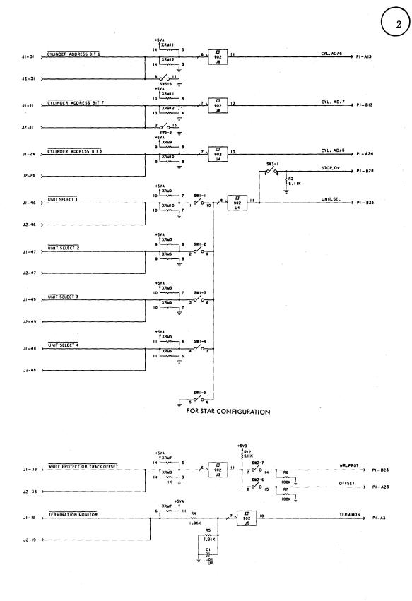
FIGURE 15-2. 3M - I/O BOARD (RACK) (SHEET 5 OF 8)
