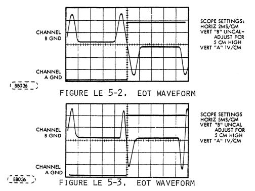
14. Adjust oscilloscope until waveform looks similar to Figure LE 5-2 or LE 5-3. Place crossover of signals A and B in middle of screen and place horizontal sweep time to 10X. Waveform should be similar to Figure LE 5-4 depending on sweep time.
