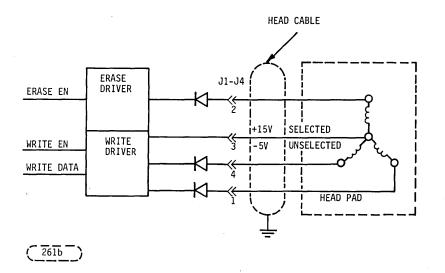
FIGURE 11-2. HEAD CABLE CONNECTIONS
