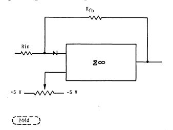
FIGURE 7-50. BIASED OR OFFSET APPLIED
