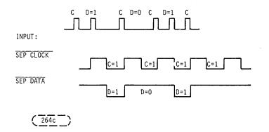
FIGURE 11-14. DATA AND CLOCK SEPARATION
