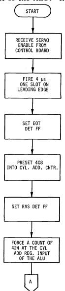
The D/A converter will thus produce a constant error signal in accordance with a difference of 16. The carriage will move forward at an estimated speed of 16 IPS. The heads will load over the disk surface and continue until the forward end of travel is sensed at track position 409. U32/8 will go low when Fwd EOT is sensed. This will reset RUS DET FF and set the Rev 409 F/F. The count of 424 at the ALU will vanish and the ALU will see a difference of 408 as the register is reset at zero.
