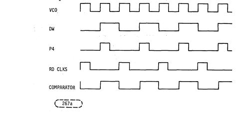
FIGURE 11-23. COMPARATOR OUTPUT - DATA/VCO IN FREQ. SYNC.
