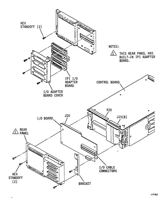
Figure 3-14. I/O Board Replacement (IPI)
