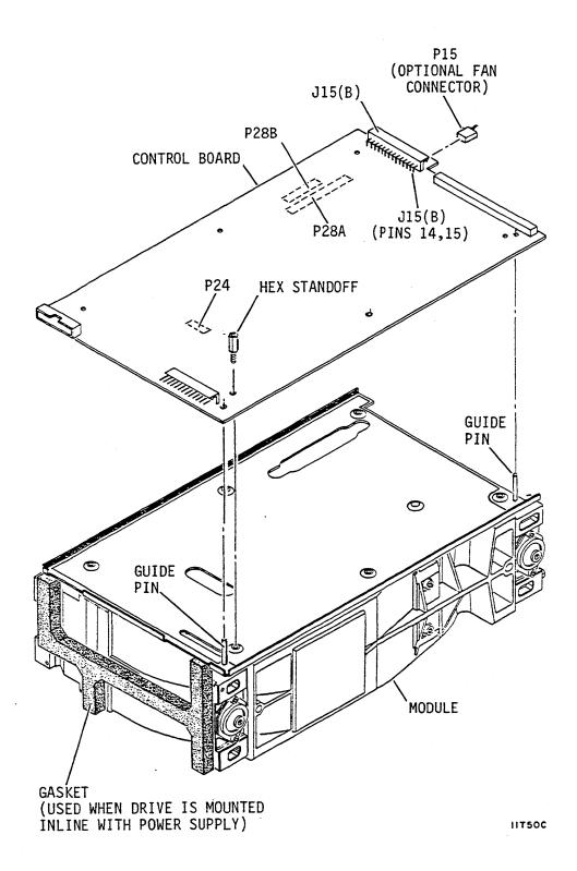
Figure 3-15. Control Board Replacement
