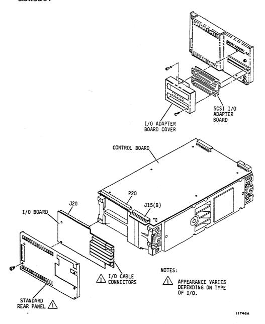
Figure 3-13. I/O Board Replacement (SMD and SCSI)
