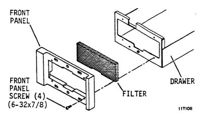
Figure 3-5. Front Panel Replacement For Drives Without Status/Control Panel or Operator Panel
