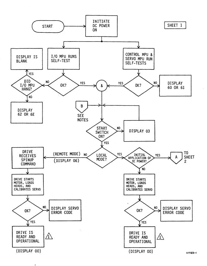
Figure 2-4. Power On Self-Test (Sheet 1 of 2)
