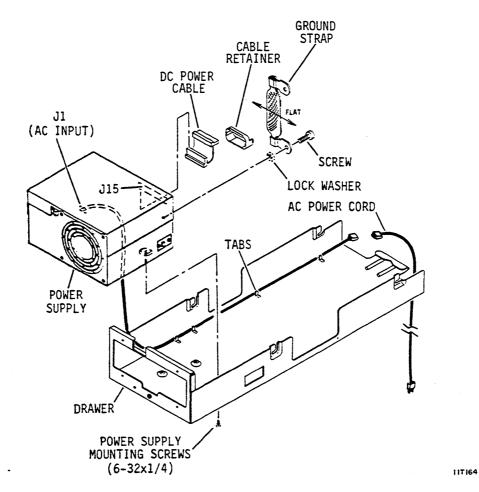
Figure 3-9. Power Supply Replacement
