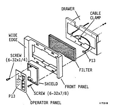
Figure 3-8. Operator Panel Replacement
