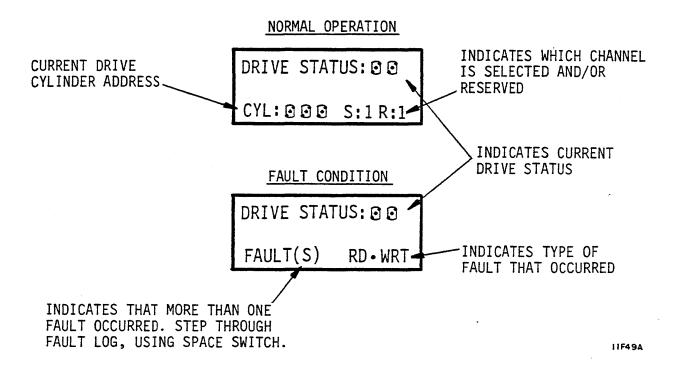
Figure 2-3. Example of LCD (Liquid Crystal Display)
