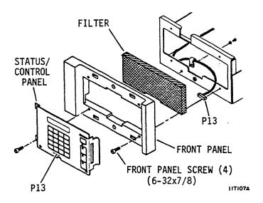
Figure 3-7. Status/Control Panel Replacement
