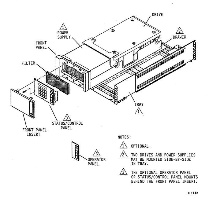
Figure 1-1. Component Locator (Sheet 2)
