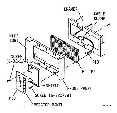
Figure 3-4. Front Panel Replacement For Drives With Operator Panel
