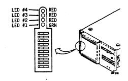
TABLE 2-12. I/O BOARD LEDS ON SCSI DRIVES
