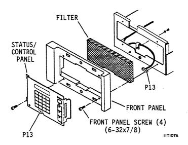
Figure 3-3. Front Panel Replacement For Drives With Status/Control Panel
