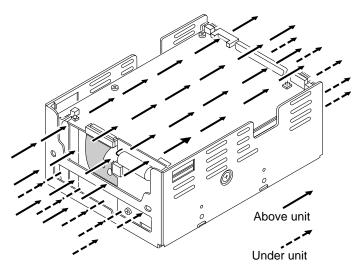
**Note.** Air flows in the direction shown (front to back) or in reverse direction (back to front)
