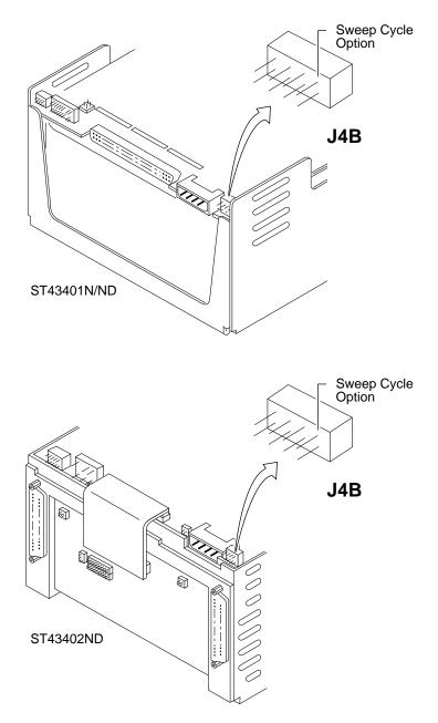
Figure 10. Control board jumpers
