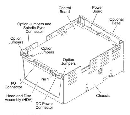
Figure 1. ST43401N/ND drive components
