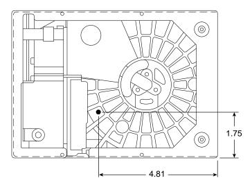
Figure 6. Temperature measurement location on the HDA (bottom)
