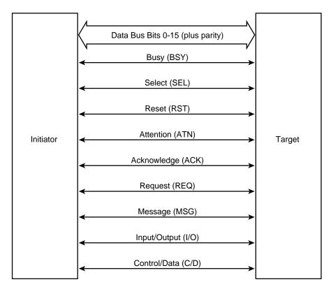
Figure 12. SCSI bus signal lines
