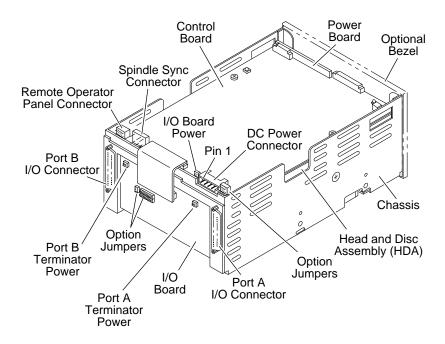
Figure 2. ST43402ND drive components
