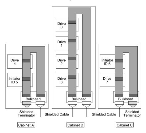
Figure 9. Cabling with three cabinets
