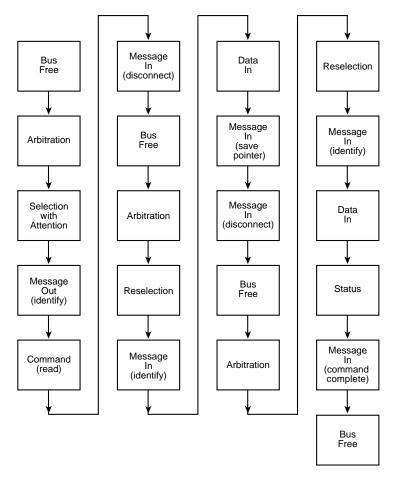
Figure 13. Sequence of a typical command
