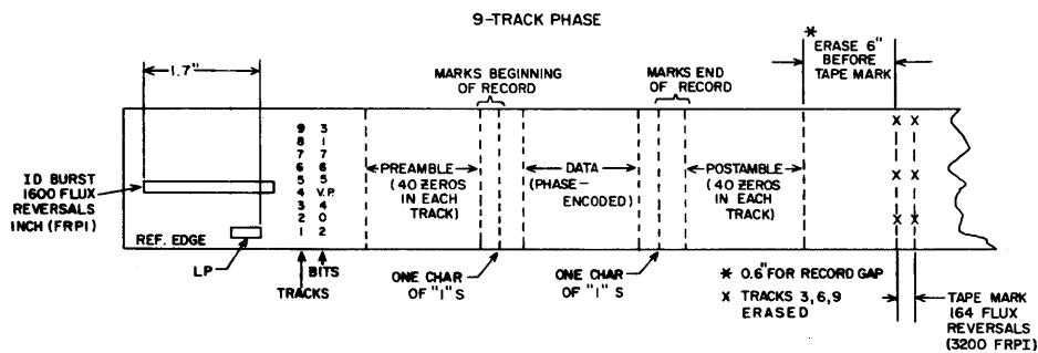
Figure 1-5. Phase Encoded Format
