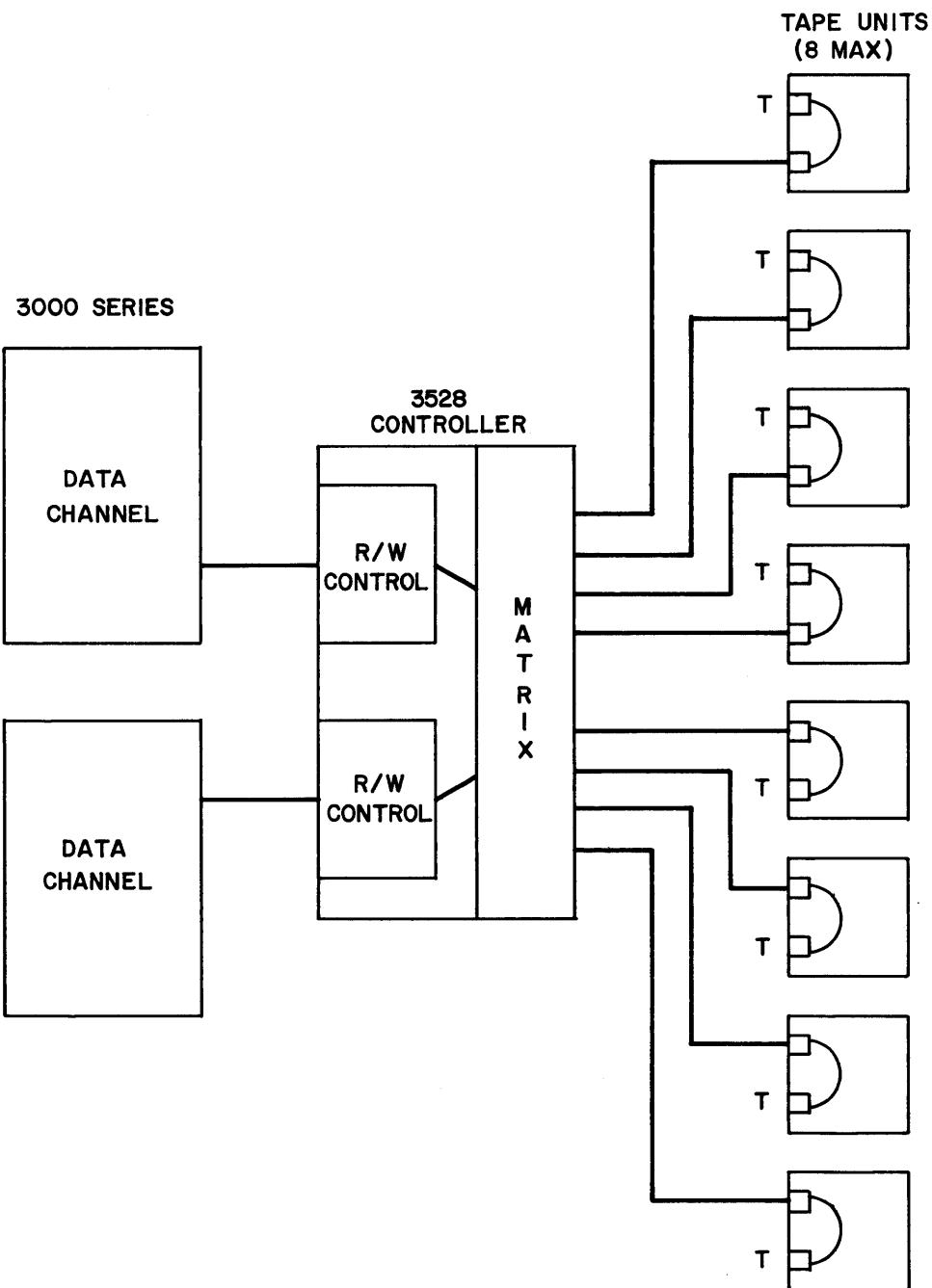
Figure 1-2. Typical Dual Channel Configuration
