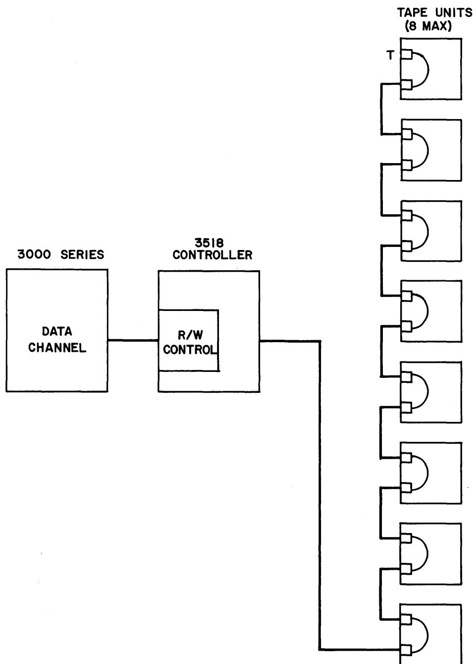
Figure 1-1. Typical Single Channel Configuration
