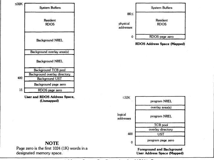
Figure 1-1. Address Space Configuration for NOVA Computers
