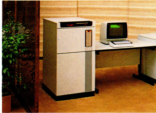
Burroughs B920: This compact cabinet can contain from five to eight powerful processors to handle your information management needs. Your particular configuration may include an operator display terminal, which shows instructions, messages and data input in bright, easy to read characters. The systems shown above and to the right are configured with Burroughs Super Mini Disk drives inbuilt.
