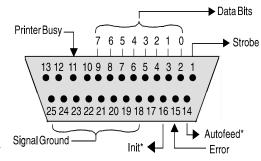
\* These signals are held high, in an inactive state.
