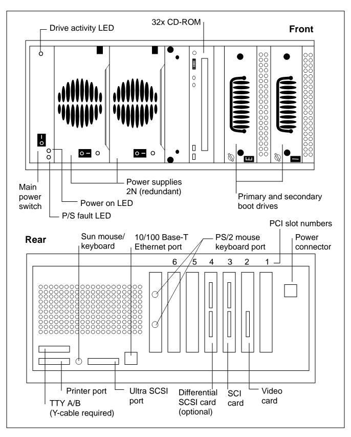
Host module (front, rear; bezels removed)
