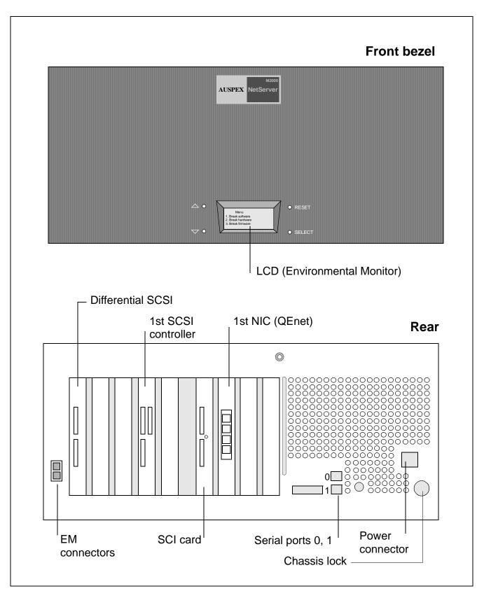
E-Box module (front, rear; rear bezel removed)
