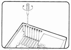
Figure 14 Removal of System Expansion Slot Cover
