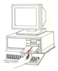
NOTE: It is extremely important that you never remove a diskette while it is being read from or written to by the computer. Doing so can destroy the information on the diskette. You can tell if the computer is accessing a diskette by looking at the indicator light on the drive that the diskette is in.
