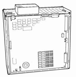
Figure 2 Positioning of System Module.
