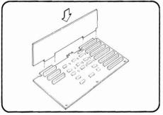
Figure 15 Insertion of Memory Expansion Board
