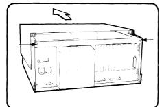
INSTALLING A MEMORY EXPANSION BOARD
