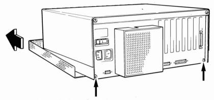
Figure 1 Removal of Basic Module's Cover.
