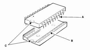
Figure 5 Chip Insertion.
