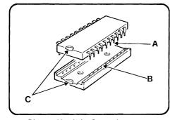
Figure 10 Chip Insertion
