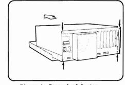
Figure 6 Removal of System Module Covers
