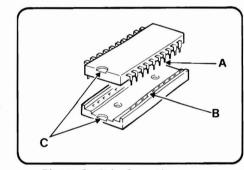
Figure 5 Chip Insertion
