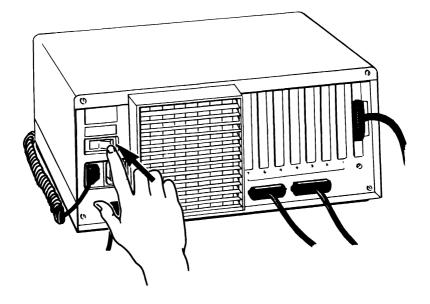
For about five seconds after your computer is turned on, it runs a self check to make sure that it is working properly.
