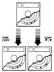
DISKCOPY transfers the files to the new diskette just as broken up as they are on the original diskette. COPY, on the other hand, copies each file individually. It locates all of the separate parts of each file and then writes them as one continuous file. Thus your disk is reorganized for you automatically when you use COPY to back up your diskettes and is therefore the recommended procedure.
