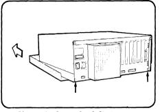
Figure 1 Removal of System Module's Cover
