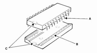
Figure 10 Chip Insertion.
