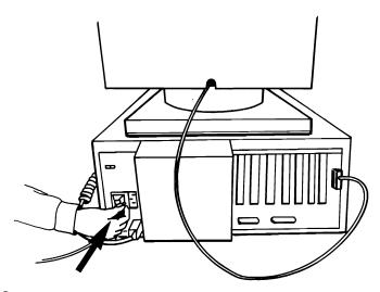
**3** Connect the female end of the power cable to the INPUT AC socket on the rear of the main unit.
