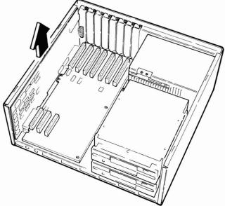
Figure 7 Removal of Memory Expansion Board.
