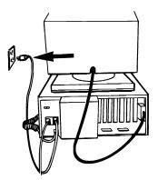
4 Plug the male end of the power cable into a 115 vac 60 Hz grounded wall outlet.
