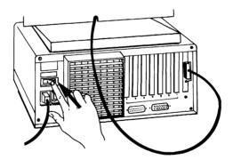
2 Turn on the computer. The on-off switch is located above the power cable socket on the rear of the main unit.
