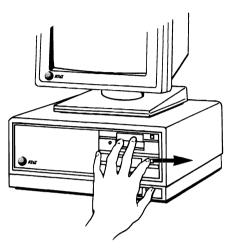
4 Hold the diskette by the side that has the label. Gently insert the diskette with its label facing up into disk drive A. Drive A is the lower one.
